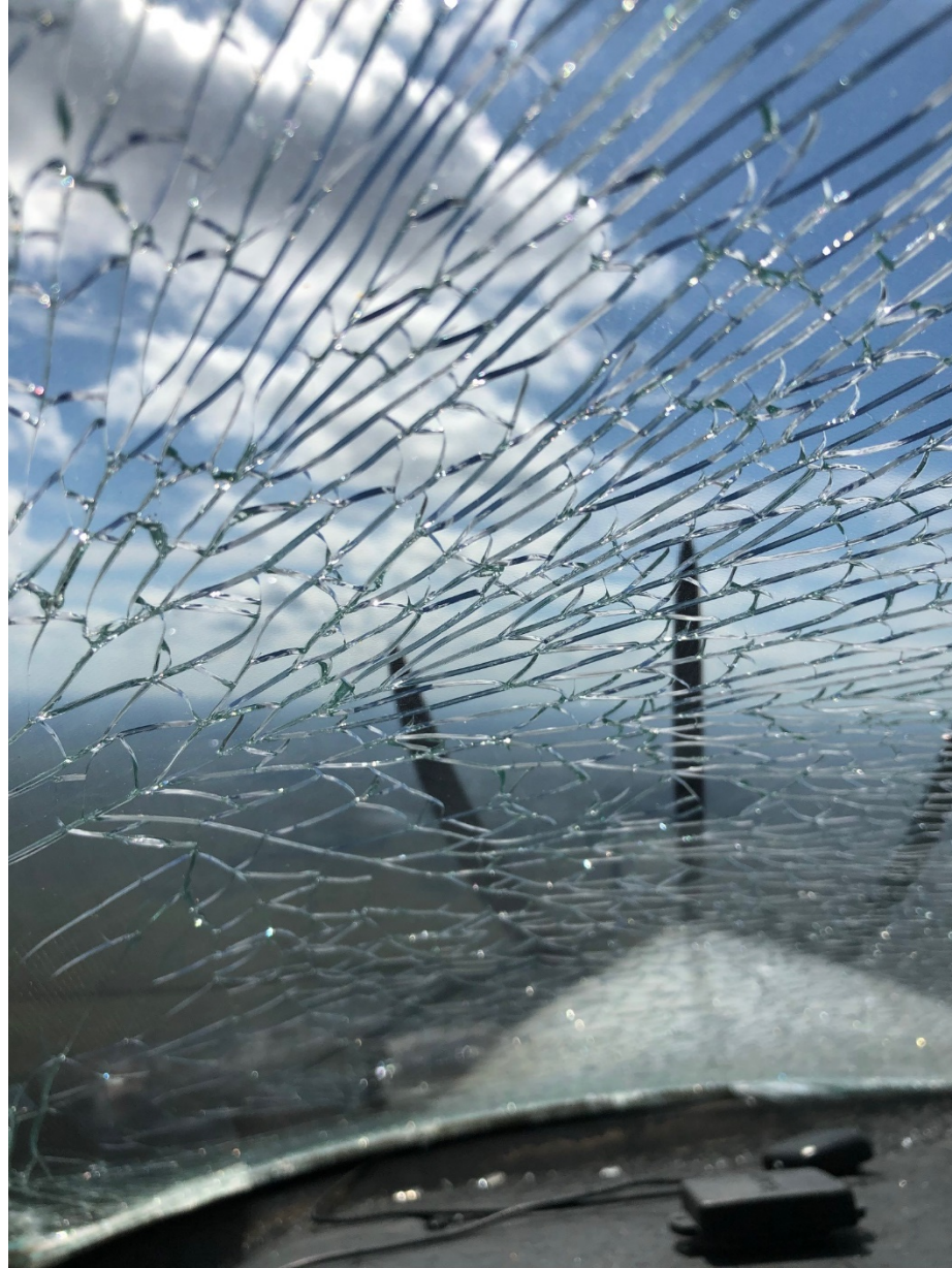
Photo 1 – Shattered Windshield, inside view
