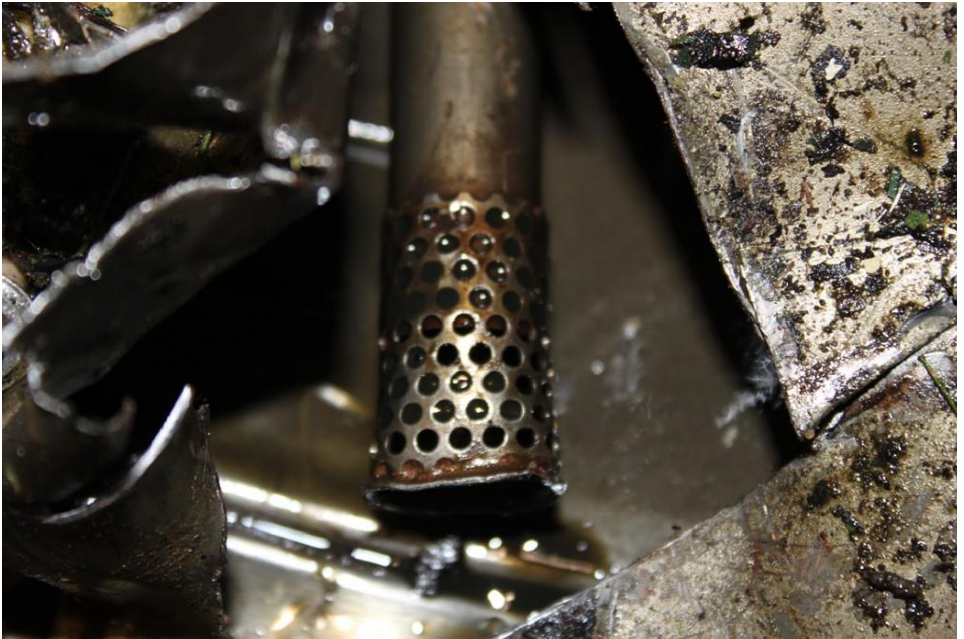
Photo 15 - NTSB Digital Photograph. View of the Oil Pickup Screen
