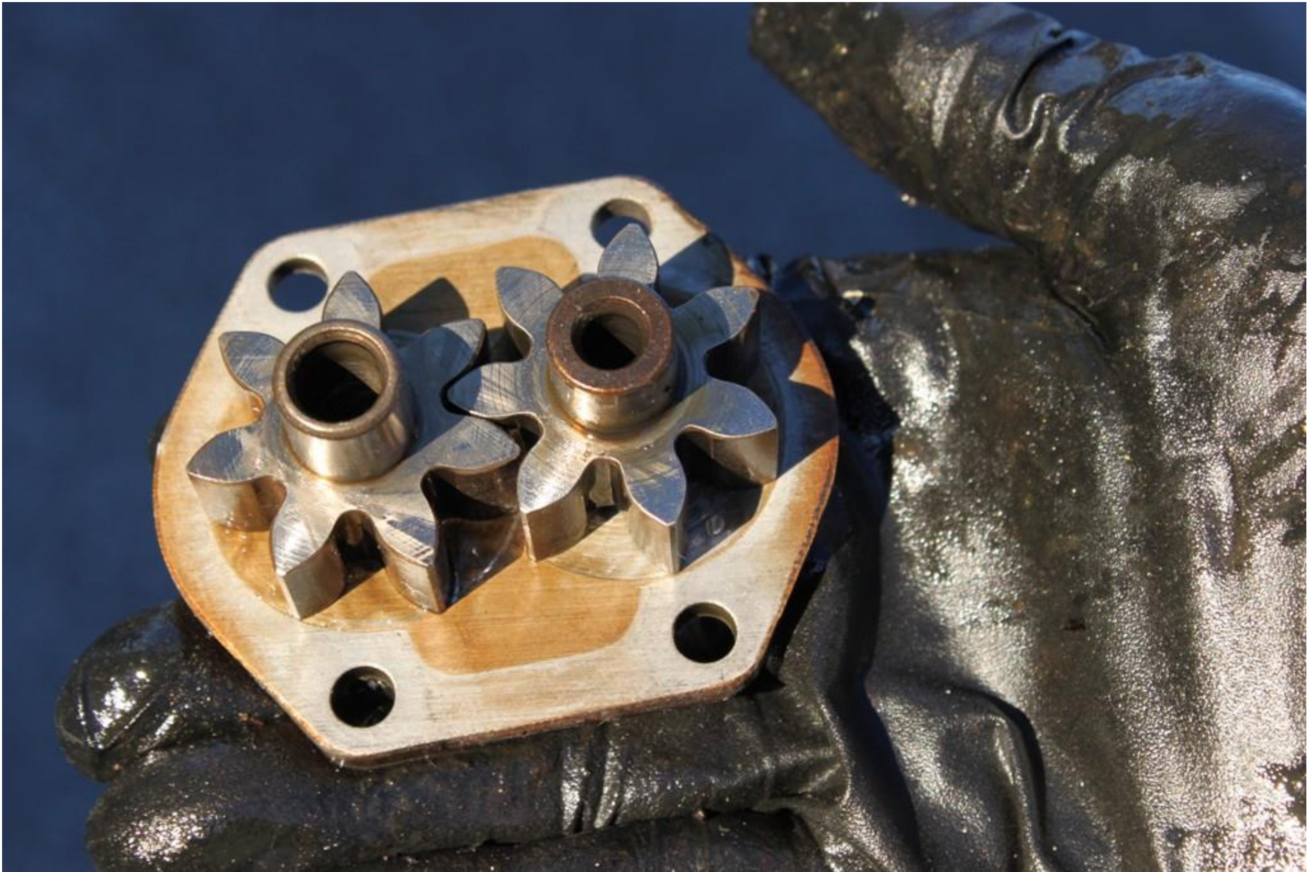
Photo 20 - NTSB Digital Photograph. View of the Oil Pump Gears
