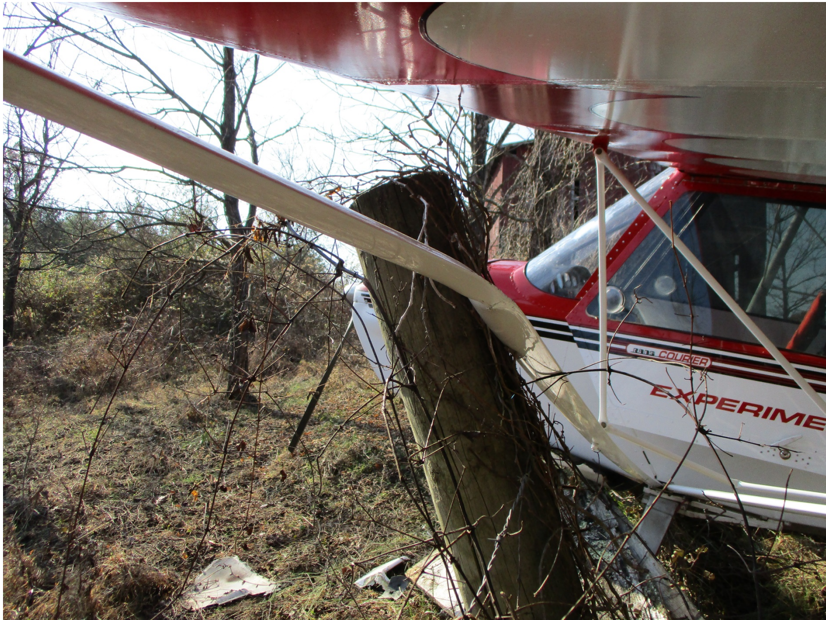
Photo 2 – View of Left Wing Damage (Courtesy of FAA)
