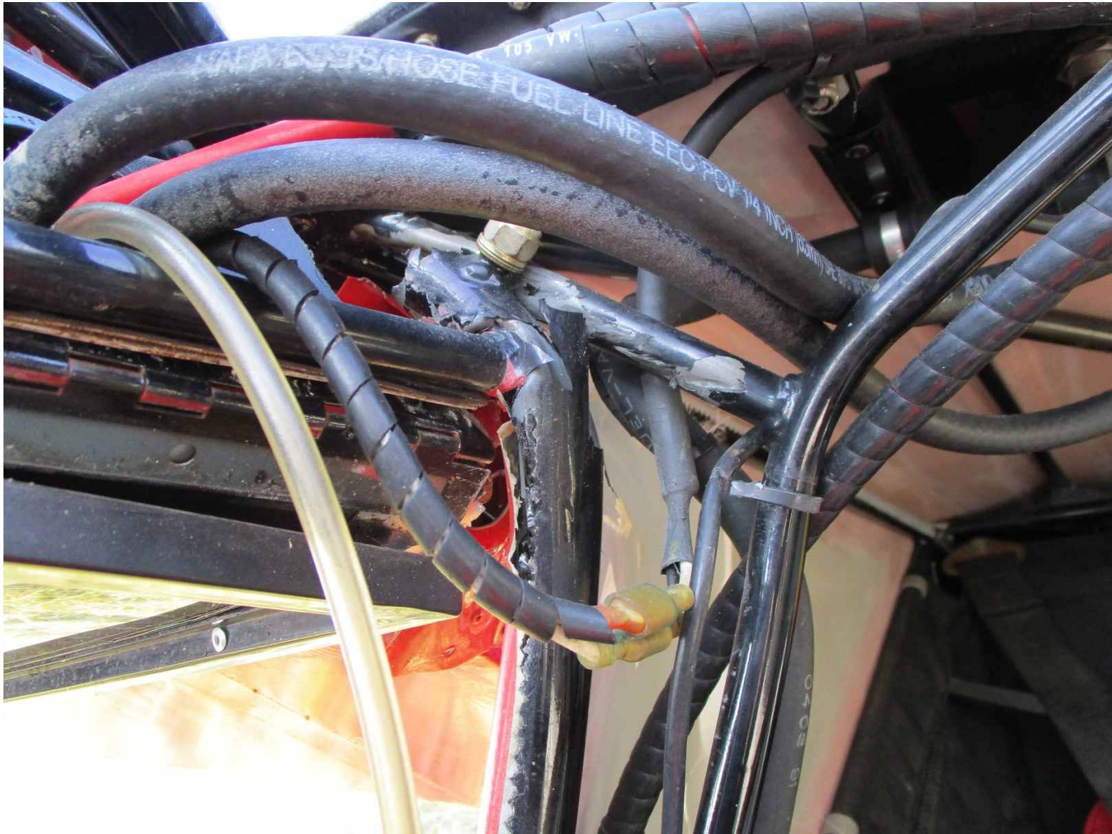
Photo 3 – View of engine mount damage (Courtesy of FAA)
