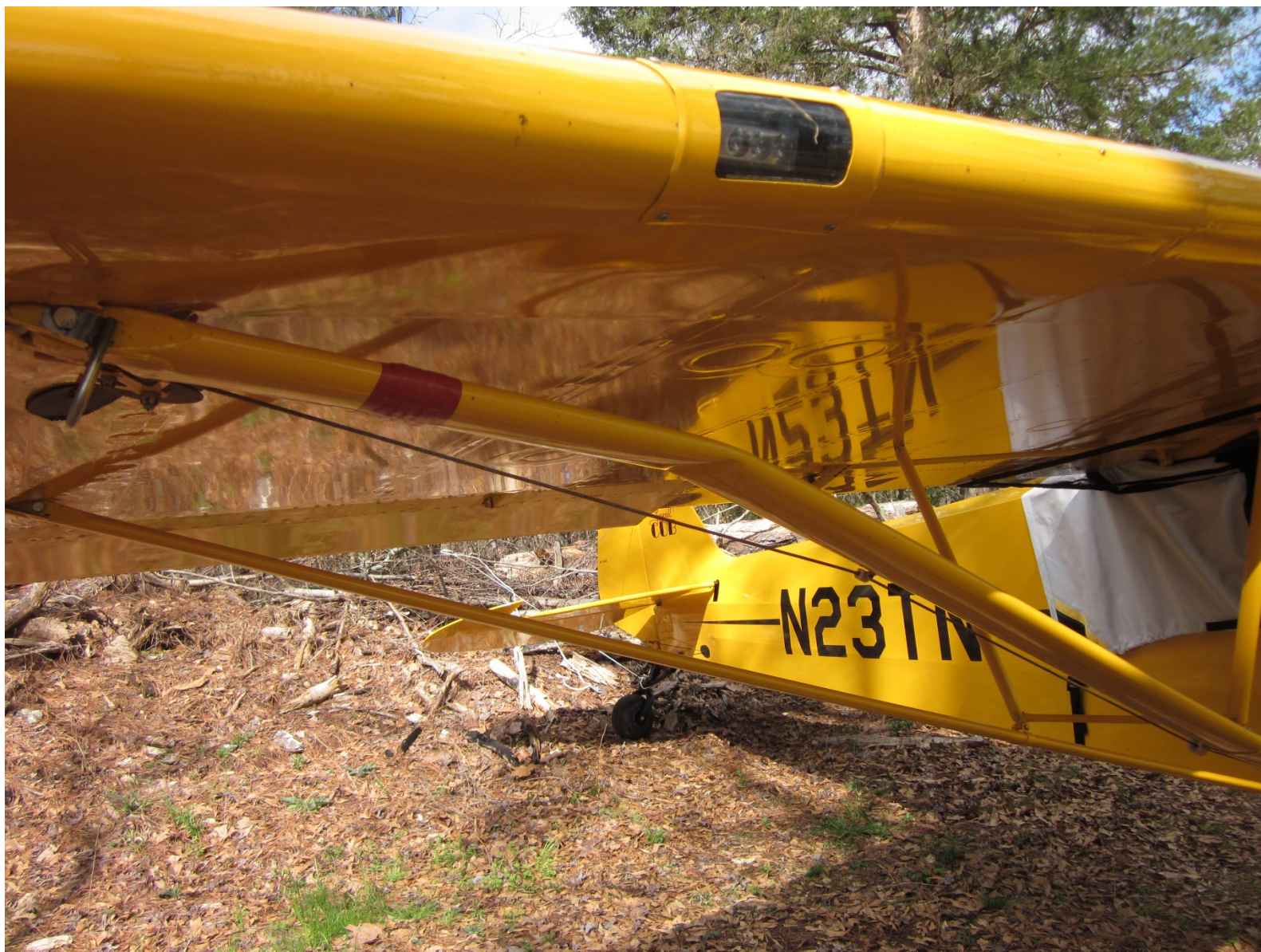
Photo 3 – View of Right Wing Strut Damage (Courtesy of FAA)
