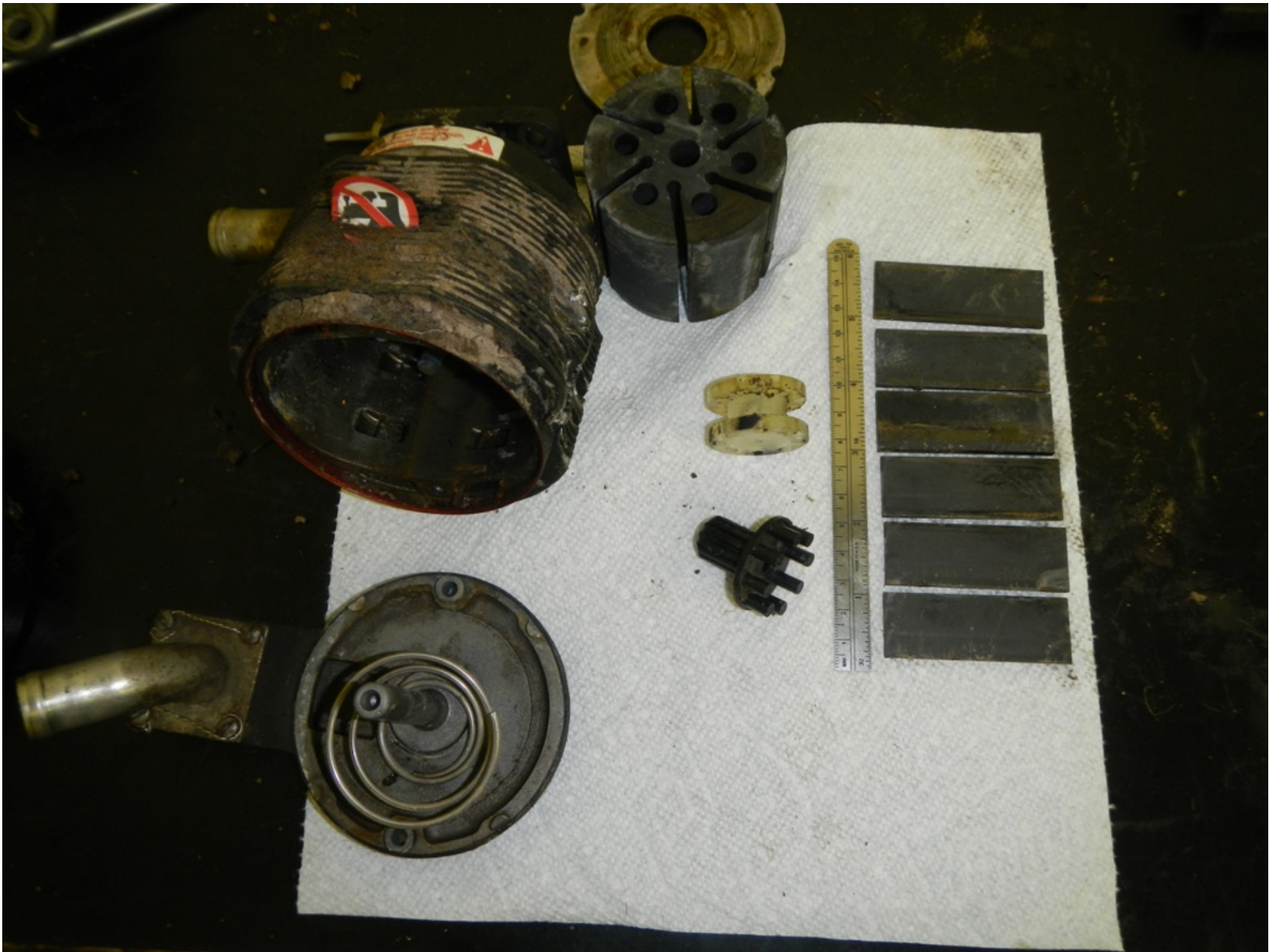
Photo 11 - Continental Aerospace Technologies Digital Photograph. View of the Right Engine-Driven Vacuum Pump Following Disassembly.
