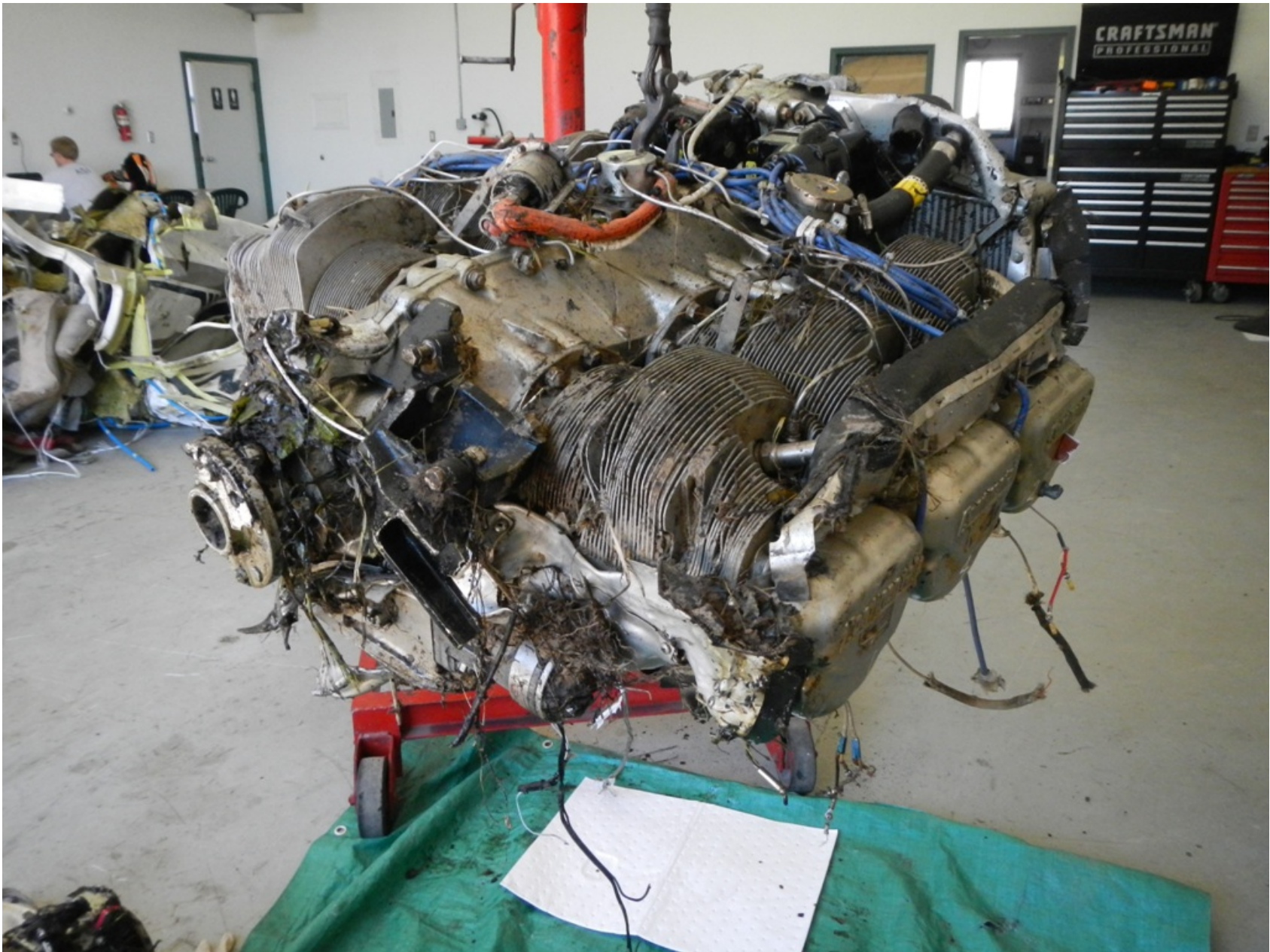
Photo 9 – Continental Aerospace Technologies Digital Photograph. View of the Left Engine Following Recovery.
