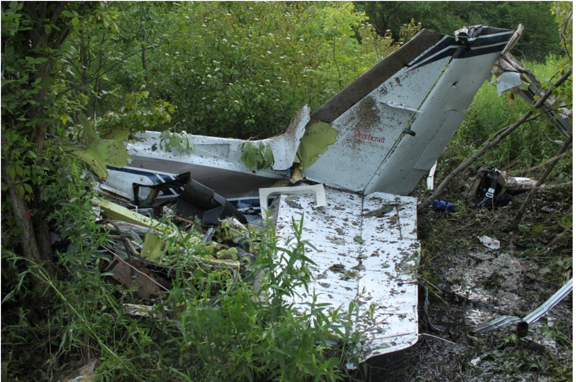
Photo 7 - NTSB Digital Photograph. Left Side View of Aft Empennage at the Accident Site.
