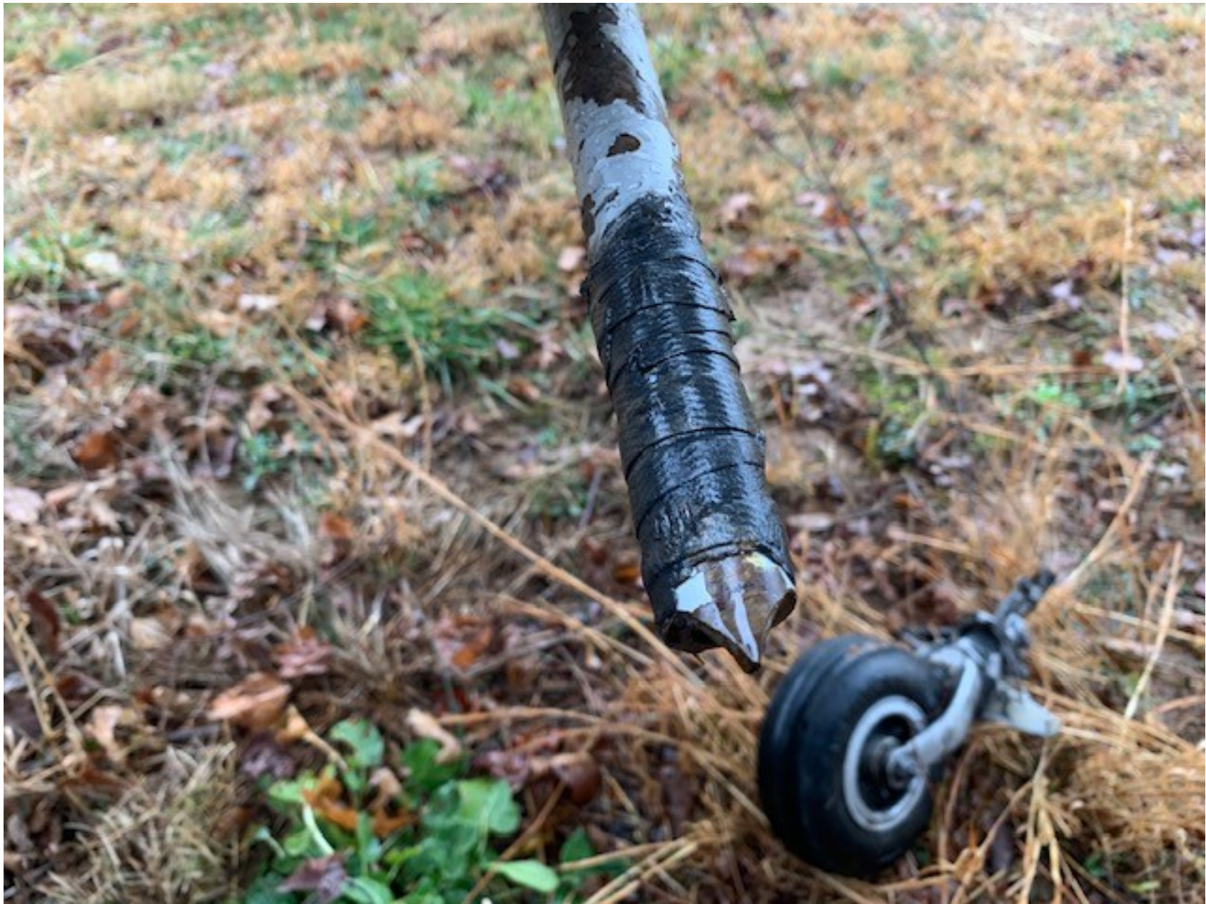
Photo 4 – Closer View of Broken Tailwheel Attach Tube (Courtesy of Salvage Company)
