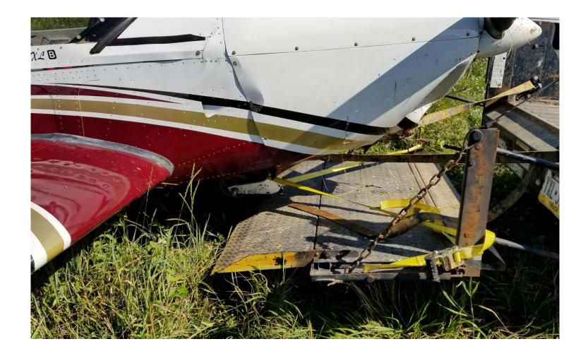
Photo 3 – Cowling Damage (Photo Courtesy of Pilot)
