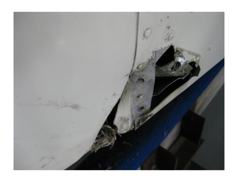
Photo 3 – Close up view of fuselage rib damage (Courtesy of FAA)
