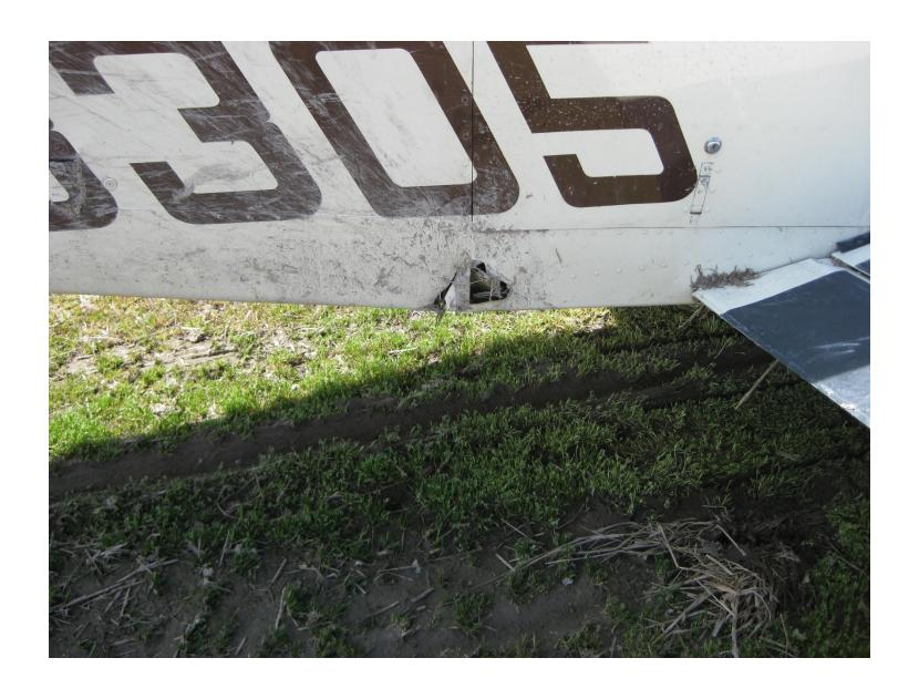
**Photo 2 – View of Fuselage Damage (Courtesy of FAA)**
