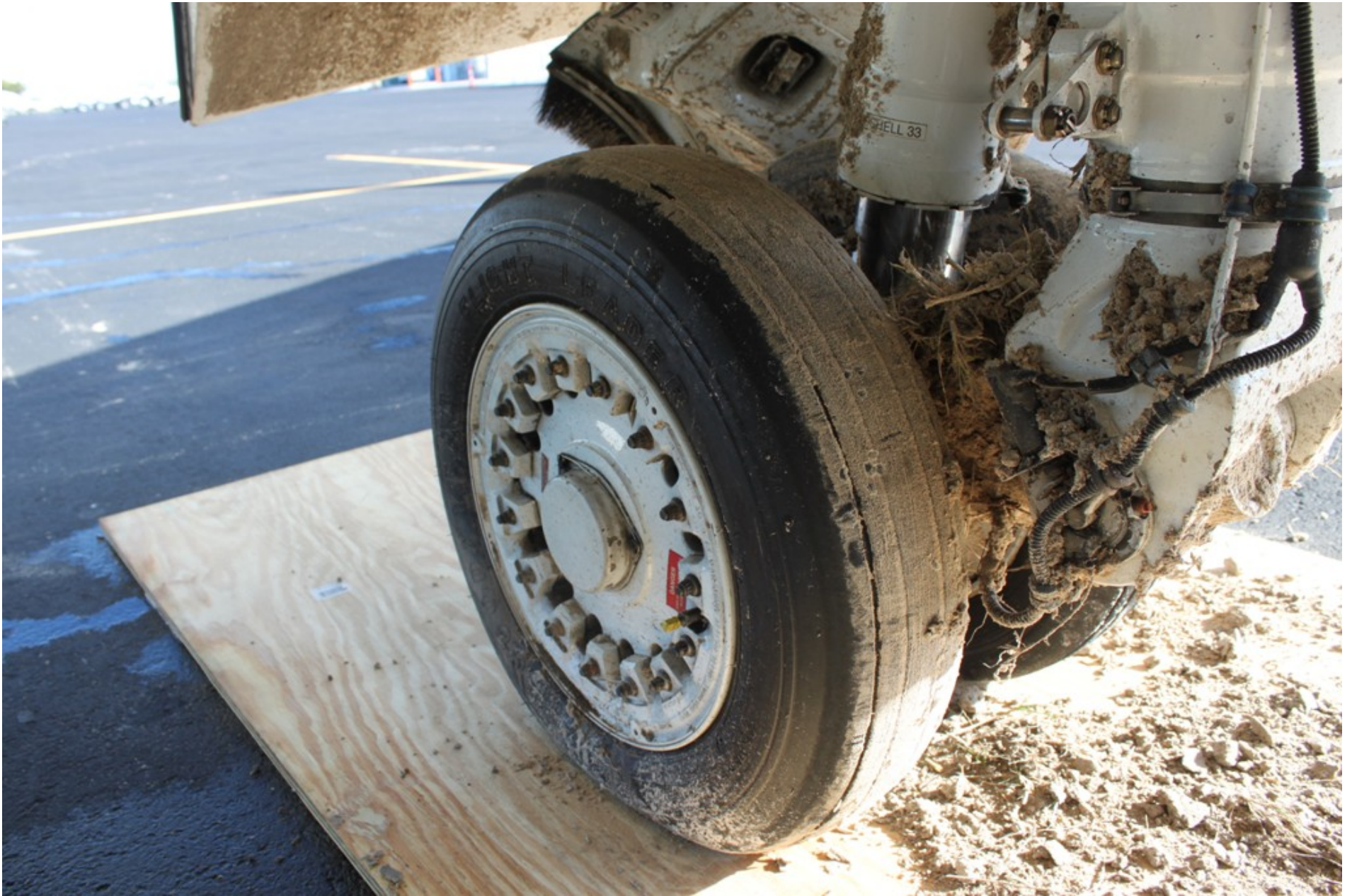
Photo 3 - NTSB Photograph. View Depicting the Inflated No. 2 Tire
