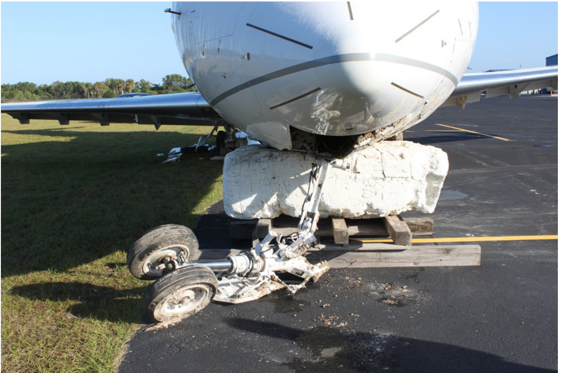
Photo 2 - NTSB Photograph. View Looking aft Depicting the Separated Nose Landing Gear
