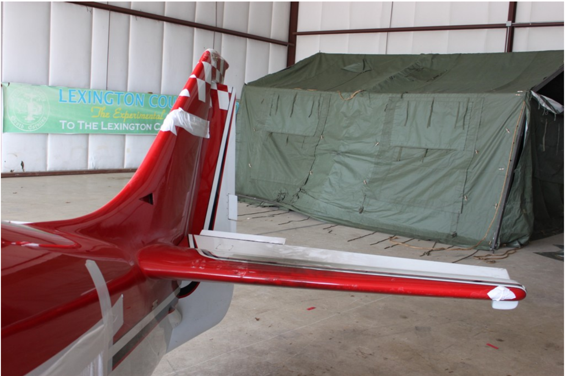
Photo 6 - NTSB Digital Photograph. Left Side of Aft Empennage with Left Horizontal Stabilizer, Elevator, Vertical Stabilizer and Rudder.
