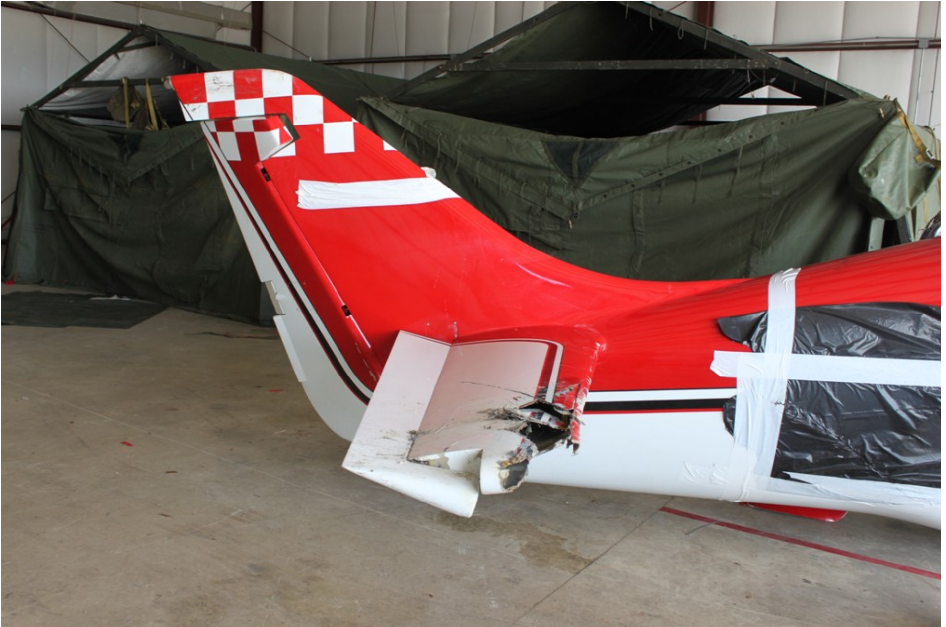
Photo 7 - NTSB Digital Photograph. Right Side of Aft Empennage with Damaged Right Horizontal Stabilizer, Elevator, Vertical Stabilizer and Rudder.
