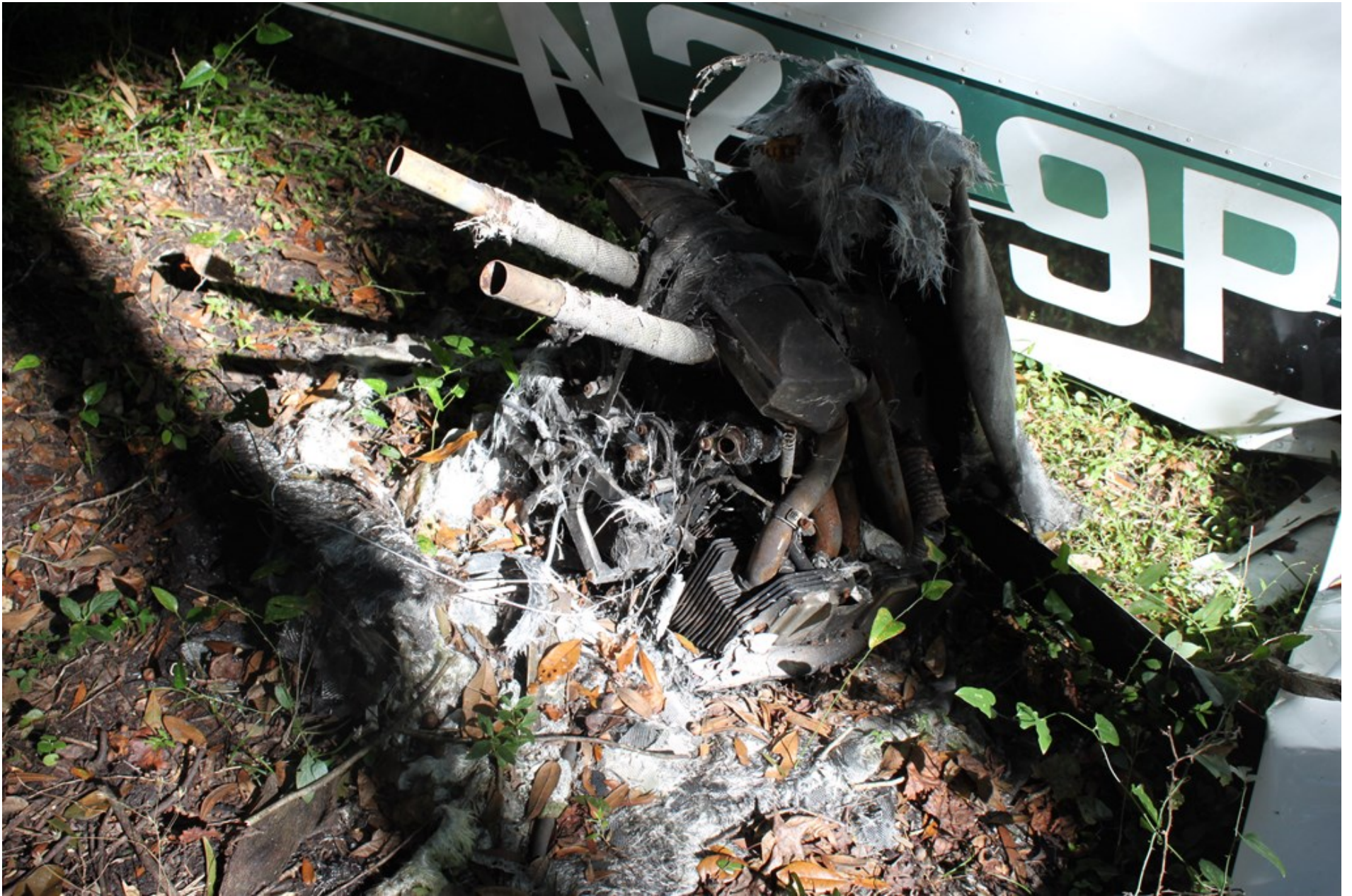
Photo 6 – NTSB Digital Photograph. View of the Separated Engine Assembly.
