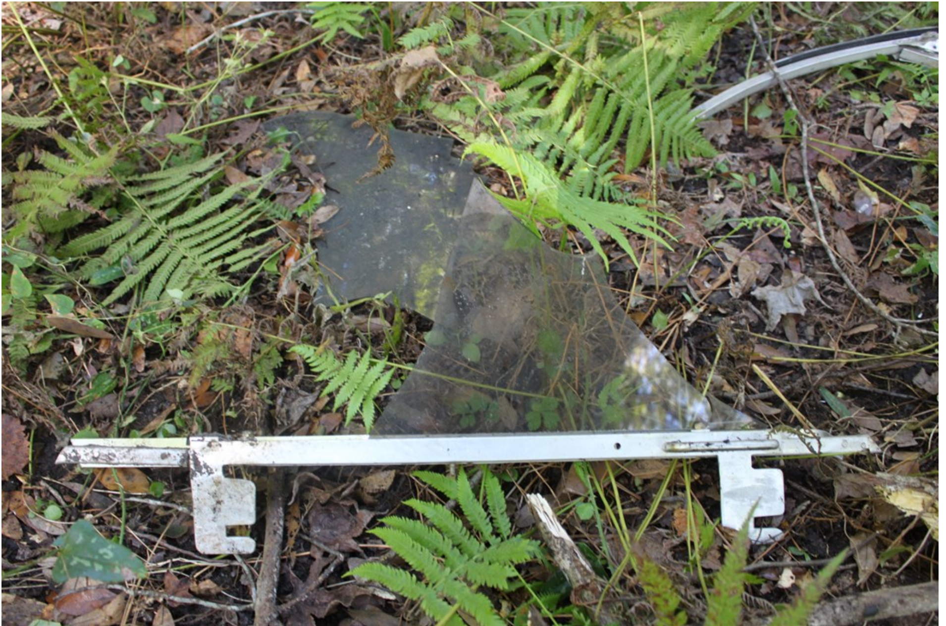
Photo 12 – NTSB Digital Photograph. View depicting the locking portion of the canopy. Note the undamaged latches for taxi (lower) and takeoff (upper) positions
