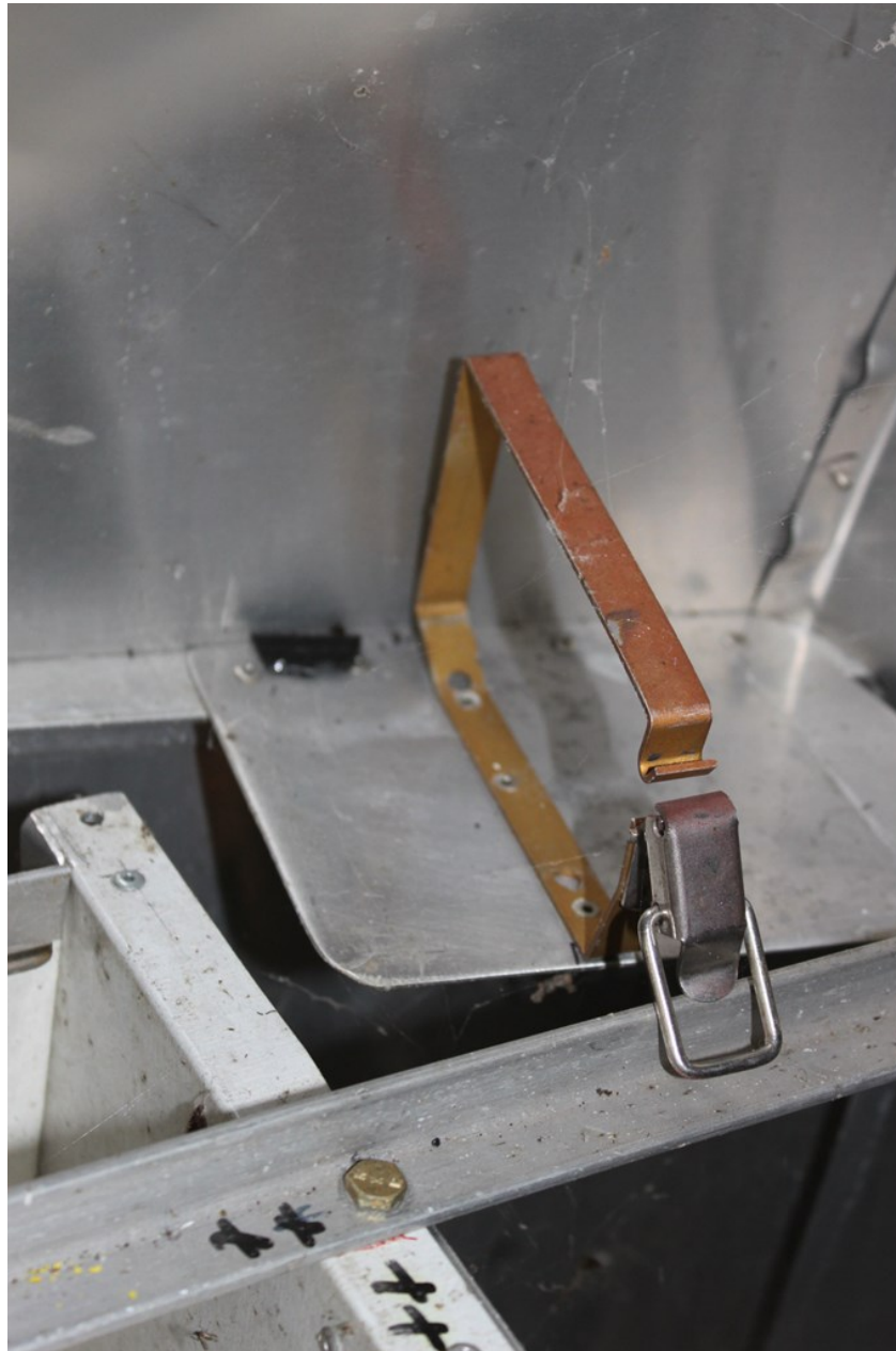
Photo 14 – NTSB Digital Photograph. View Depicting the ELT Bracket and Lower Mount Tray
