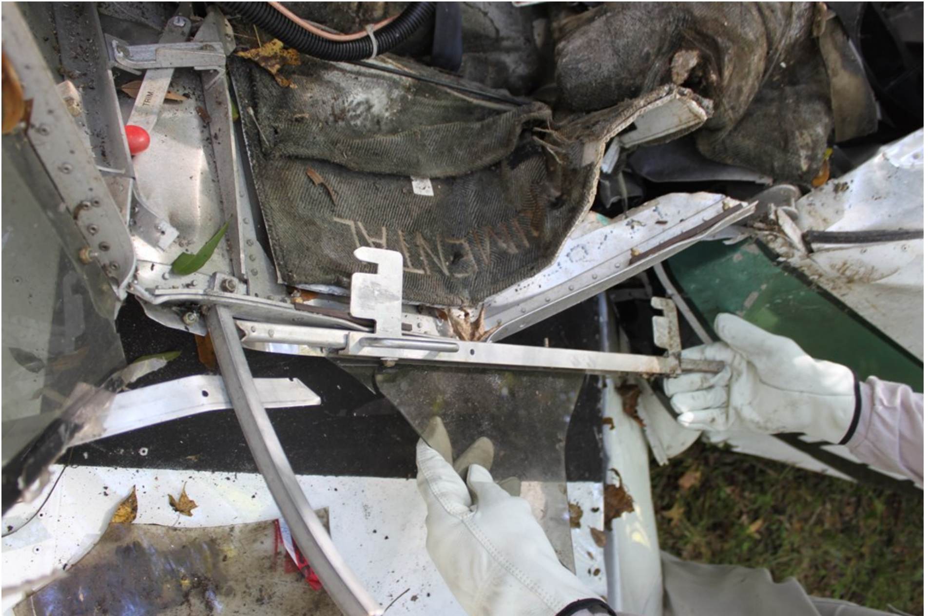
Photo 13 – NTSB Digital Photograph. View Depicting the Damage to the Longeron adjacent to the Locking Portion of the Canopy Frame, and the Locking Portion of the Canopy Frame
