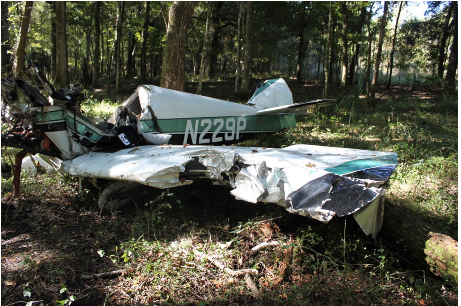
Photo 8 – NTSB Digital Photograph. View of the Left Wing. Note the Leading Edge Tree Contact Damage
