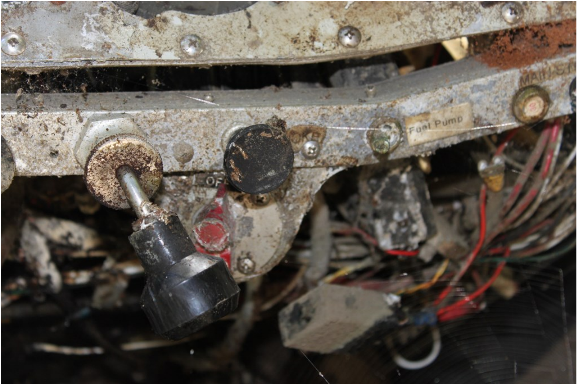
Photo 11 – NTSB Digital Photograph. View of the Fuel Shutoff Valve Position.
