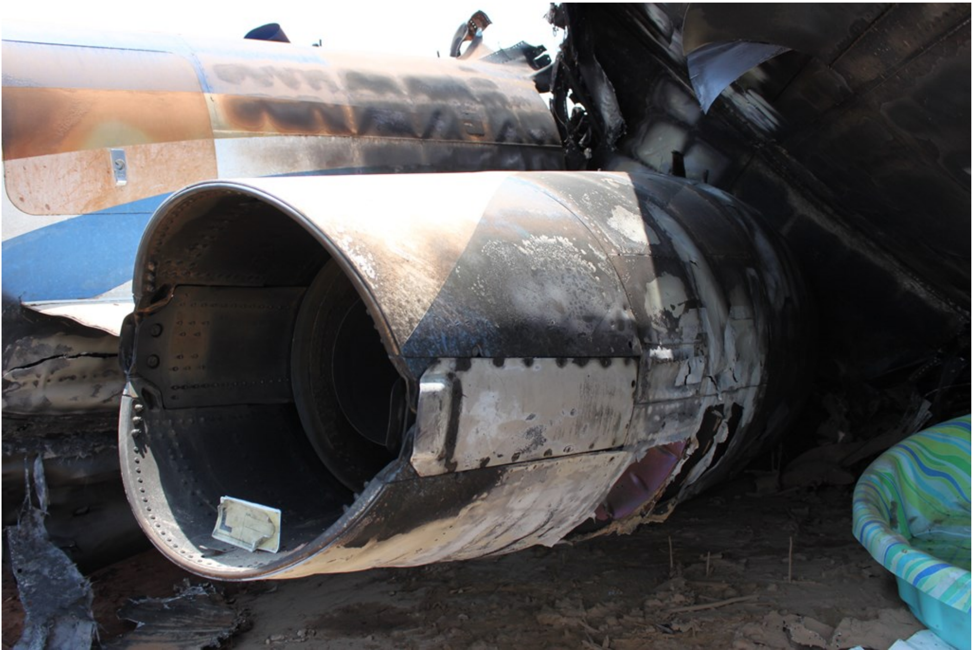
Photo 8 - NTSB Digital Photograph. View depicting the left engine upper and lower thrust reverser clamshell doors.
