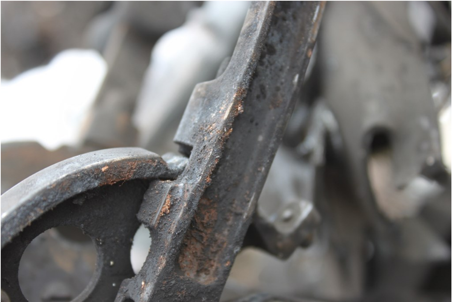
Photo 11 - NTSB Digital Photograph. Close-up View of the Right Engine Thrust Reverser Piggy Back Lever and Adjacent Portion of Throttle Quadrant. Note the impact signature aft of the deploy detent.
