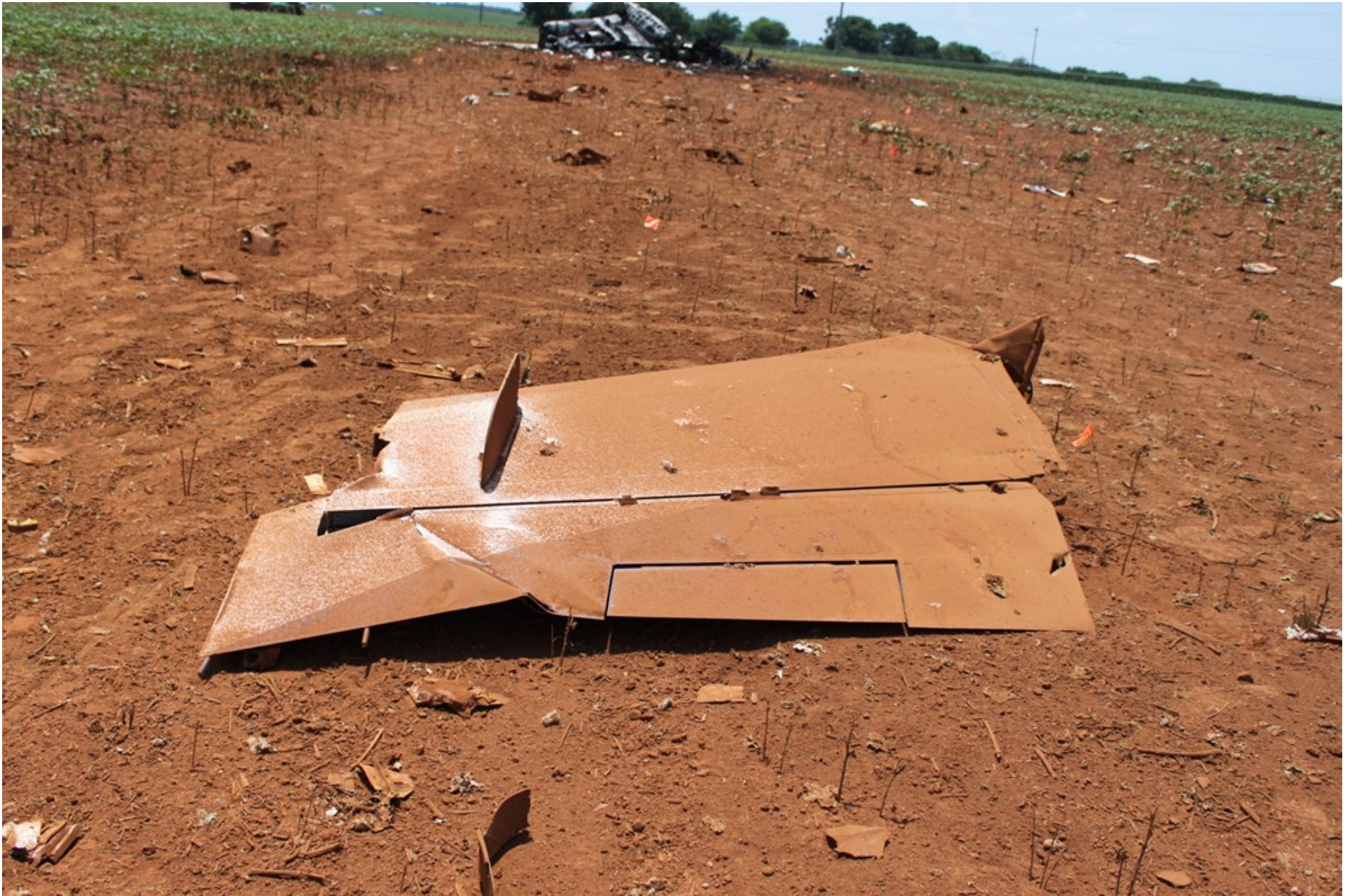
Photo 4 - NTSB Digital Photograph. View depicting the separated vertical stabilizer, rudder, and attached rudder trim tab, with wreckage in the background.
