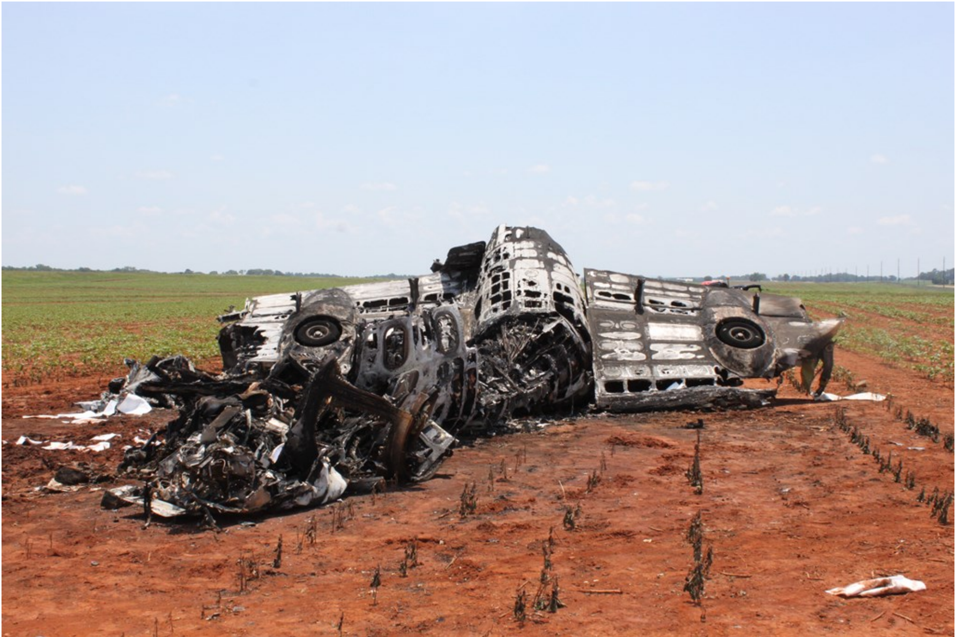
Photo 6 - NTSB Digital Photograph. Another view depicting the resting position of the inverted wing and fuselage section of the wreckage.
