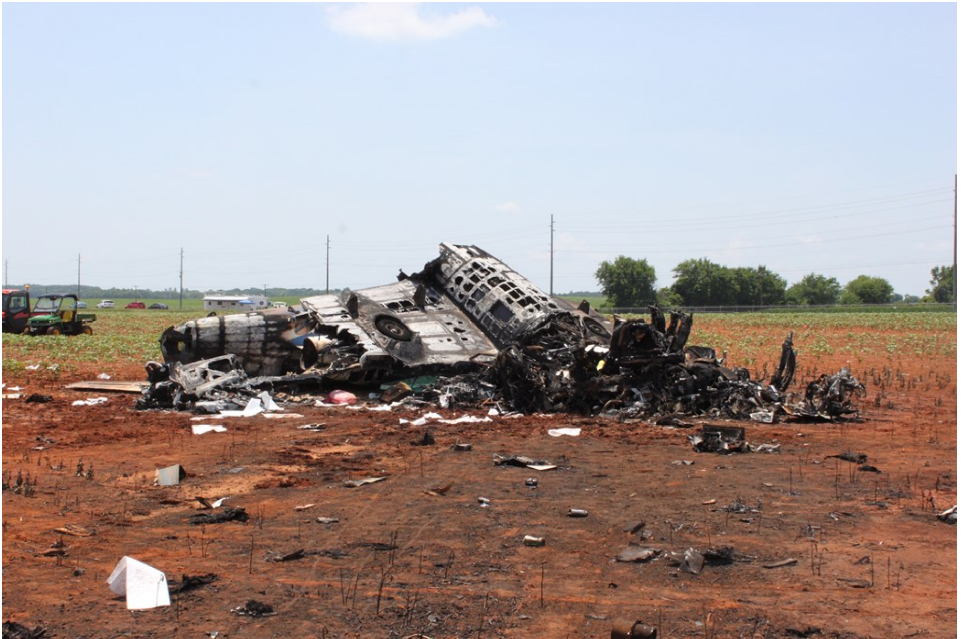
Photo 5 - NTSB Digital Photograph. View depicting the resting position of the inverted wing and fuselage section of the main wreckage.
