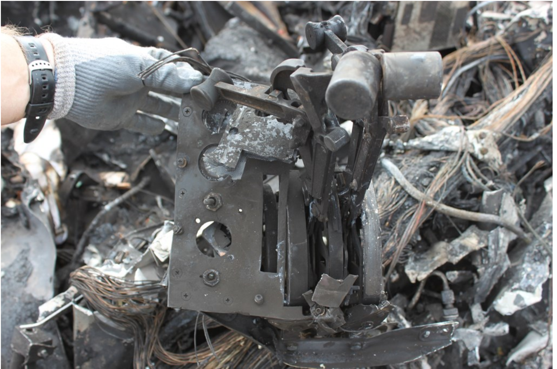
Photo 9 - NTSB Digital Photograph. View of the throttle quadrant.
