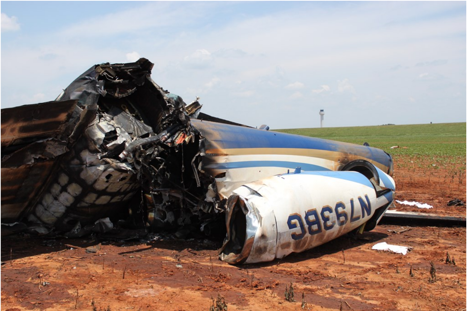
Photo 7 - NTSB Digital Photograph. View depicting the inverted wing and fuselage. Note the attached right engine and partially deployed upper and lower right thrust reverser clamshell doors.
