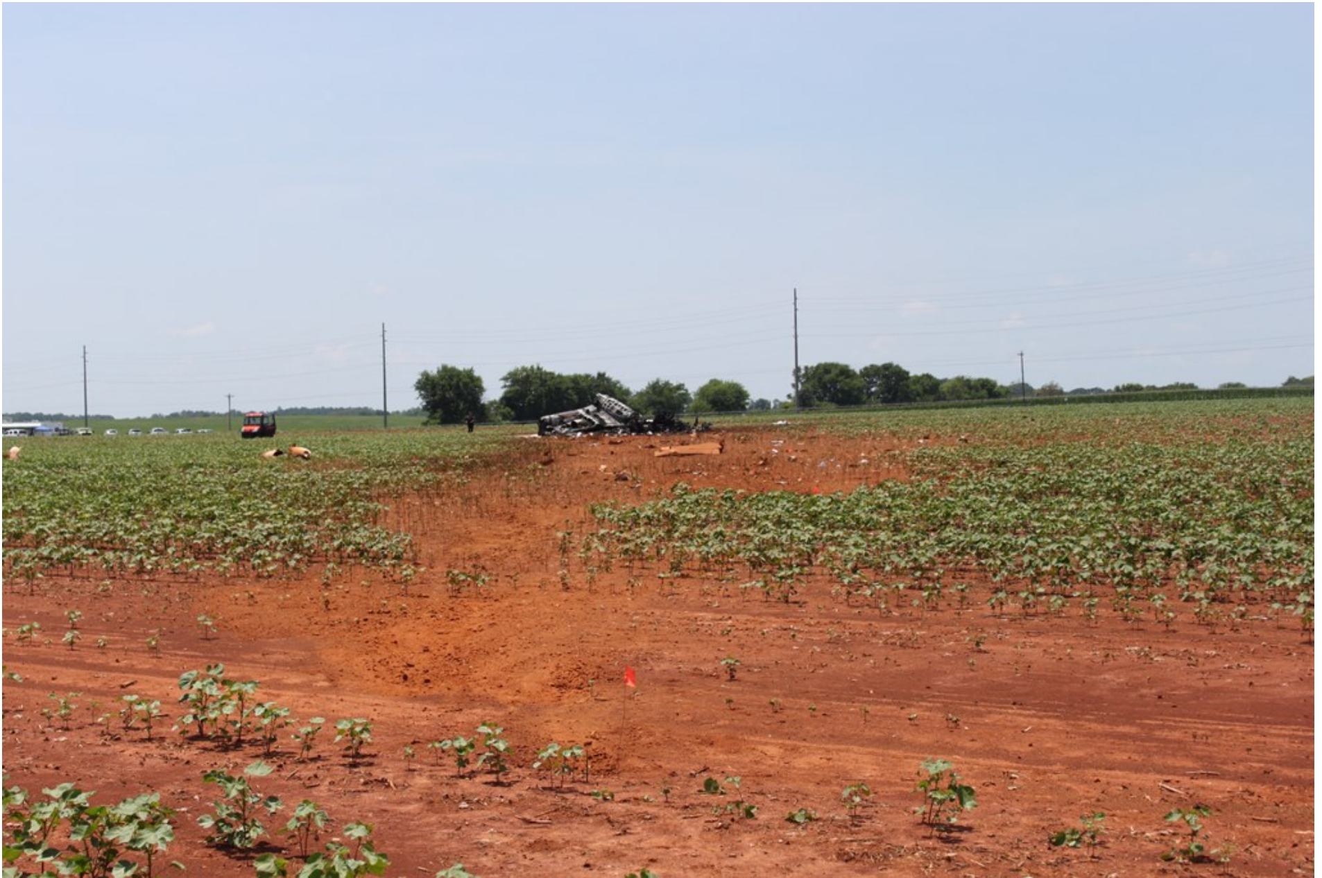
Photo 2 - NTSB Digital Photograph. View depicting the first impact crater and the energy path of the airplane with the wreckage in the background.
