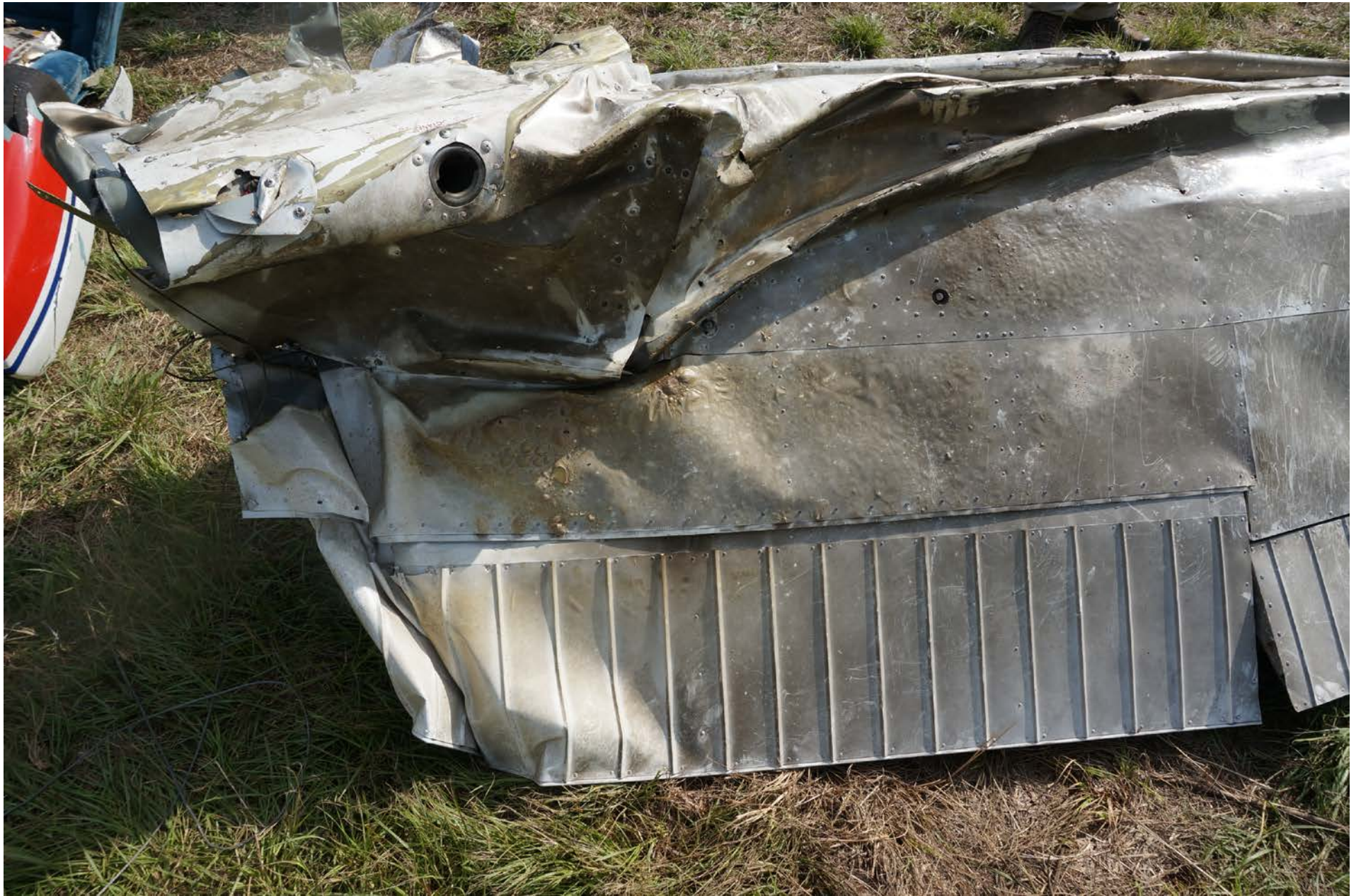
Photo 7 – Paint Scorching on Upper Side of Right Wing
