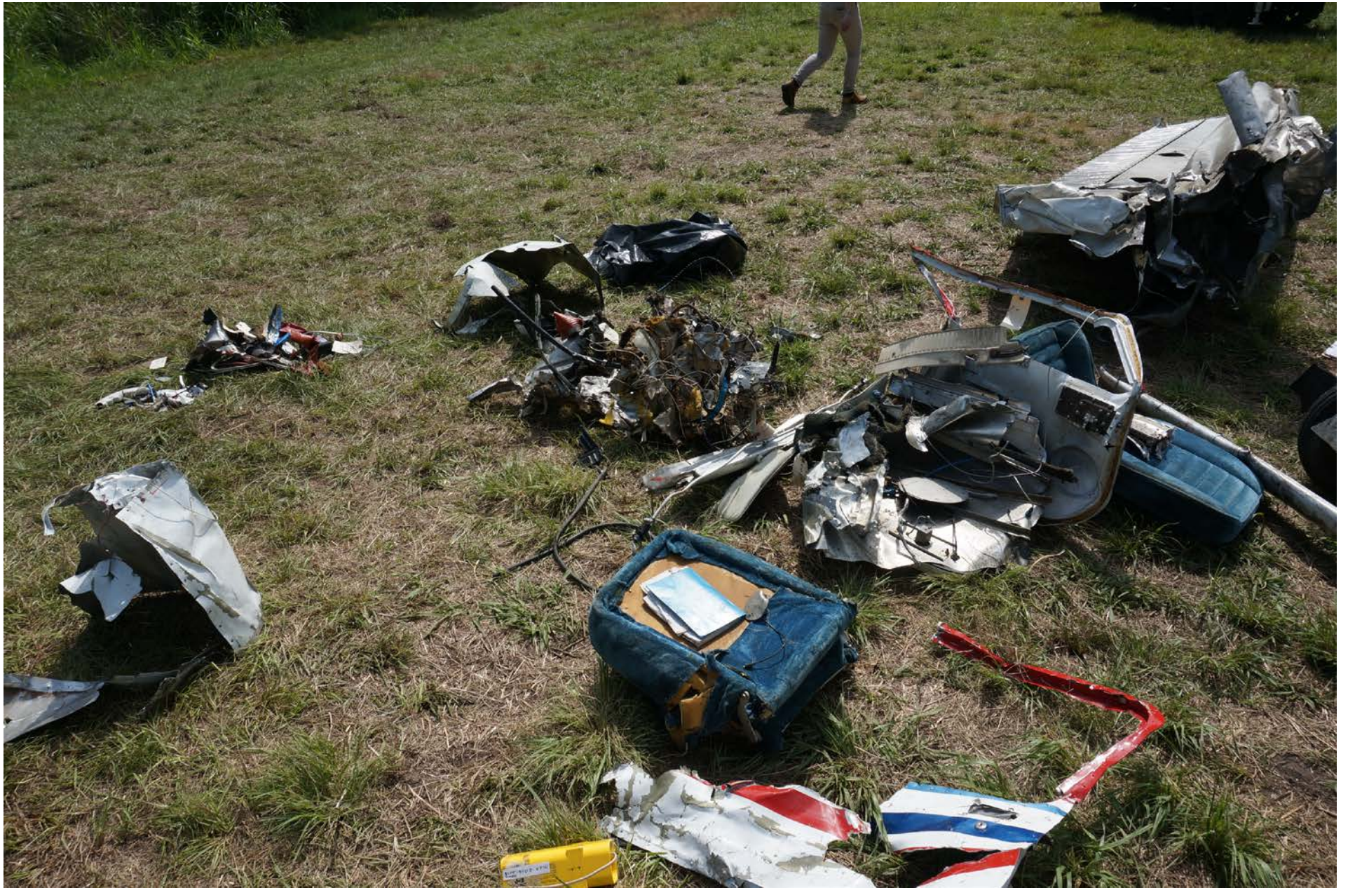
Photo 8 – Recovered Portions of Cessna Cabin
