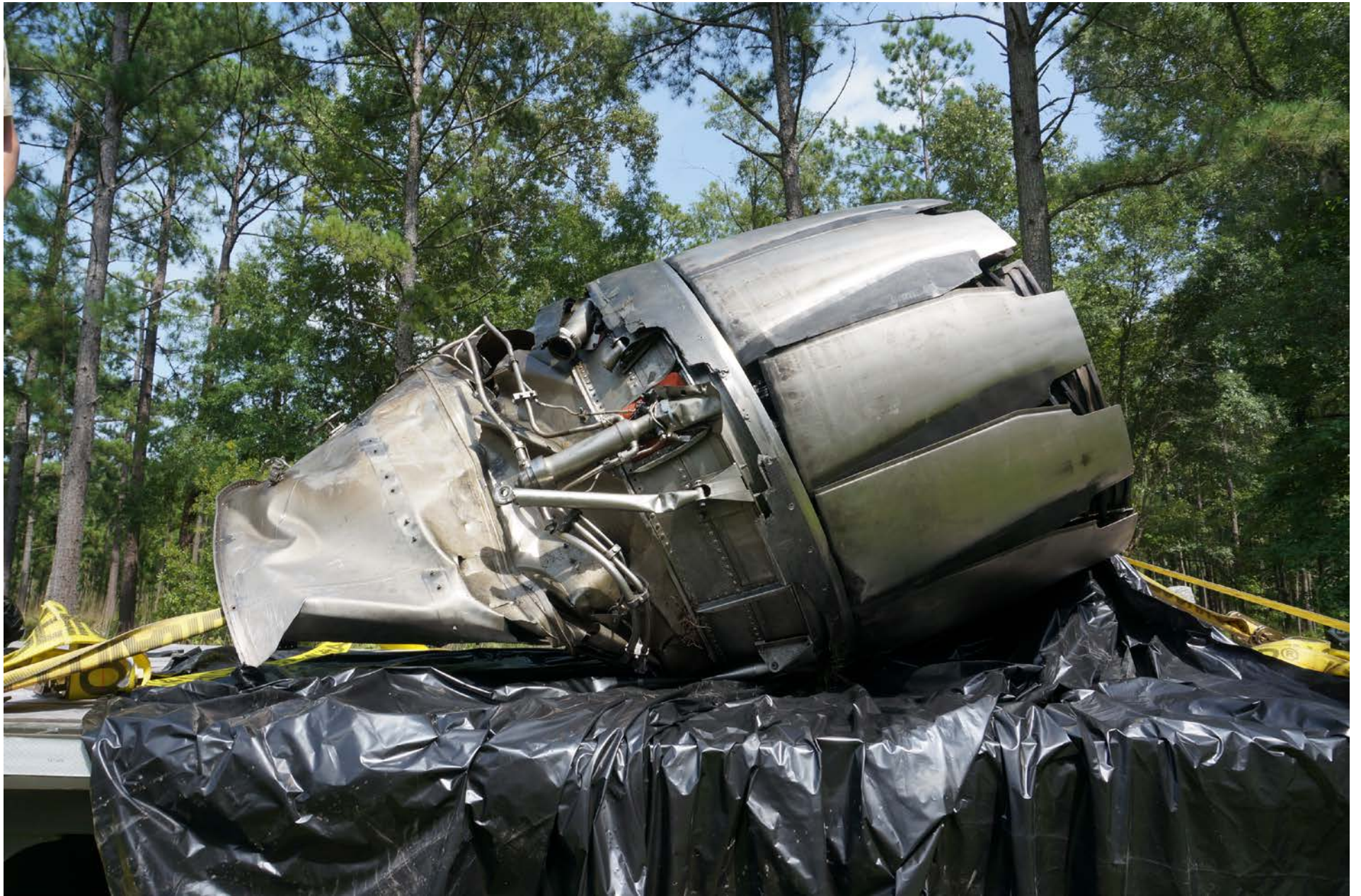
Photo 9 – F-16 Engine Augmenter (Recovered from Collision Site)
