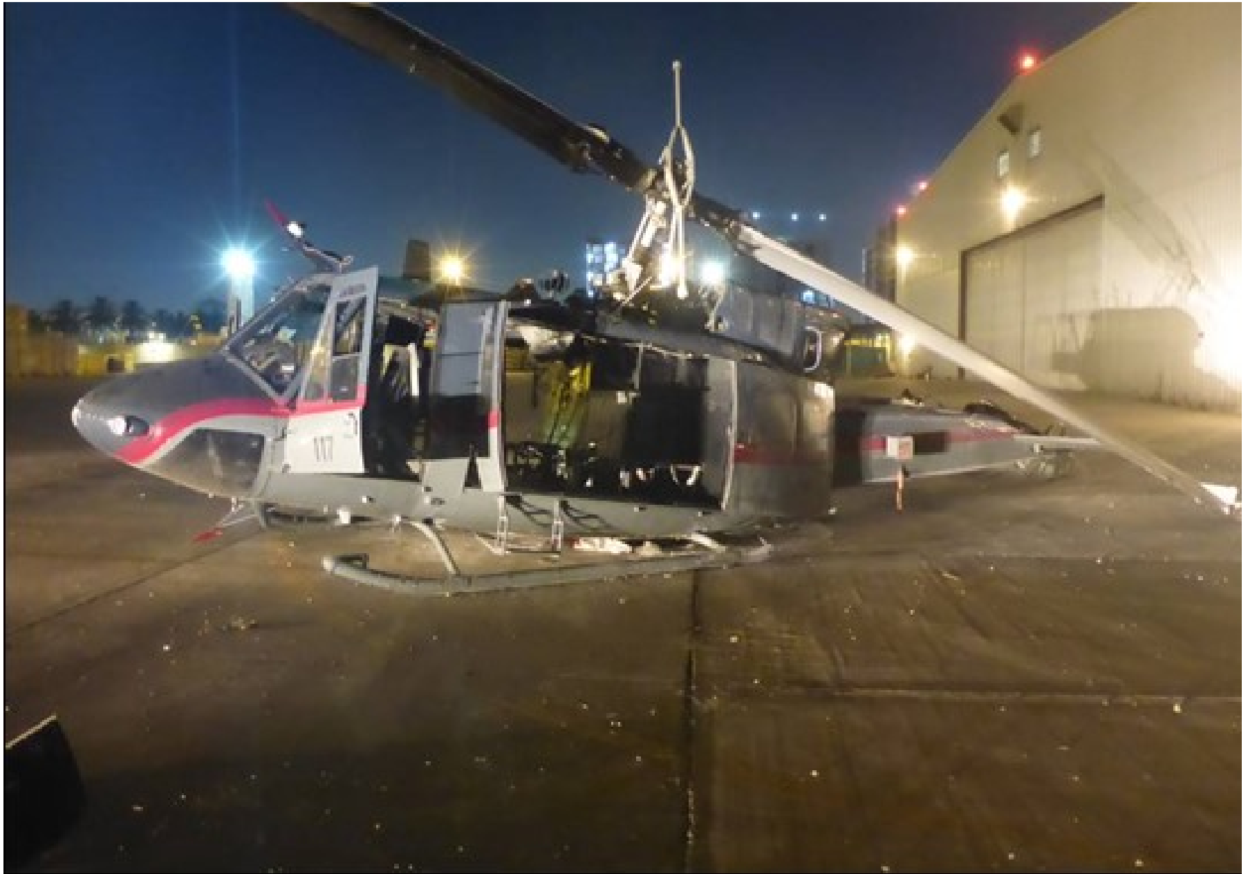
Photo 1 – Post-Accident View of Helicopter (Provided by DOS)
