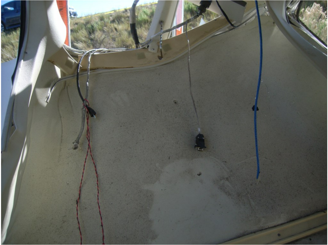
Figure 33 - Cabin Ceiling with Soot Layer
