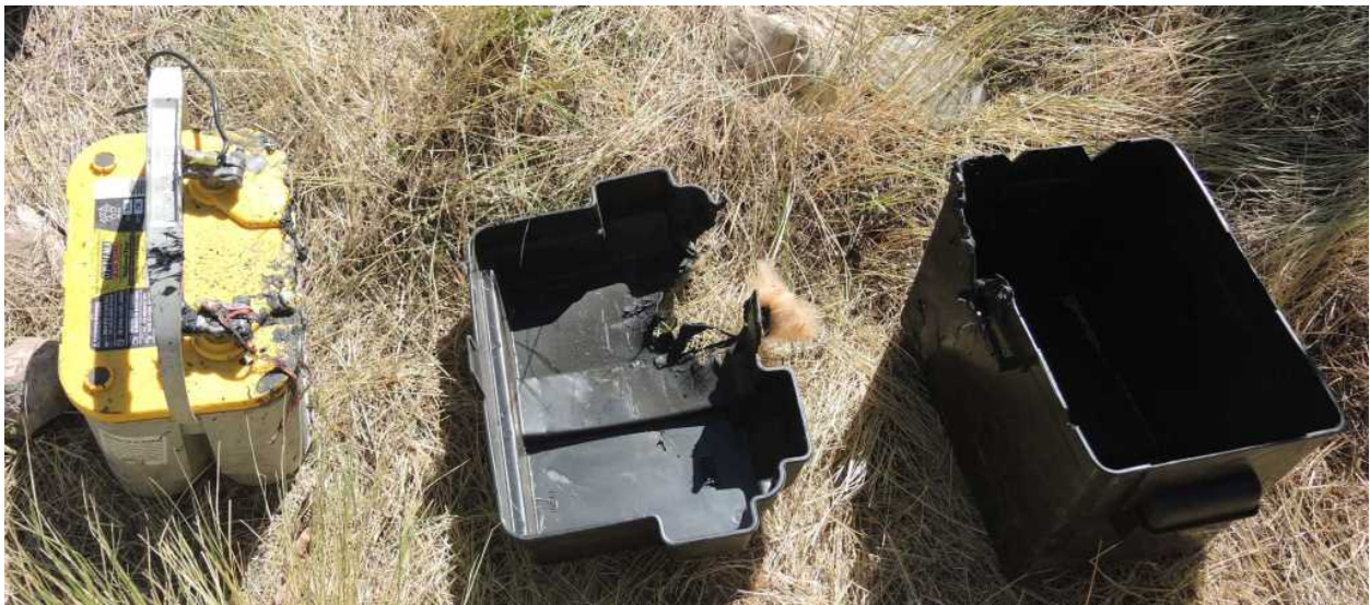
Figure 42 - Battery, Battery Box Cover, and Battery Box (Cessna photo)
