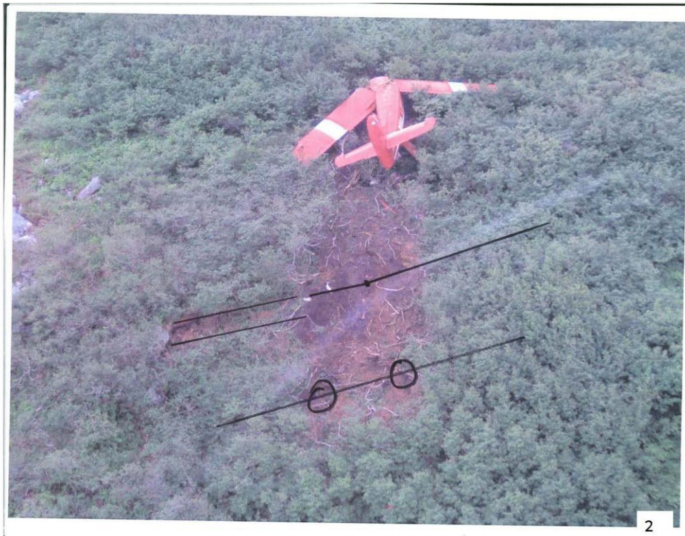
Photo 2- Roll Angle at Impact. The float and left wing ground scars are highlighted.
