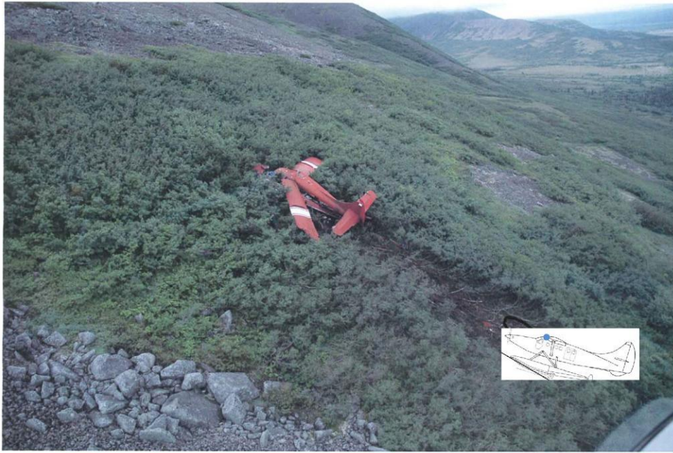
Photo 4 - A two-dimensional photograph of a DCH-3 on floats is rotated 17 degrees up to derive the height of the point at the leading edge of the wing at the centerline (LE/CL) – left float.
