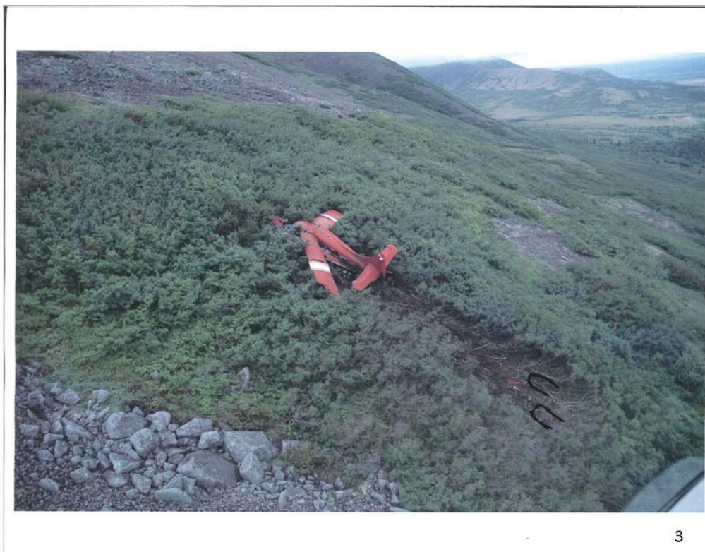
Photo 2- Roll Angle at Impact. The float and left wing ground scars are highlighted.
