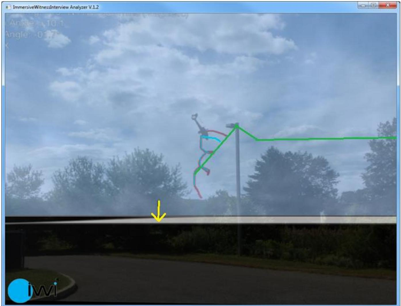
**Figure 6: M. Borek's 2D description (red) combined with the iwi reconstructed flight path (blue), radar data (green) and main wreckage position (yellow arrow)**
