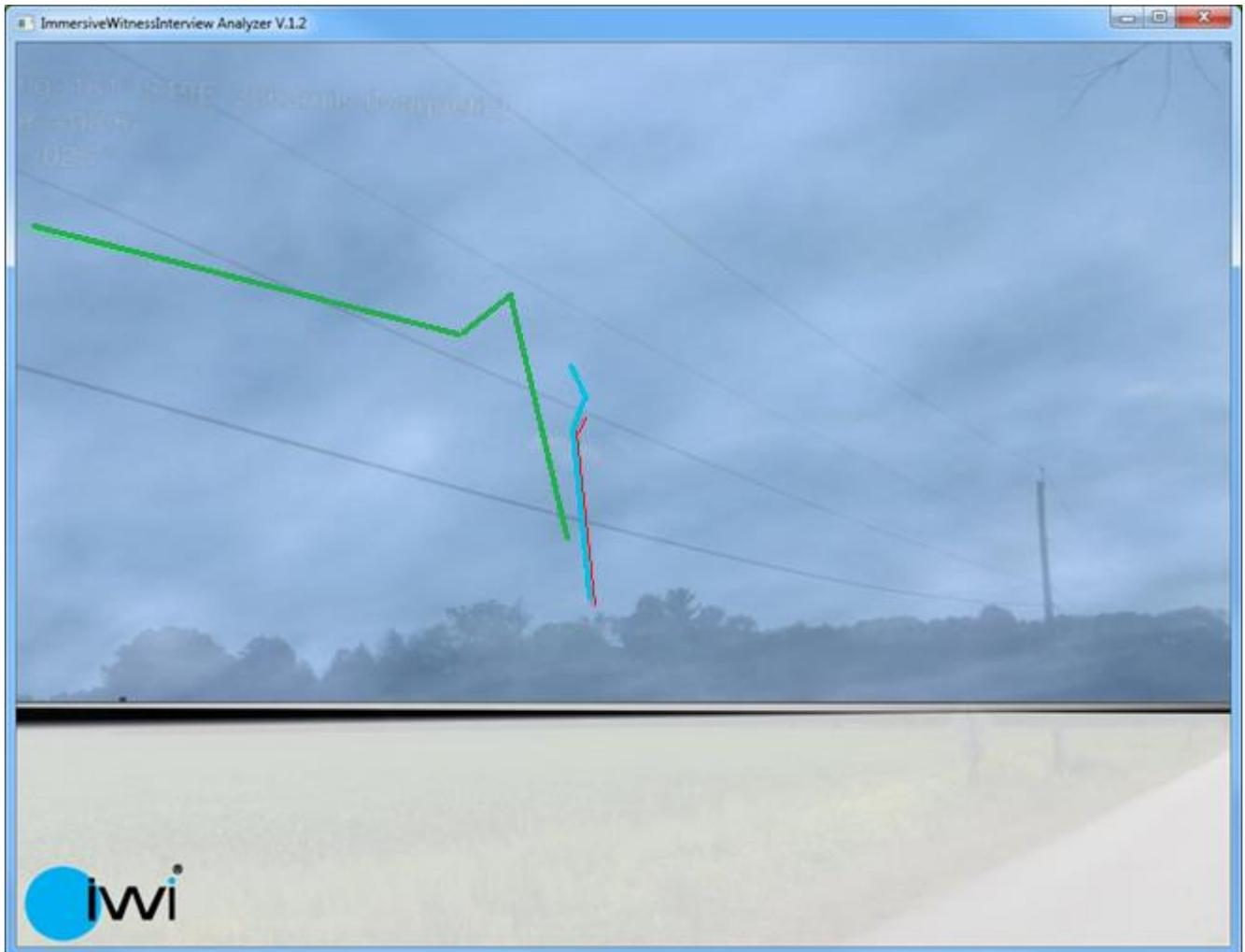
**Figure 12: M. Tellez's 2D description (red) combined with the iwi reconstructed flight path (blue) and radar data (green)**
