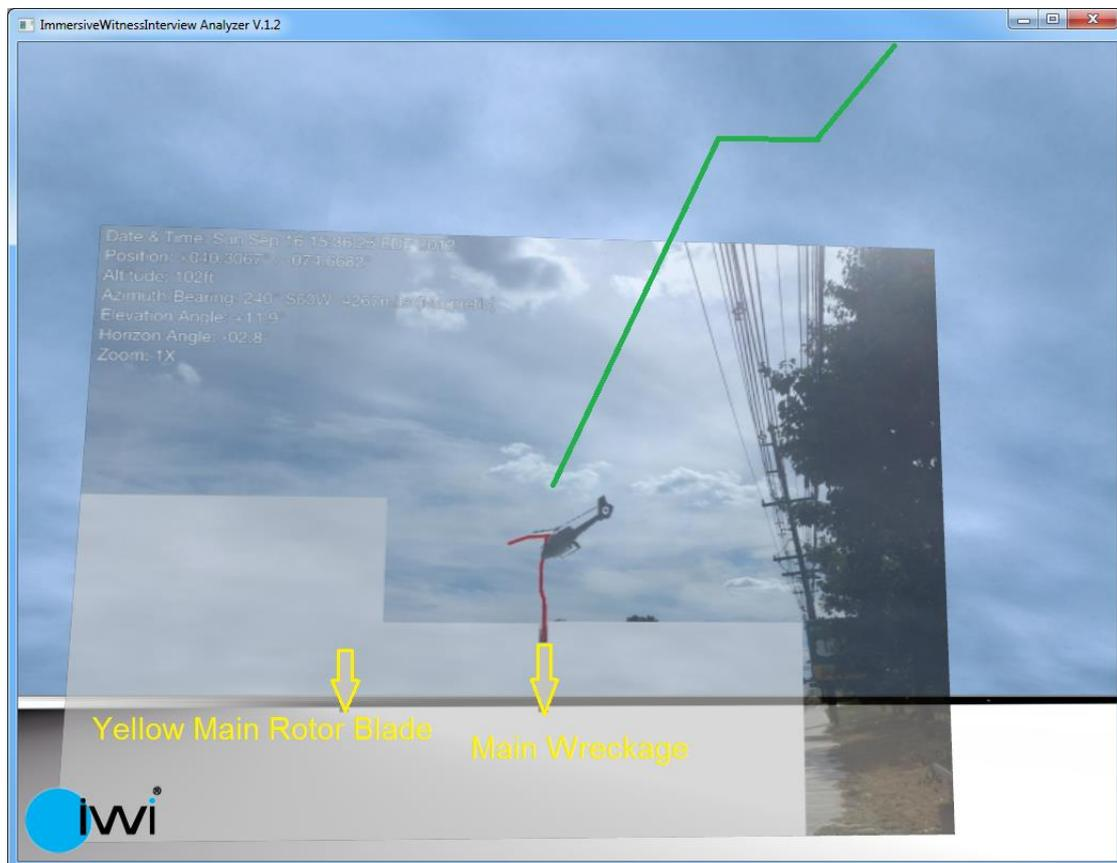
**Figure 11: M. Cox's virtual view at moved position with radar data (green), described flight path (red) and yellow main rotor blade and main wreckage position (yellow arrows)**
