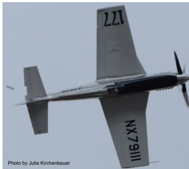
Figure 9. Trim tab separates at 16:24:33.5 PDT
