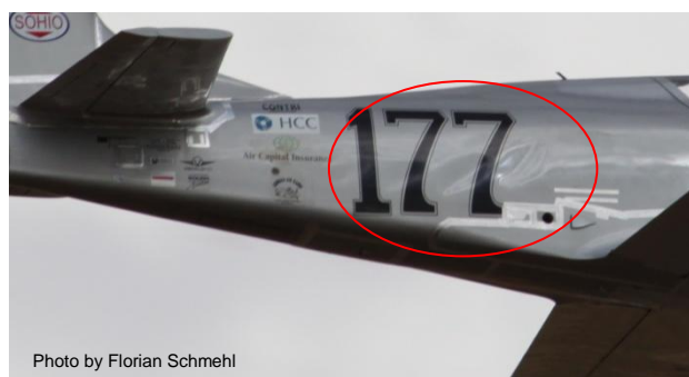
Figure 17. Oil canning on right side during accident flight.
