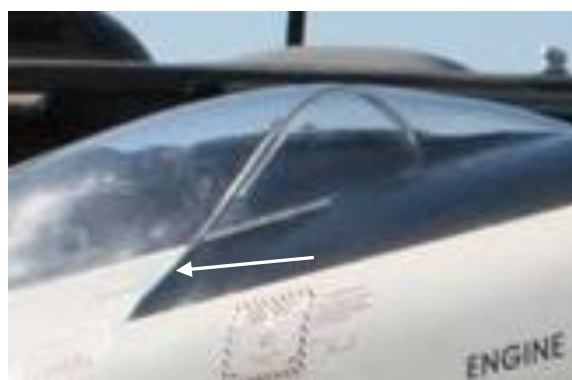
Figure 20. Canopy flush with fuselage on ground.
