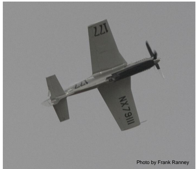
Figure 6. Trim tab begins to separate.
