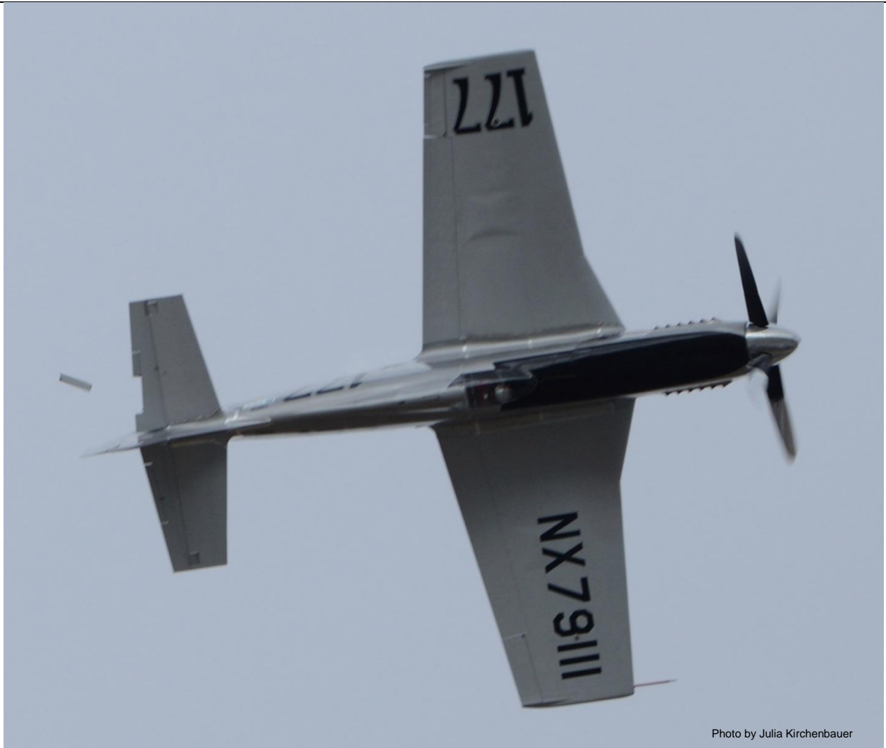
Figure 37. Trim tab separates from aircraft 5.3 seconds after left roll upset.
