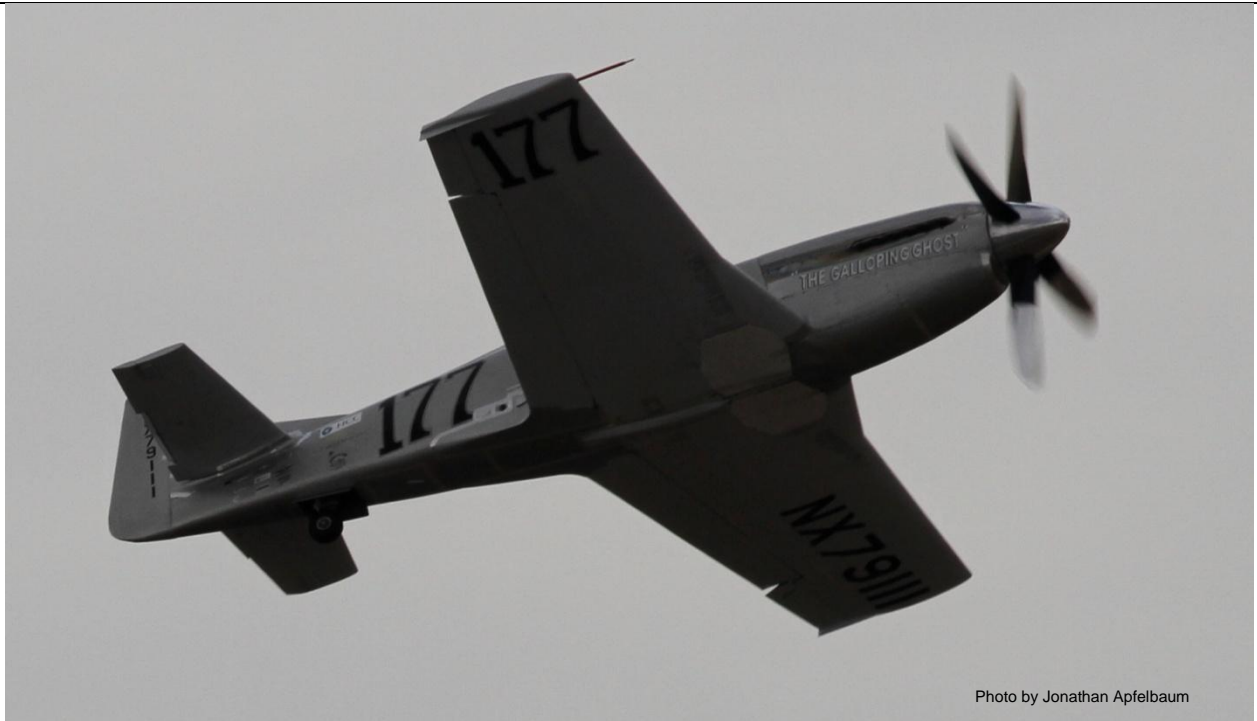
Figure 34. Aircraft pitching up with near full right wing down aileron deflection.
