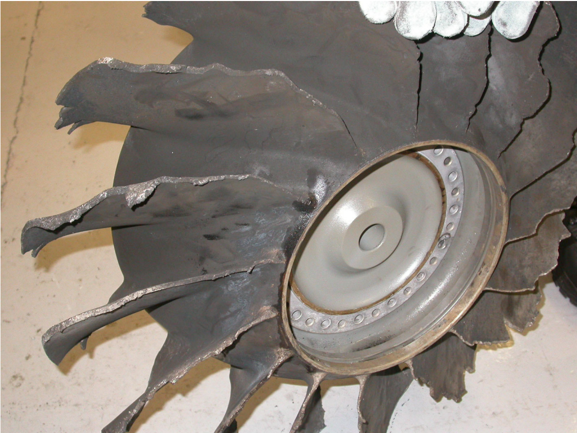
Closer view of damaged inlet fan.
