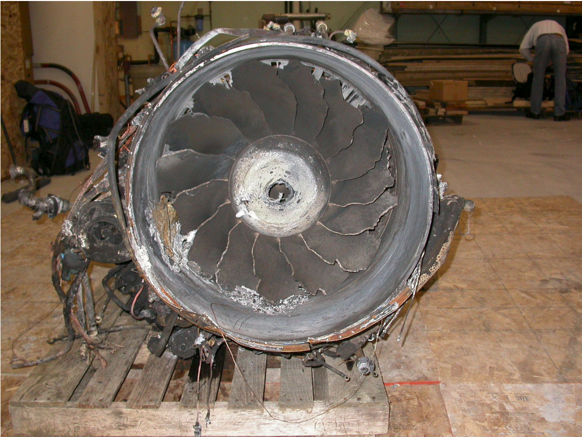
View of inlet fan. Note damage to leading edges.
