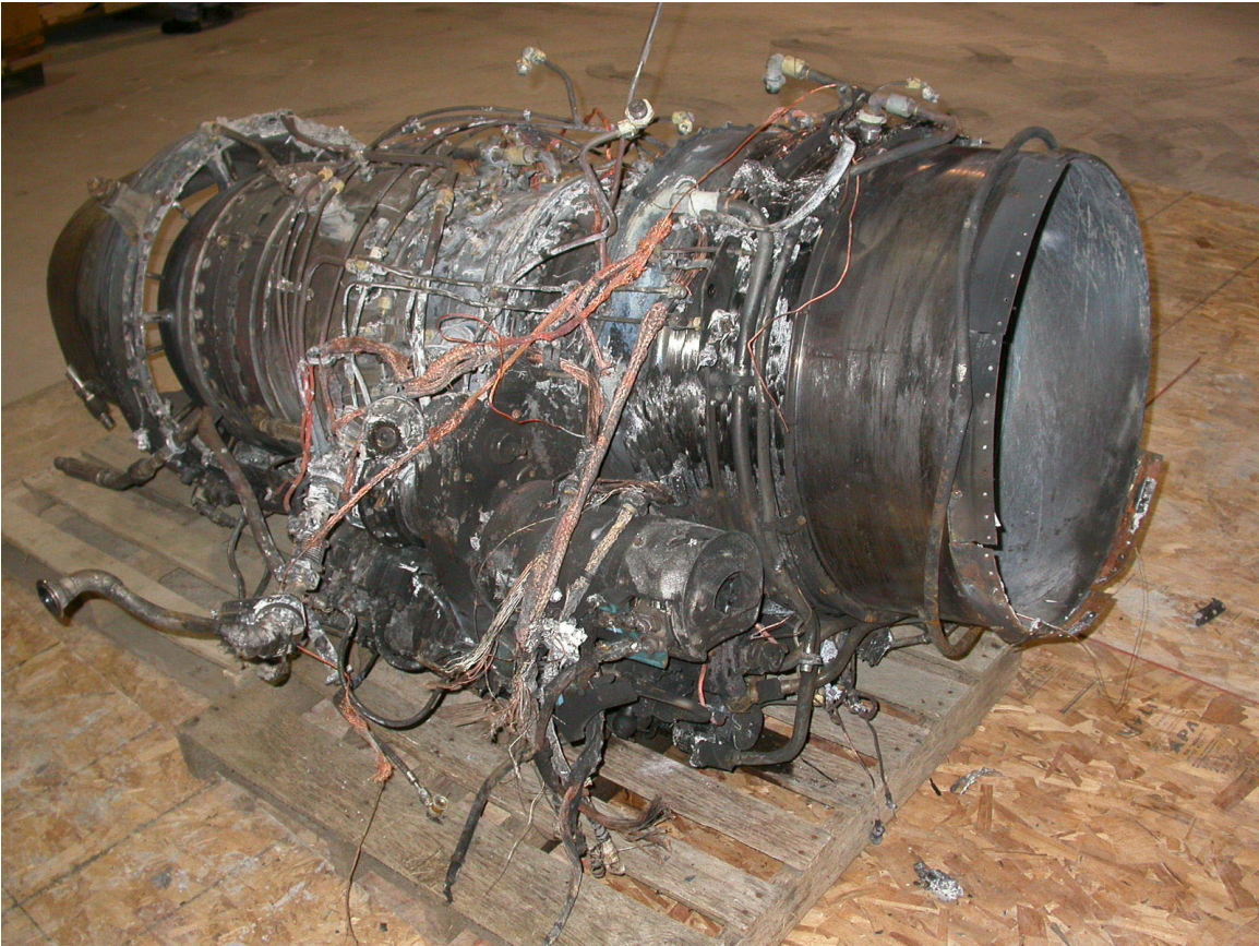
View of fire damaged right side of engine after removal from the airframe
