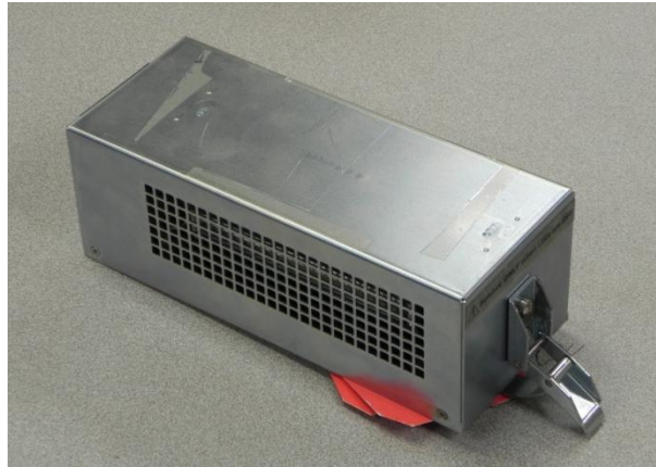
Figure 1. Exemplar Wabtec Traintrax TIR hard drive.
