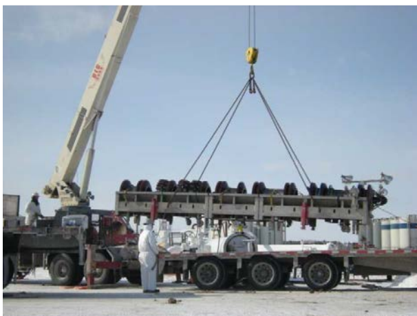
Fig 3- UltraScan™ Duo pipeline inspection tool with phased array ultrasound
