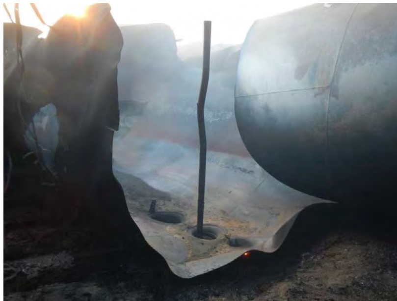
Figure 115: Thermal tear in tank car GATX 33119.
