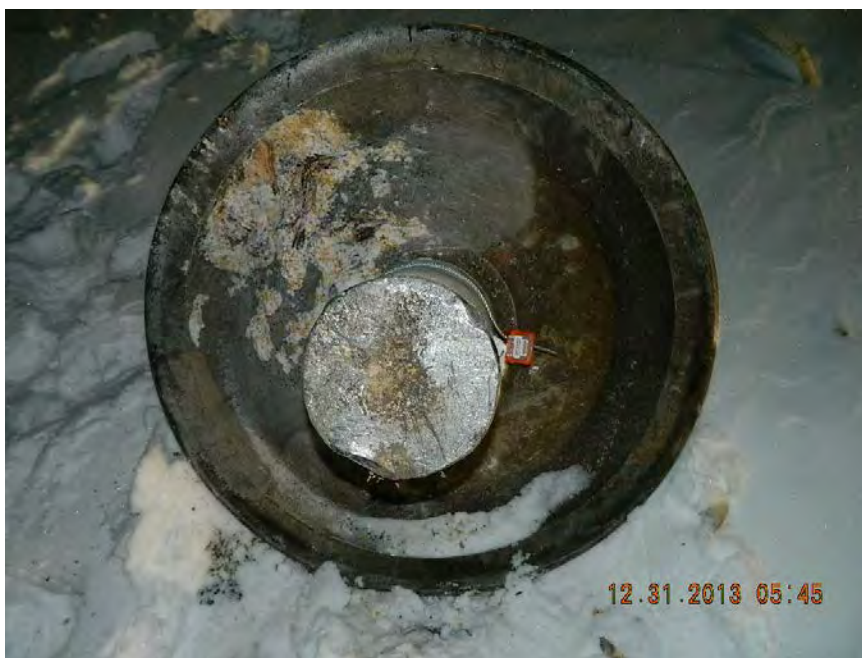
Figure 11. Broken axle assembly as found on-scene; serial number SSD 1102 7A1 E 0912 F.
