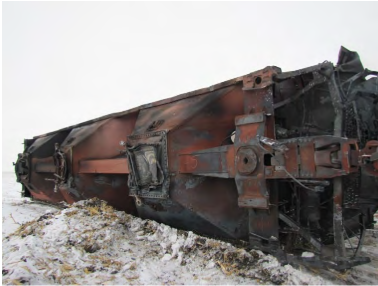
5 6 Figure 5. BNSF 486653, the 45th car with bottom outlet gate damage.
