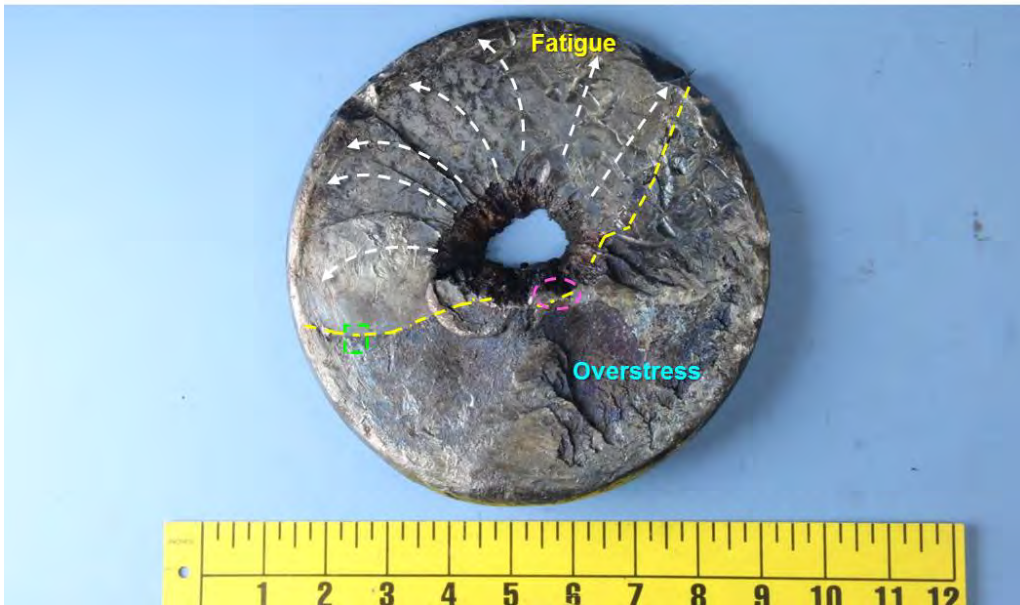
Figure 47 – The fracture surface from Figure 46, after cleaning, with the progressive (latter determined to be fatigue) and overstress areas labeled. The dashed line is the boundary between the progressive and overstress regions. The green dashed box is magnified in Figure 48, and the dashed oval is magnified in Figure 49.
