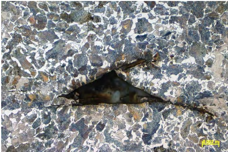
5 6 Figure 58 – Optical metallograph showing the microstructure of the axle, showing a 7 small void, the boxed area in Figure 57 (etched with 2% Nital). 8
