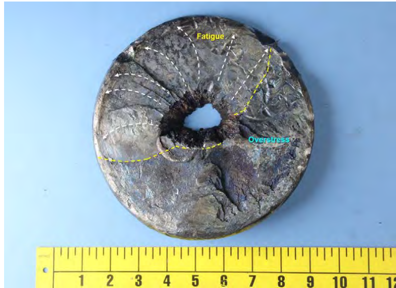
Figure 47 (repeated here). Fracture surface of the broken axle with fatigue and overstress areas labeled
