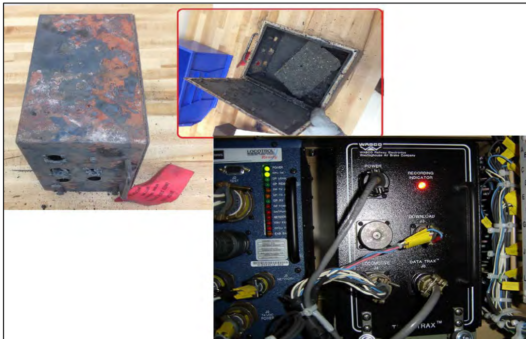
Figure 28. P/T 2nd locomotive BNSF 5958 event recorder and exemplar installation.
