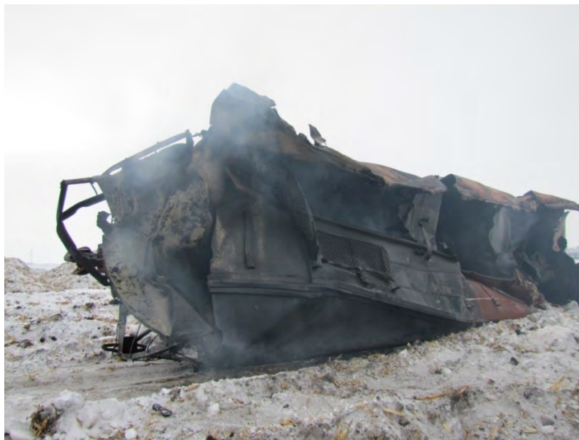
6 7 Figure 7. BNSF 486653, the 45th car, showing car damage on the top of the car. 8
