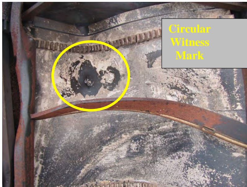
11 12 Figure 6. BNSF 486653, the 45th car, with 8-inch diameter circular witness mark.
