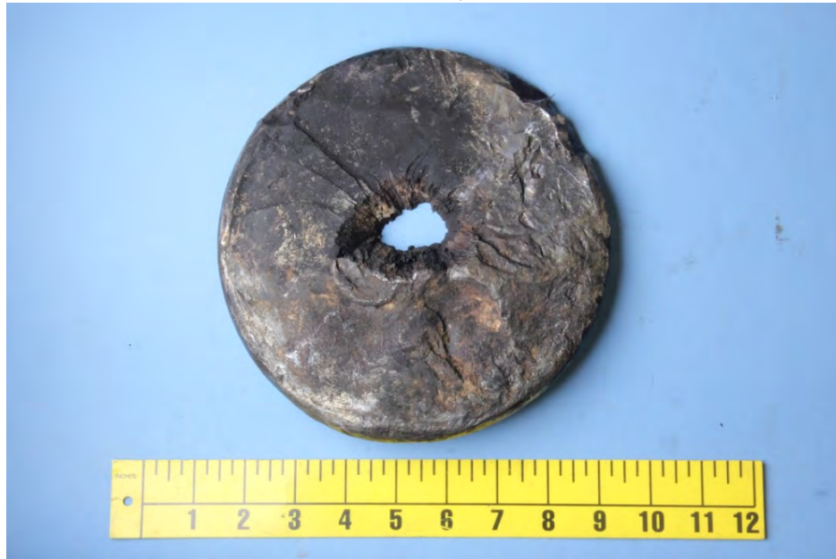
Figure 46 – The longer axle segment fracture surface, after removal.
