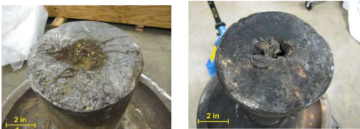
Figures 41 and 42. Mating fracture surfaces of the axle received.
