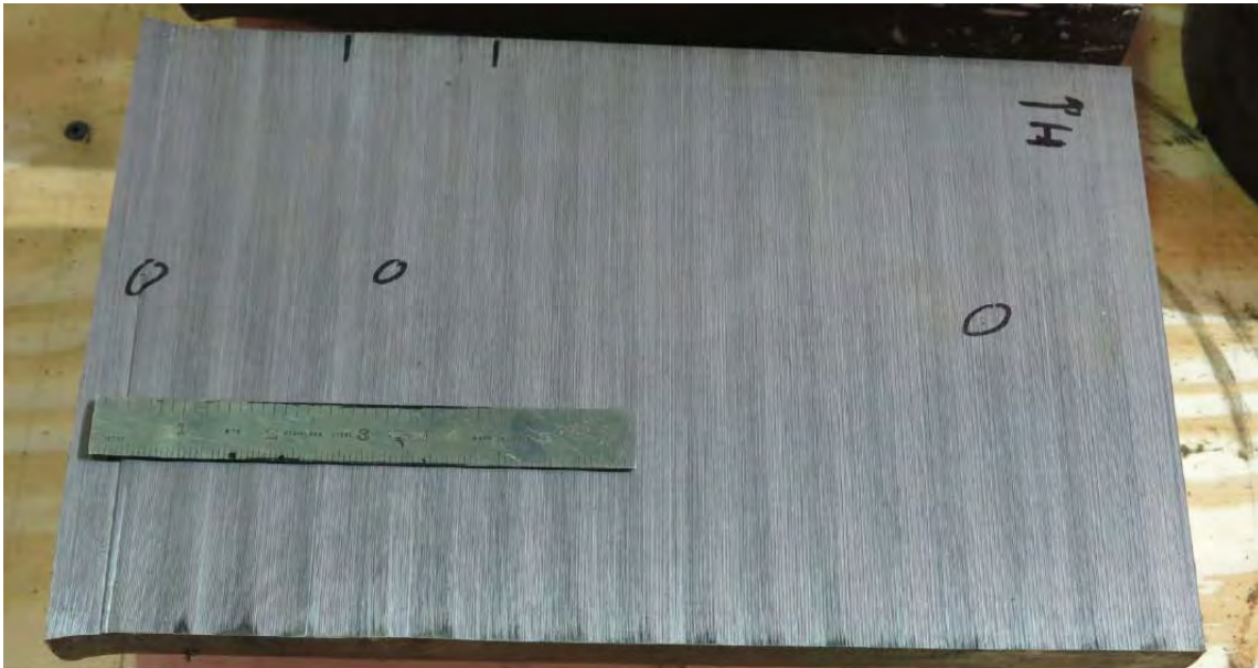
Figure 54 – Cross section of the short side axle fragment, showing three small voids along the centerline.
