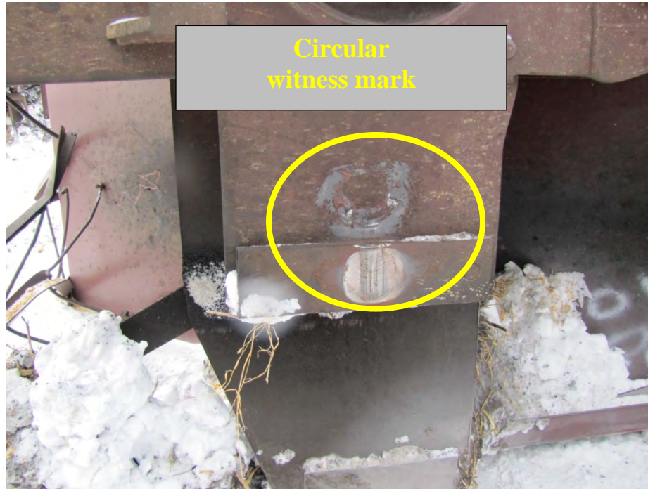
9 10 Figure 10. BNSF 480263, the 48th car, with 8-Inch diameter circular witness mark.
