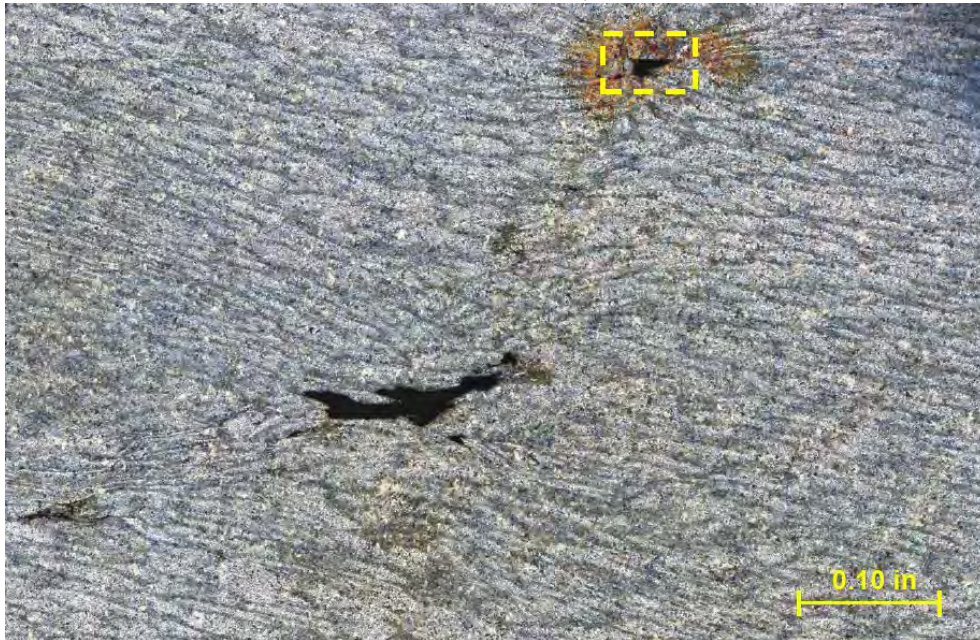
1 2 Figure 57 – Optical metallograph of a cross-section through a small void in the 3 centerline of the axle (etched with 2% Nital). The boxed area is shown in Figure 58. 4
