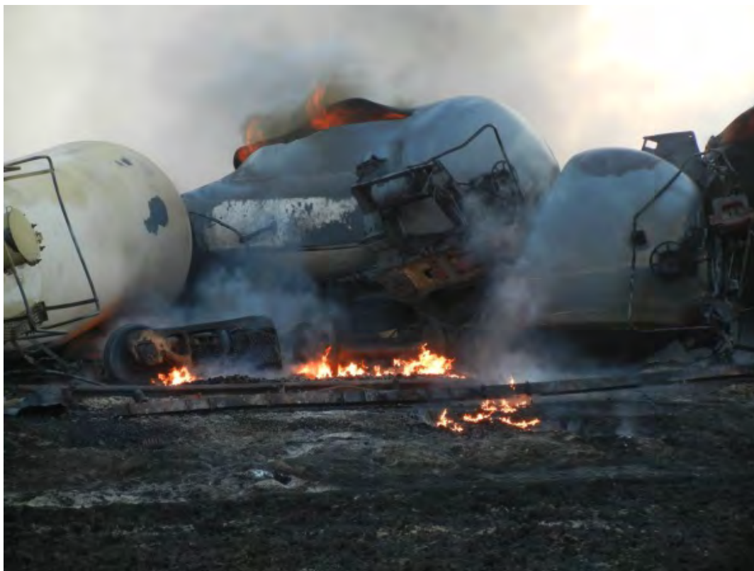
10 Figure 46: Fire coming out of thermal tear in top of the tank car GATX 33125.
