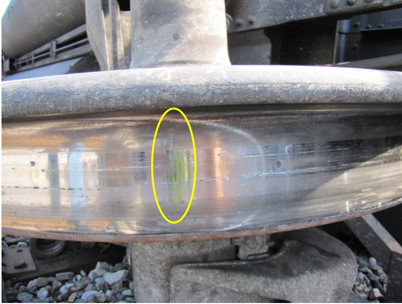
2 Figure 3 - Photograph of Witness Mark on CSXT 398511, Wheel R4
