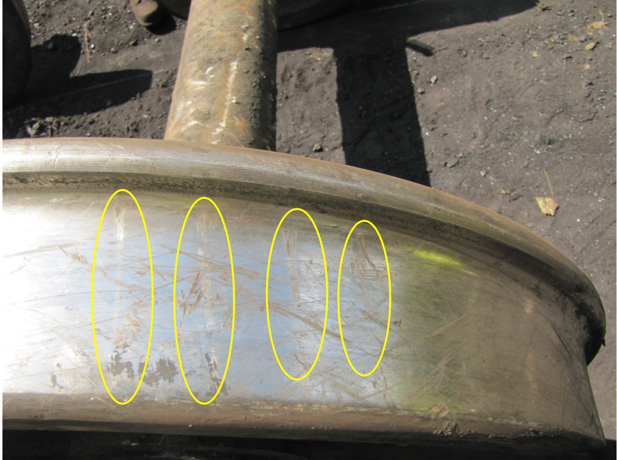
2 Figure 5 2- Photograph of Witness Marks on Wheel R3 from CSXTT 302724
