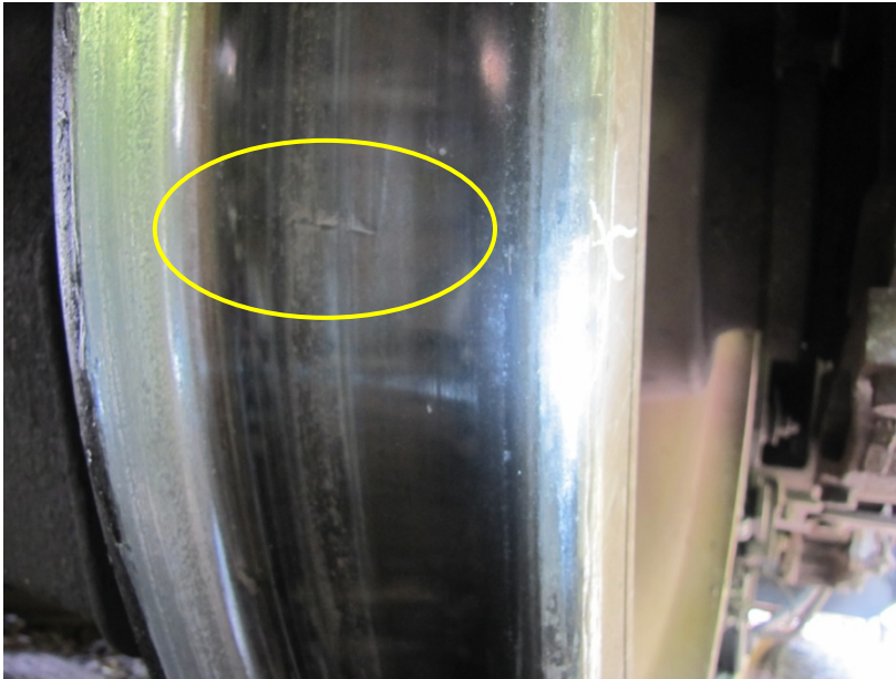
3 Figure 2 - Photograph of Witness Mark on CSXT 4579, Wheel R1
