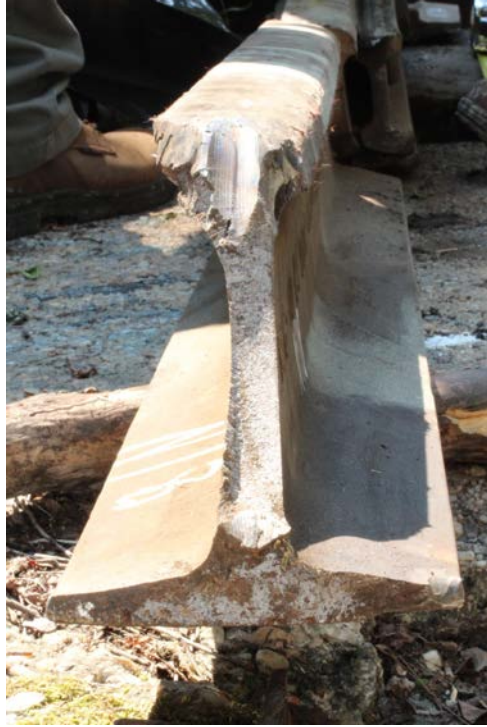
1 2 Figure No. 6. A view of a severe wheel 3 flange strike mark on piece No. "N 18". 4
