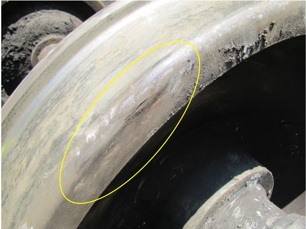
2 Figure 6 - Photograph of Corresponding Witness Mark on Wheel L3 from CSXT 302724
