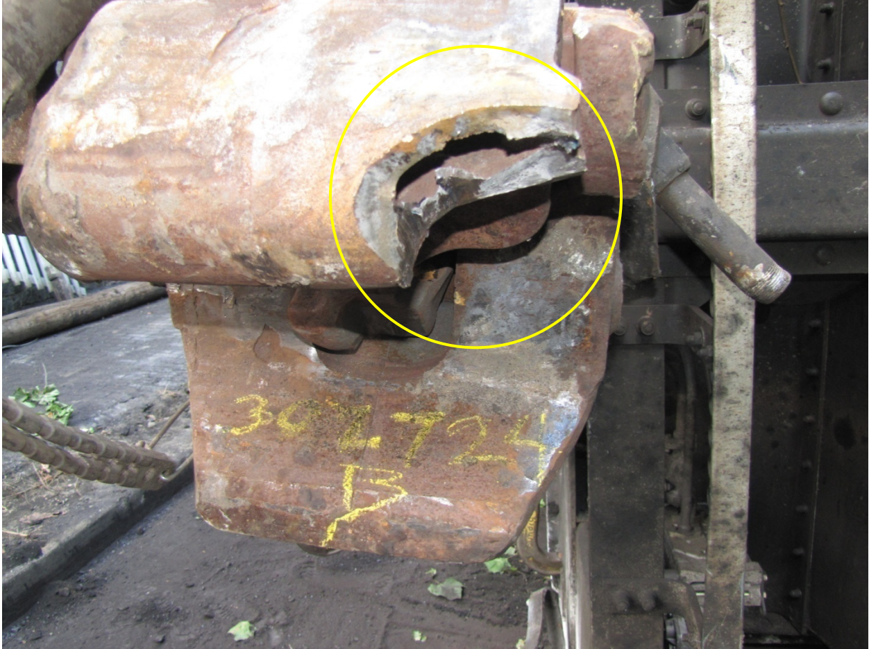
2 Figure 8 3- Photograph of CSXT 302724 B-End Fractured Knuckle Assembly
