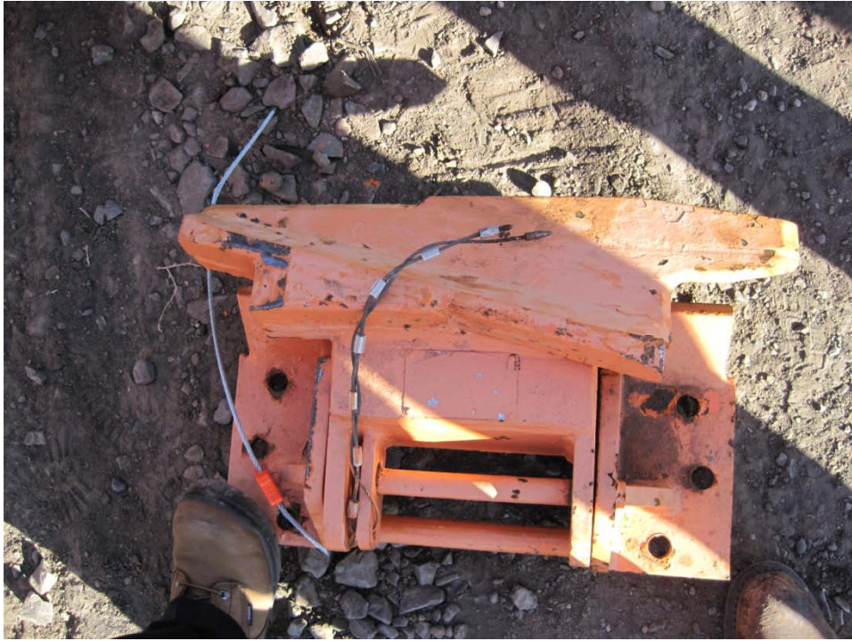
Figure 3 Photograph of the Hinged Derail Involved in the Accident
