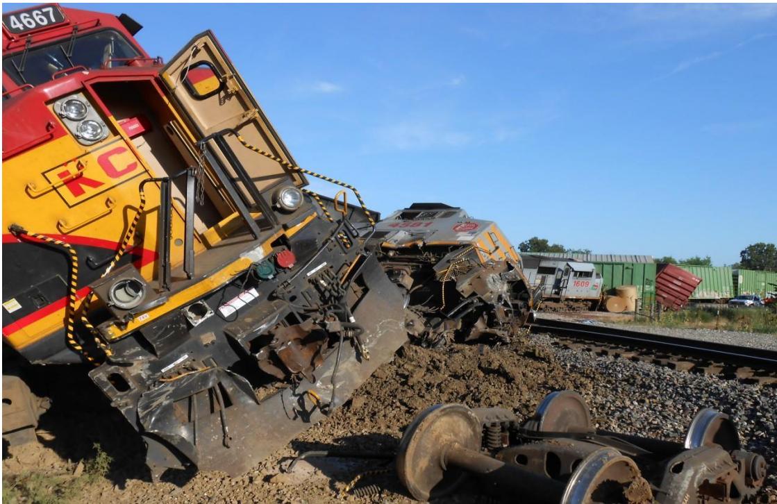
Figure No. 1 – Kansas City Southern locomotive No. 4667 derailed as a result of side collision with BNSF train near Arcadia, KS.
