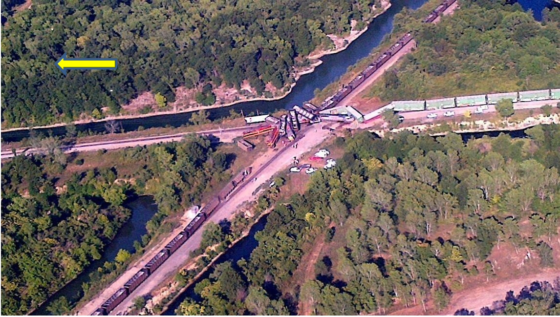
Figure No 2. – Overview of accident site. KCS train operating right to left. BNSF train operating from upper right to bottom left (arrow indicates north).
