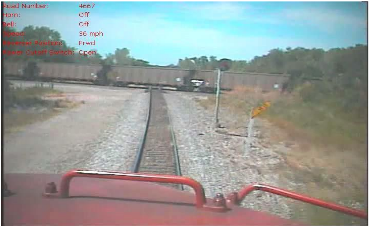
Figure 4. This photograph was taken by the KCS freight train's outward facing camera positioned on the lead locomotive. The railroad crossing Home signal can be seen ahead of the train on the right side of the tracks. The KCS train is likely less than 10 seconds before impact with the BNSF train, which is now traversing the railroad crossing. It is estimated that this was the point where the KCS crew jumped from the lead locomotive.
