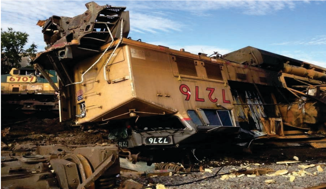
Figure 2. Photograph of the lead locomotive of Train MSIDV 15. The locomotive 7276 is upside down and has rotated 180°. (Photo by Union Pacific)
