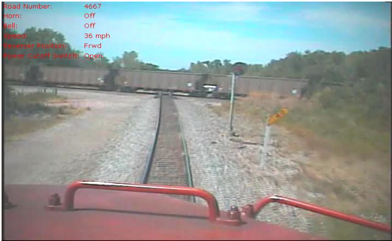
Figure 4. This photograph was taken by the KCS freight train's outward facing camera positioned on the lead locomotive. The Home signal can be seen ahead of the train on the right side of the tracks. The KCS train is likely less than 10 seconds before impact with the BNSF train, which is now traversing the interlocking. It is estimated that this was the point where the KCS crew jumped from the lead locomotive.
