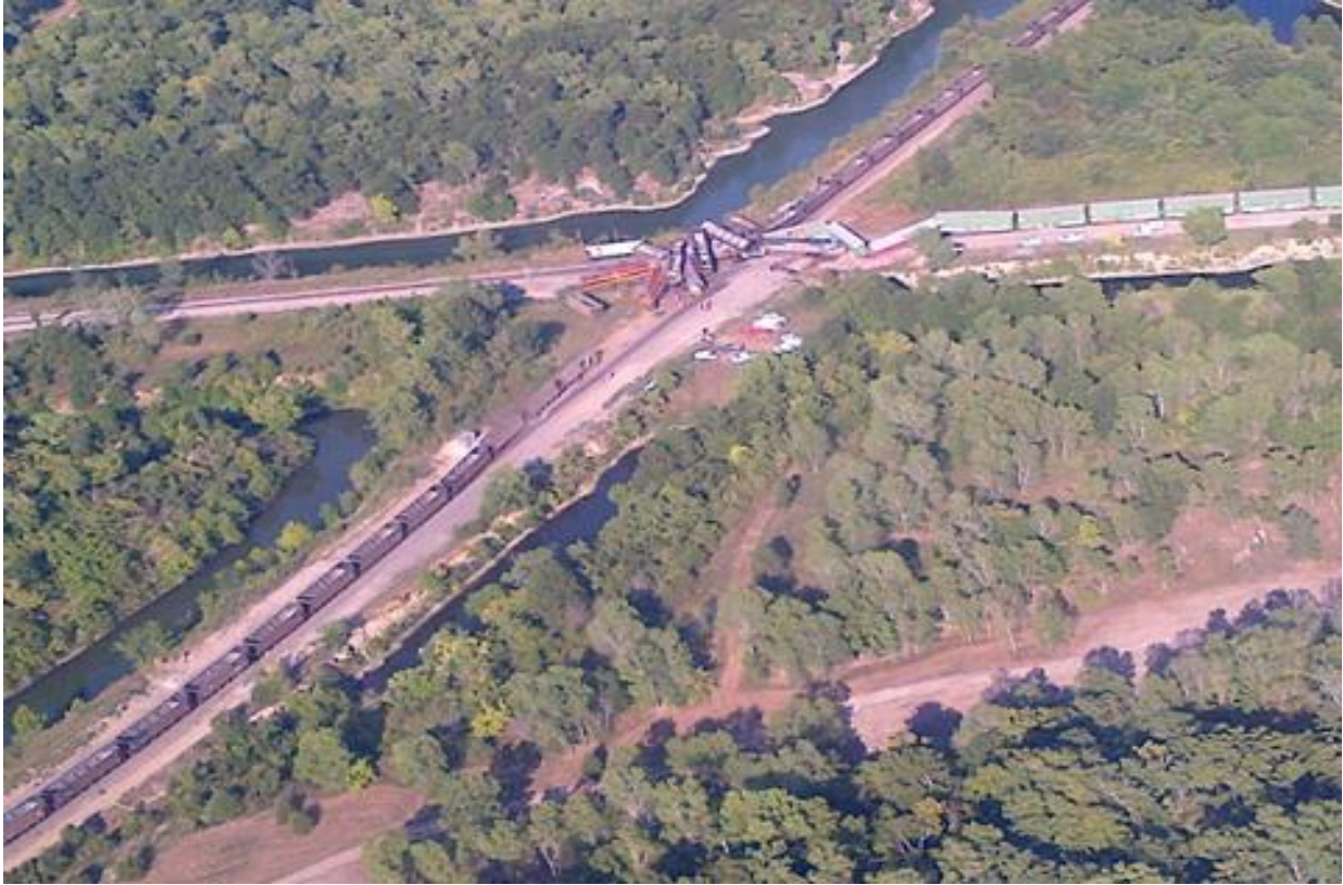
Figure 1. Aerial picture shows a northbound Kansas City Southern Railroad mixed freight train (pictured traveling from right to left) that had collided into the side of a westbound BNSF Railway empty unit coal train (pictured traveling from top to bottom) at a joint KCS / BNSF diamond crossing near Liberal (Barton County), Missouri.
