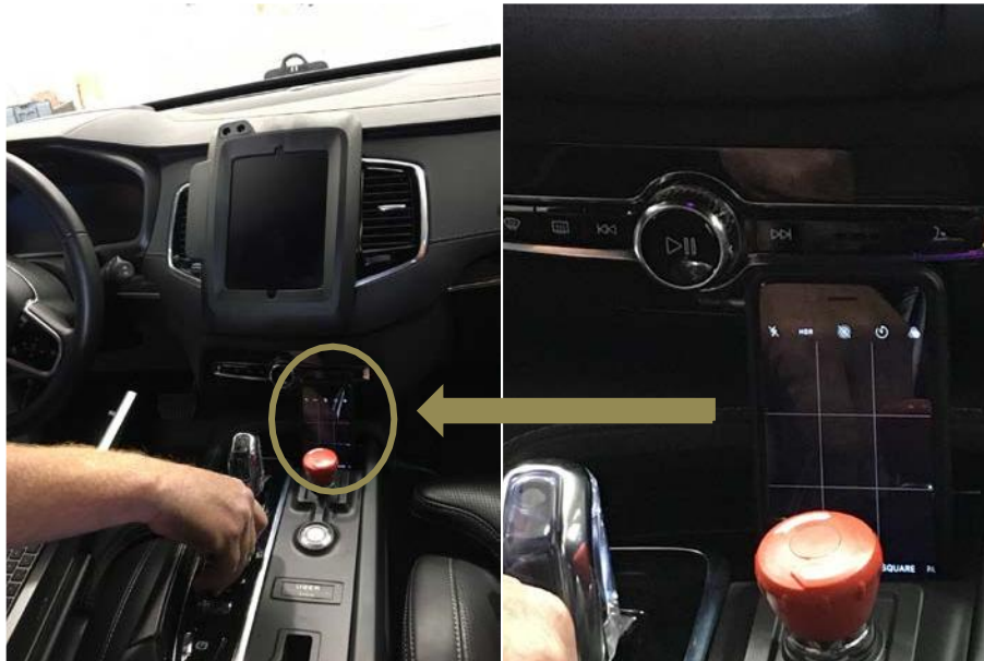
Figure 1. The interior of the accident vehicle, with an exemplar cell phone placed in a slot under the Uber-mounted tablet computer.
