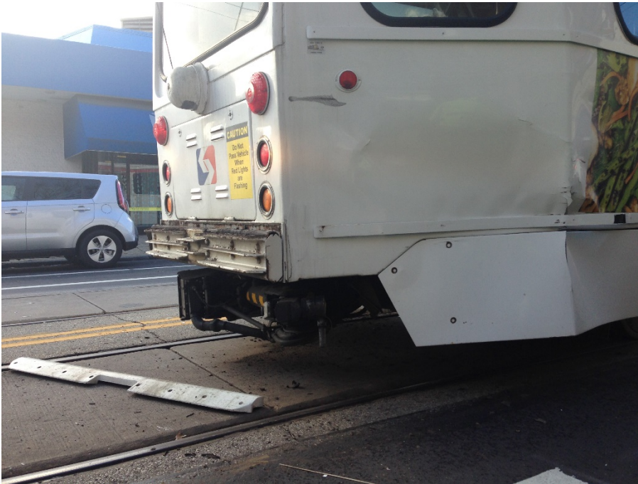
Figure 2: Photo of SEPTA Trolley 9101 with bumper displaced from vehicle and laying on the ground (photo courtesy of SEPTA).
