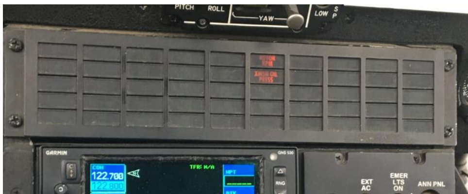
Photo 9: Caution/warning panel; instrument lights set to “BR”; transfer pumps “ON”; taken outside/daylight.
