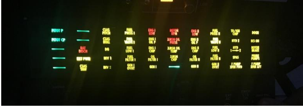
Photo 14: Caution/warning panel; instrument lights set to “OFF”; depressing annunciator panel test switch; taken about 15 minutes after sunset.
