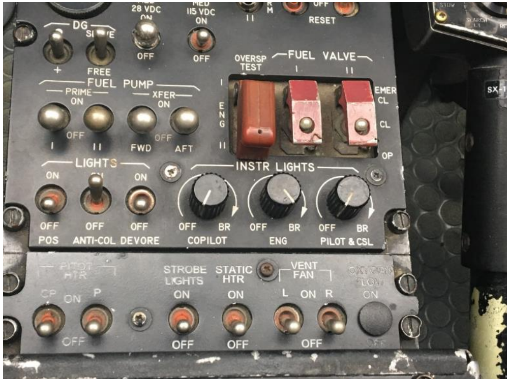
Photo 13: Center console showing location of FUEL PUMP switches and INSTR LIGHTS dials; taken outside/daylight.
