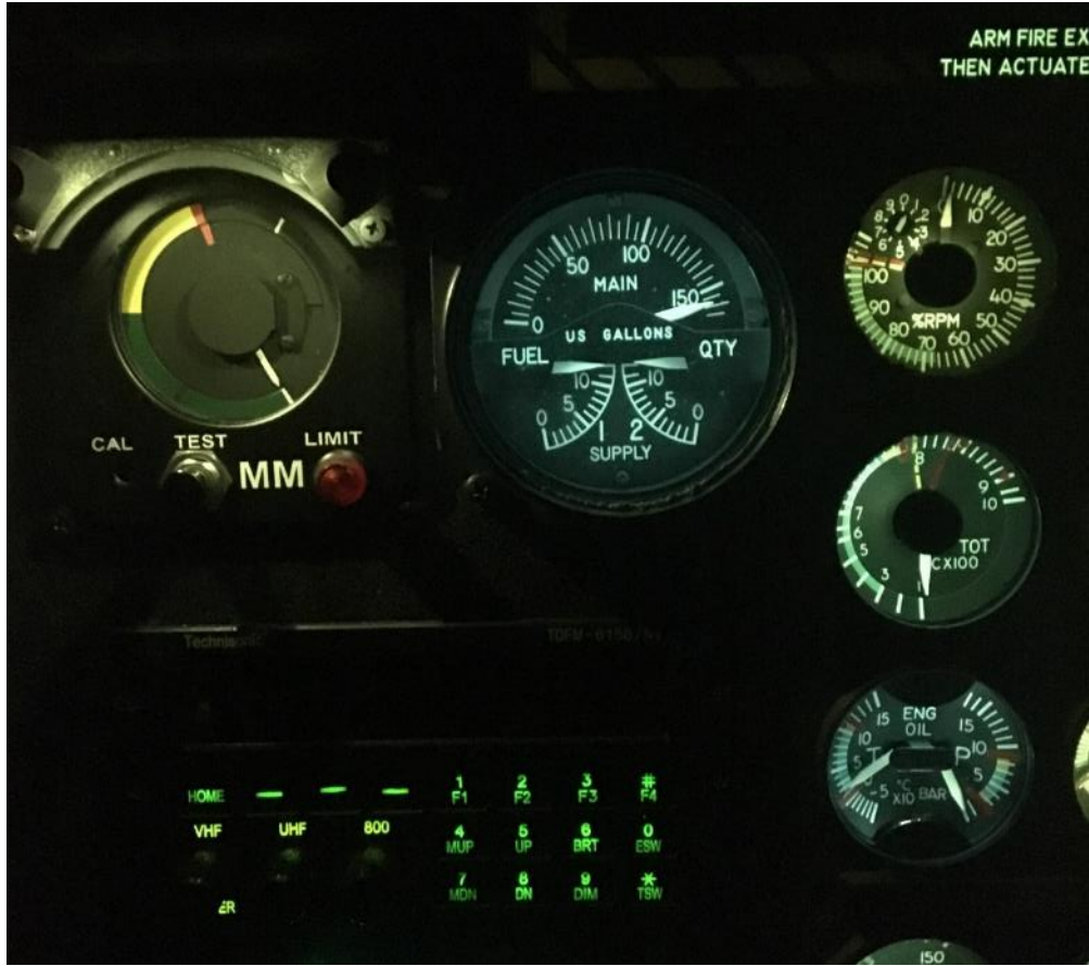
Photo 6: Fuel gauges; instrument lights set to “BR”; taken in hangar with hangar lights off.
