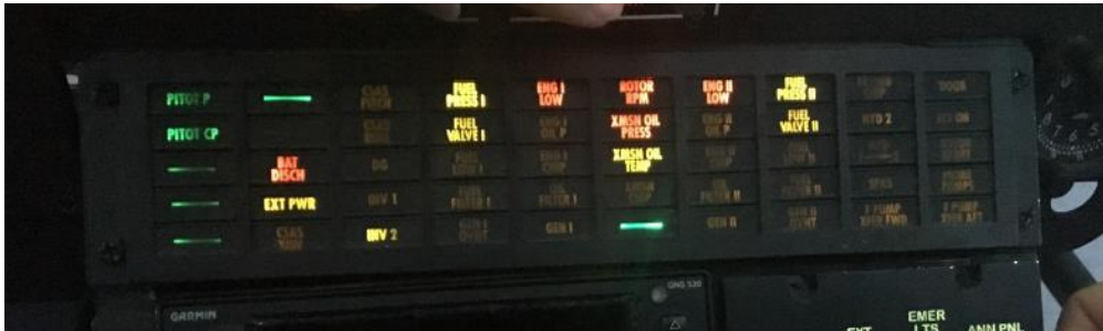
Photo 15: Caution/warning panel; instrument lights set to “BR”; depressing annunciator panel test switch; taken about 15 minutes after sunset.
