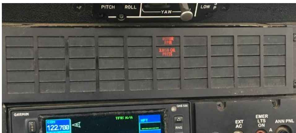
Photo 8: Caution/warning panel; instrument lights set to “BR”; transfer pumps “Off”; taken outside/daylight.
