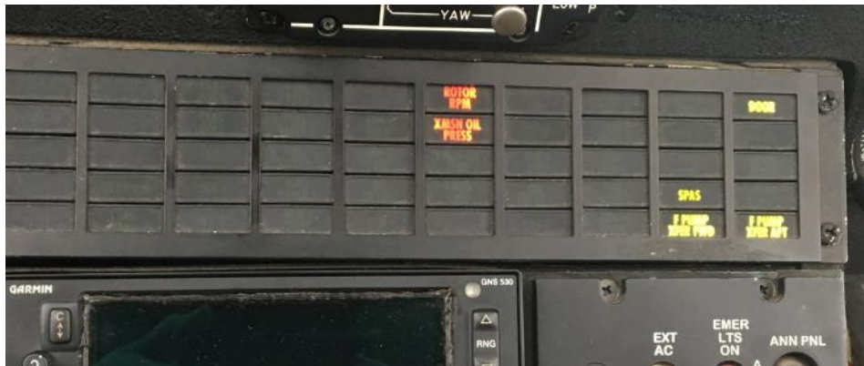
Photo 7: Caution/warning panel; instrument lights set to “Off”; transfer pumps “Off”; taken outside/daylight.
