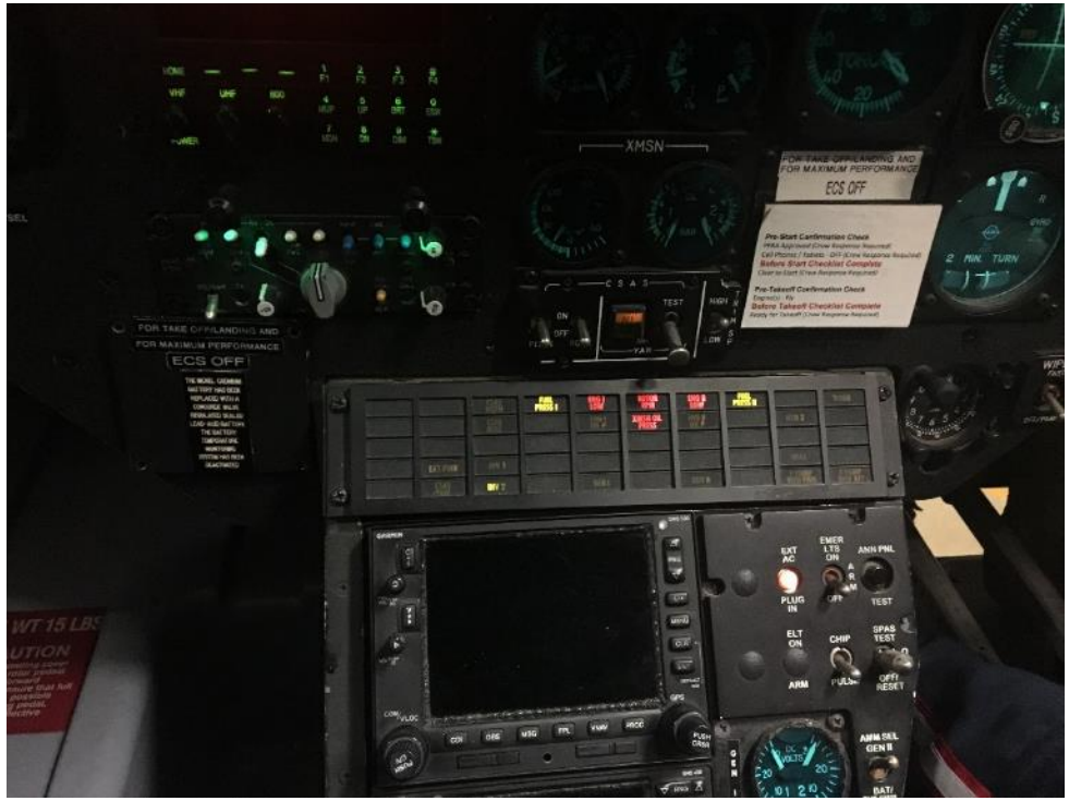
Photo 3. Caution/warning panel; instrument lights set to “BR”; transfer pumps “OFF”; taken in hangar with hangar lights on.
