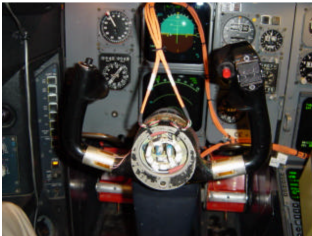
Figure 3: The instrumented control wheel.
