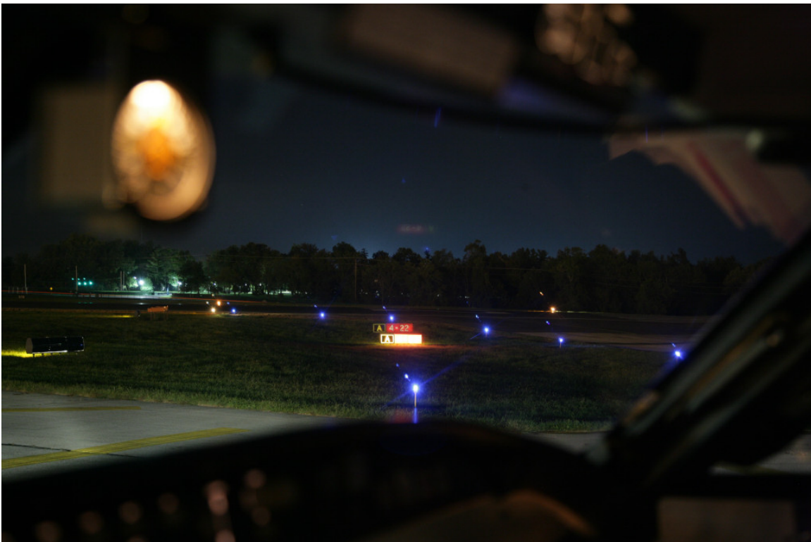
Figure 6. Position 7 – View through right windshield of RW 22 hold short line. (Image is overexposed. Horizon was not visible. RW 4-22 sign washed out and refracted.)
