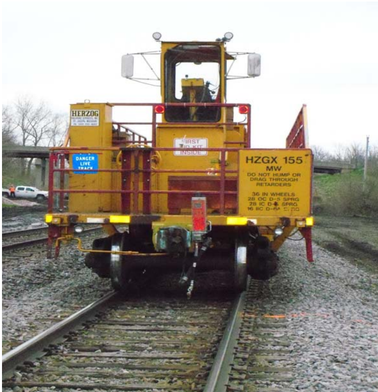
Clip car with an end of train (EOT) device (red) and reflectors.
