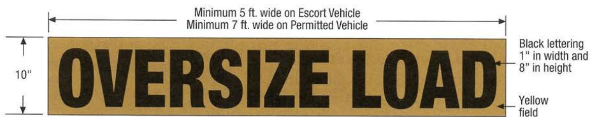
FIG. 2.7.2-1 OVERSIZE LOAD SIGN
