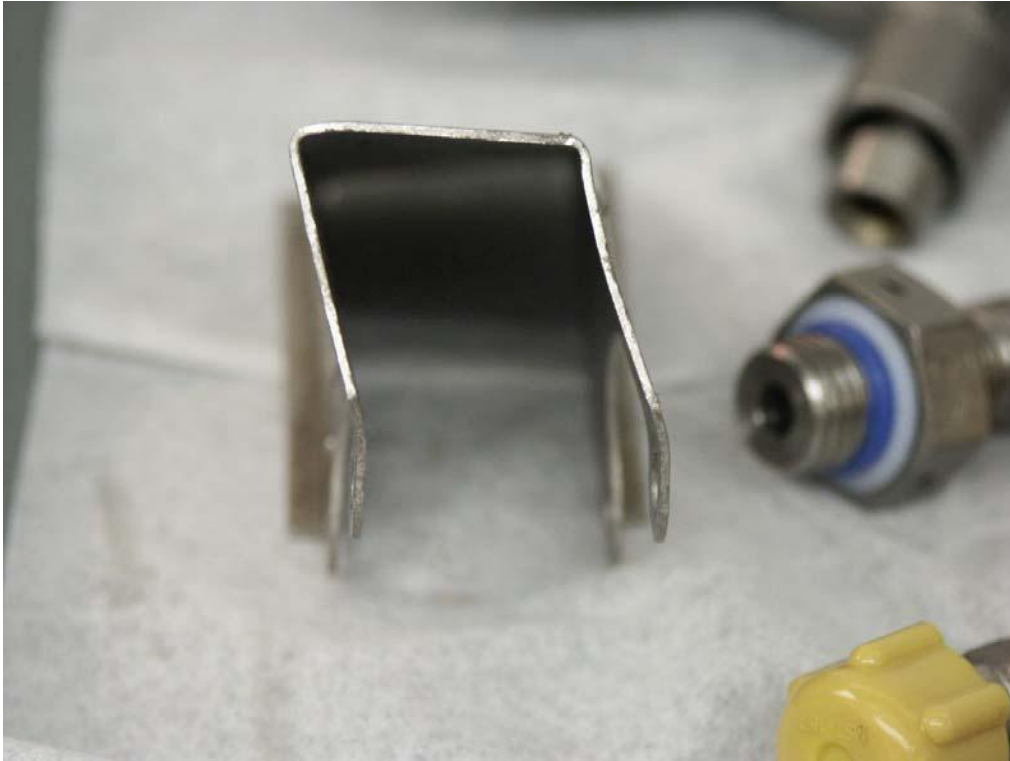
Figure 11 deformation of manual override shield
