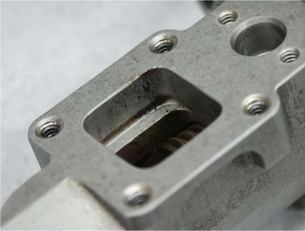
Figure 33 wear debris in bellows MOR cavity
