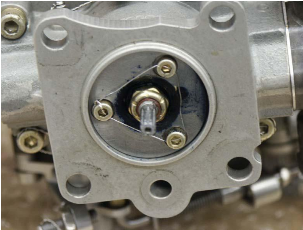
Figure 9 drive pad blue grease dilution
