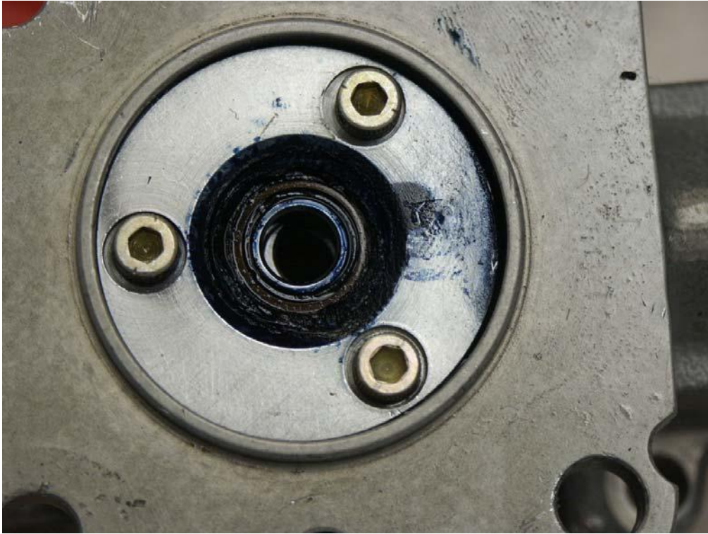
Figure 25 drive pad with driveshaft removed
