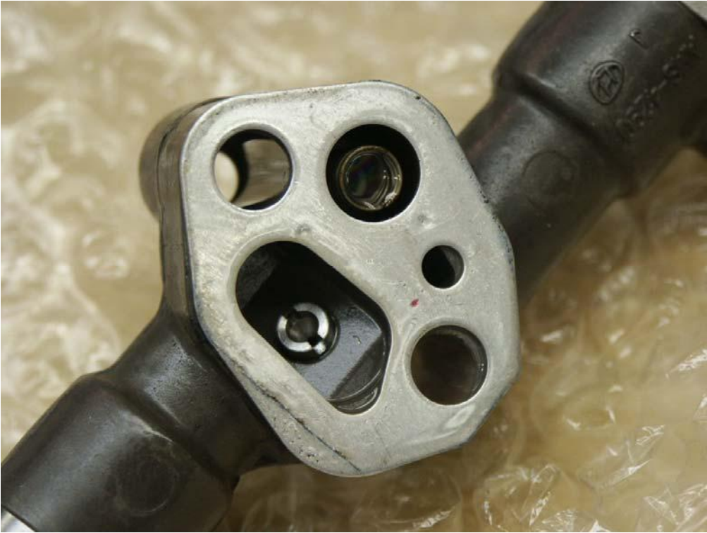
Figure 13 air adapter cavity and gasket wet with fuel
