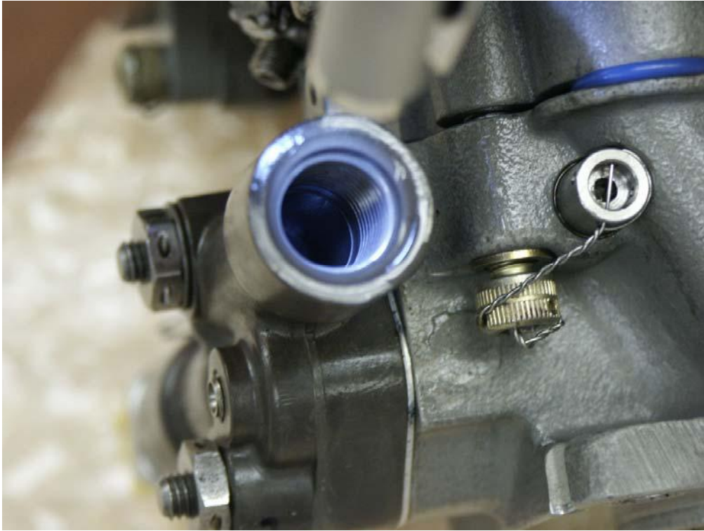
Figure 17 air adapter Pc inlet wet with fuel
