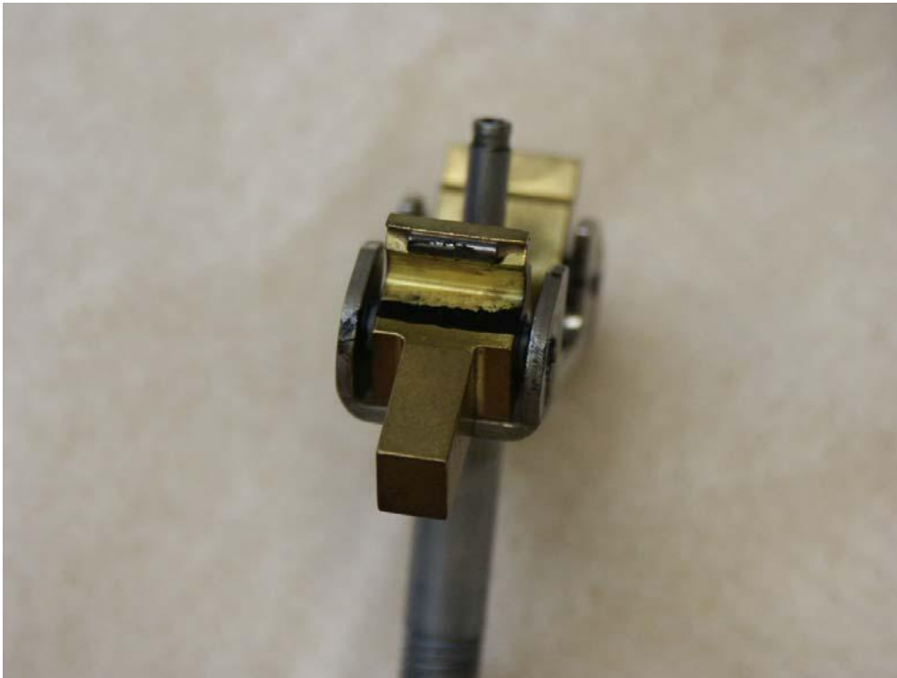
Figure 22 ribbon of blue grease on flyweight
