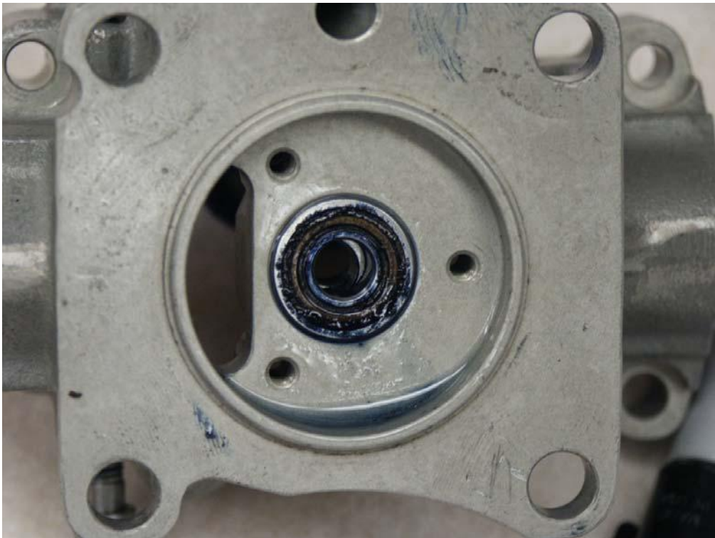
Figure 26 fuel found underneath drive bearing retaining plate
