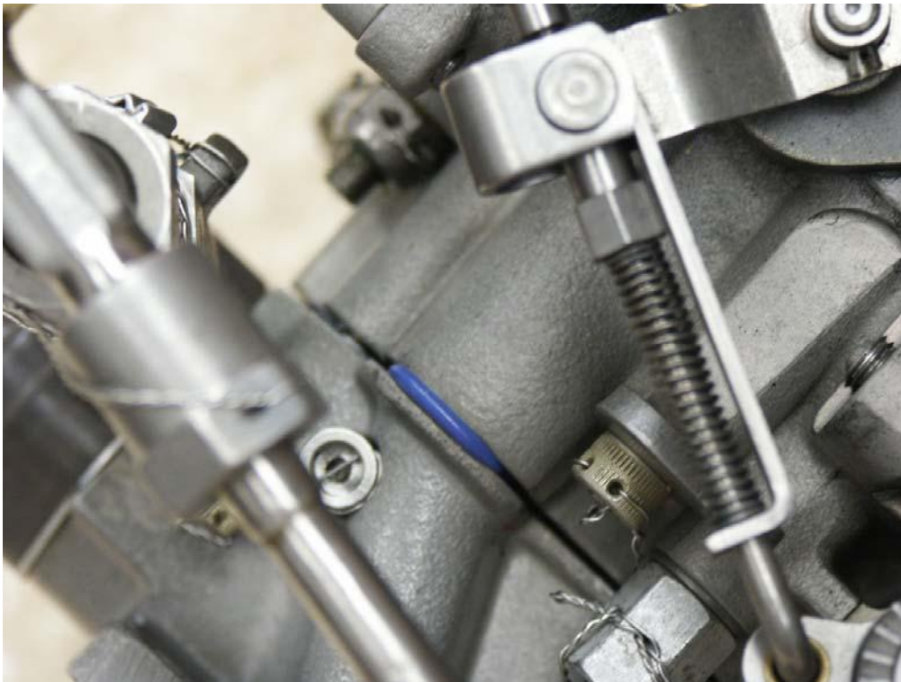
Figure 6 separation of bodies and extrusion of P0 o-ring
