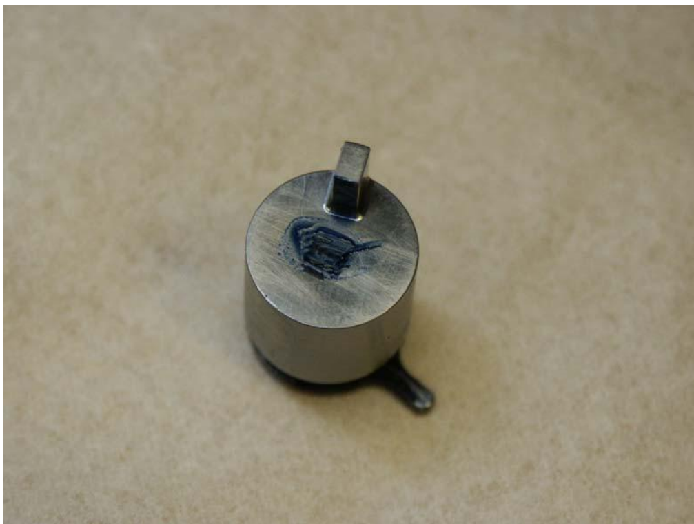
Figure 19 diluted blue grease on spool bearing assembly
