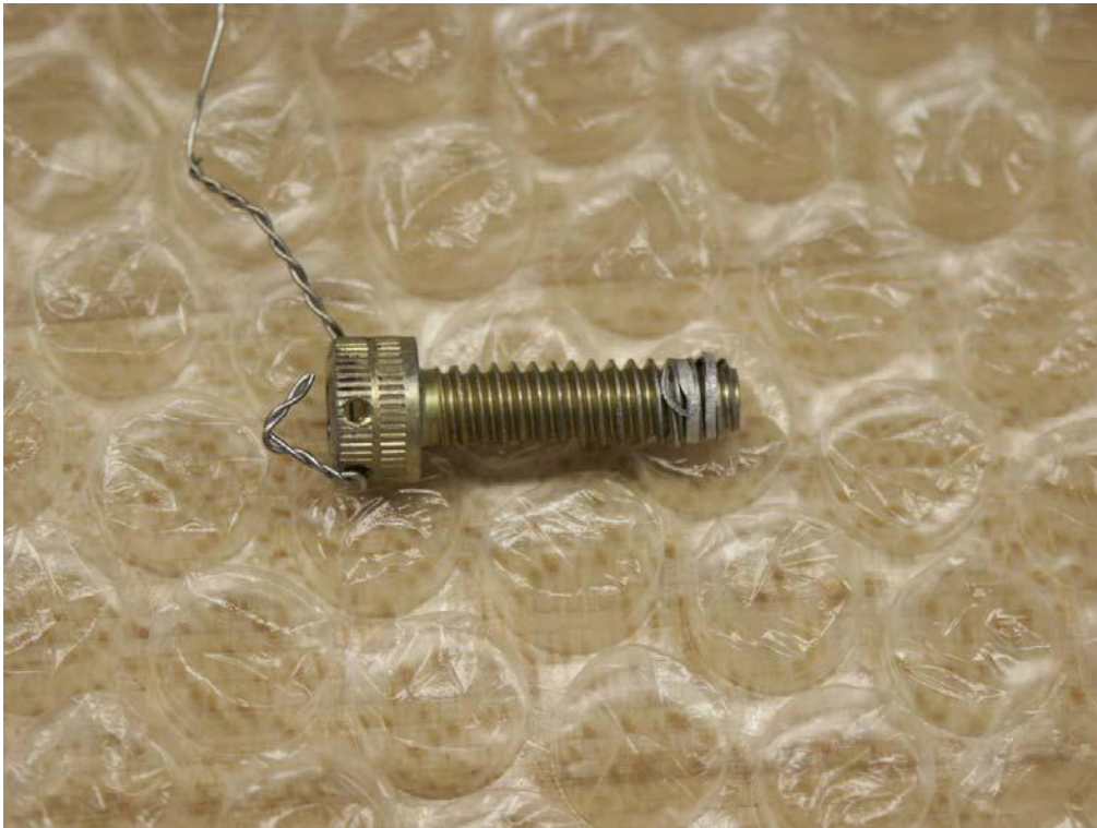
Figure 18 pulled drive body mounting screw
