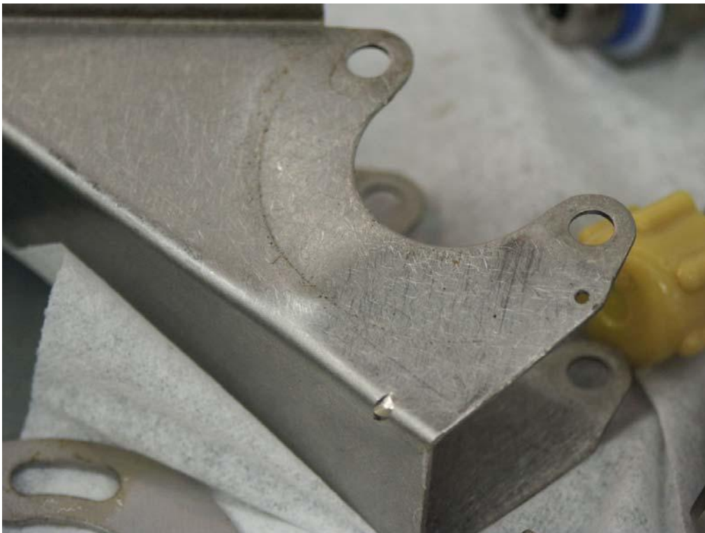
Figure 12 deformation of shield and sharp dent
