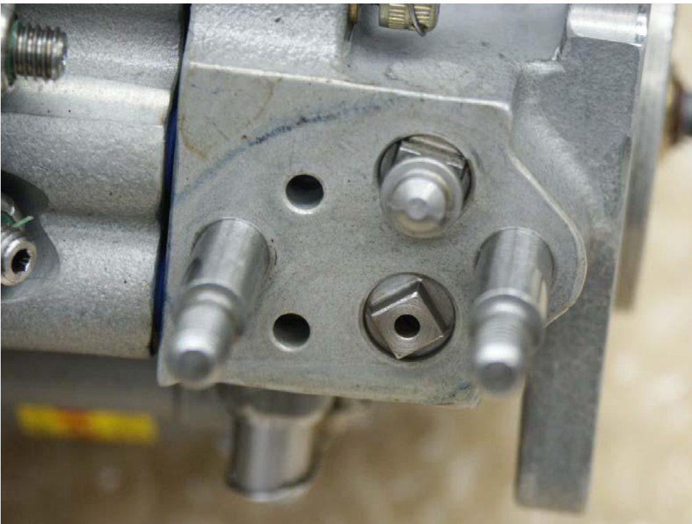
Figure 14 drive body adapter mating surface with ring of blue grease
