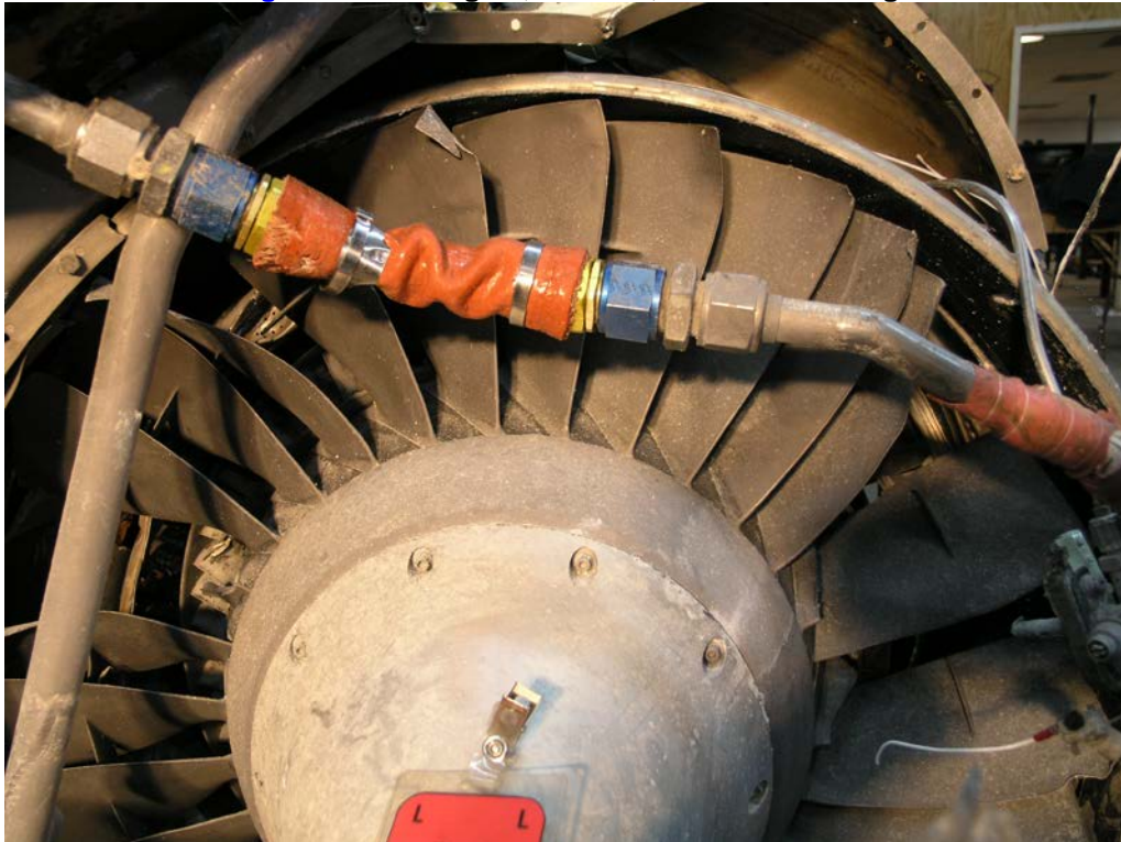
Figure 3. Left Engine, P-74717, Main Fan Damage
