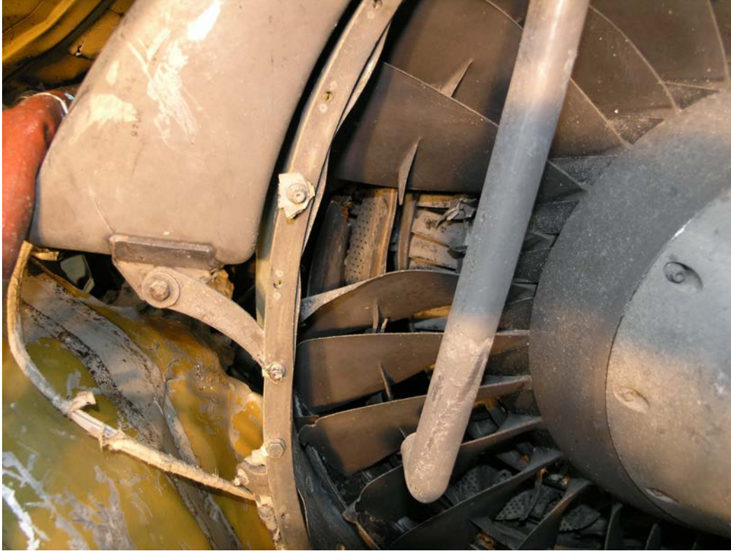
Figure 5. Left Engine, P-74717, Main Fan Damage
