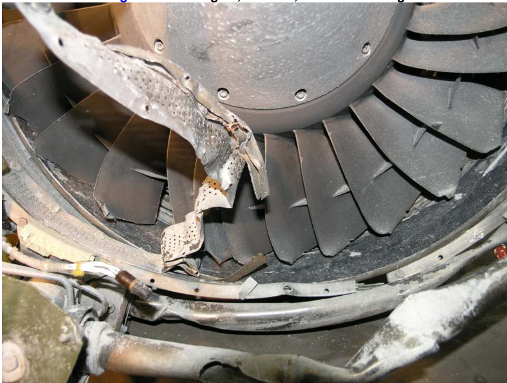
Figure 5. Left Engine, P-74717, Main Fan Damage
