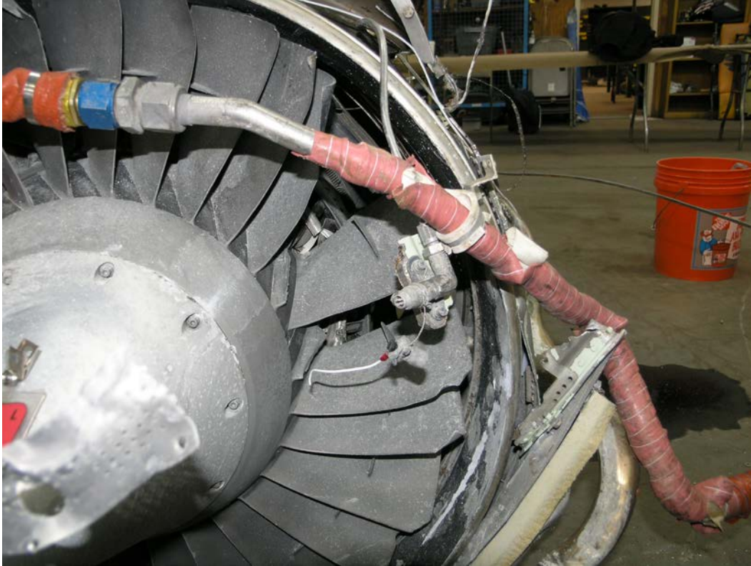
Figure 3. Left Engine, P-74717, Main Fan Damage
