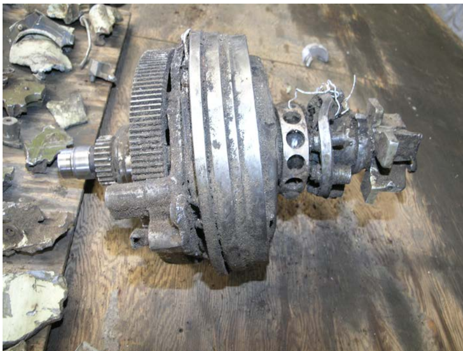
Figure 1. Bull Gear, Ring Gear, Engine Propeller Shaft, and Propeller Fork.
