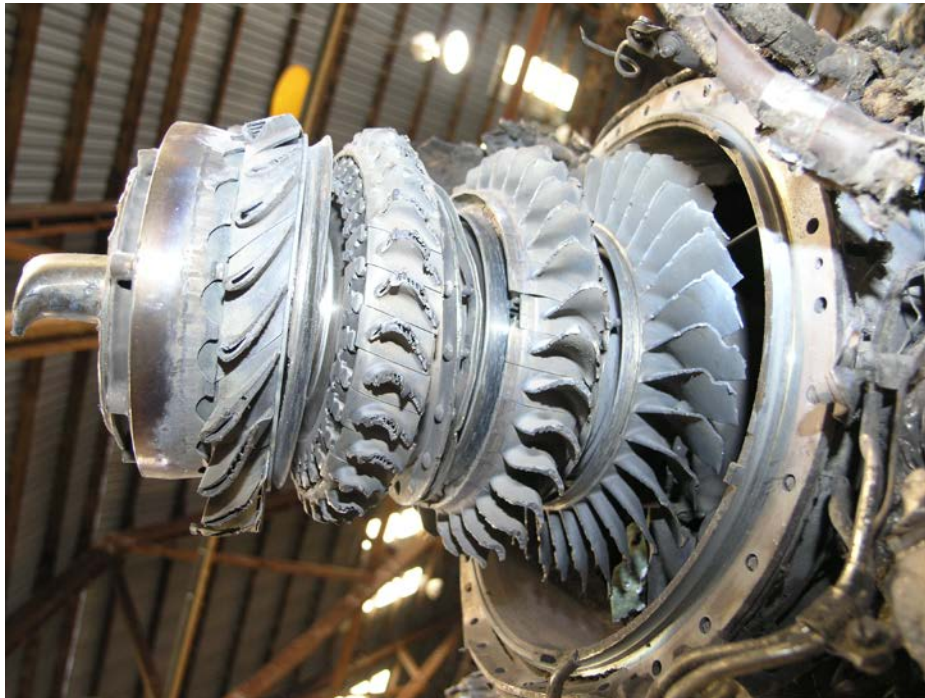
Figure 11. First-, Second-, and Third-Stage Turbine Rotors.
