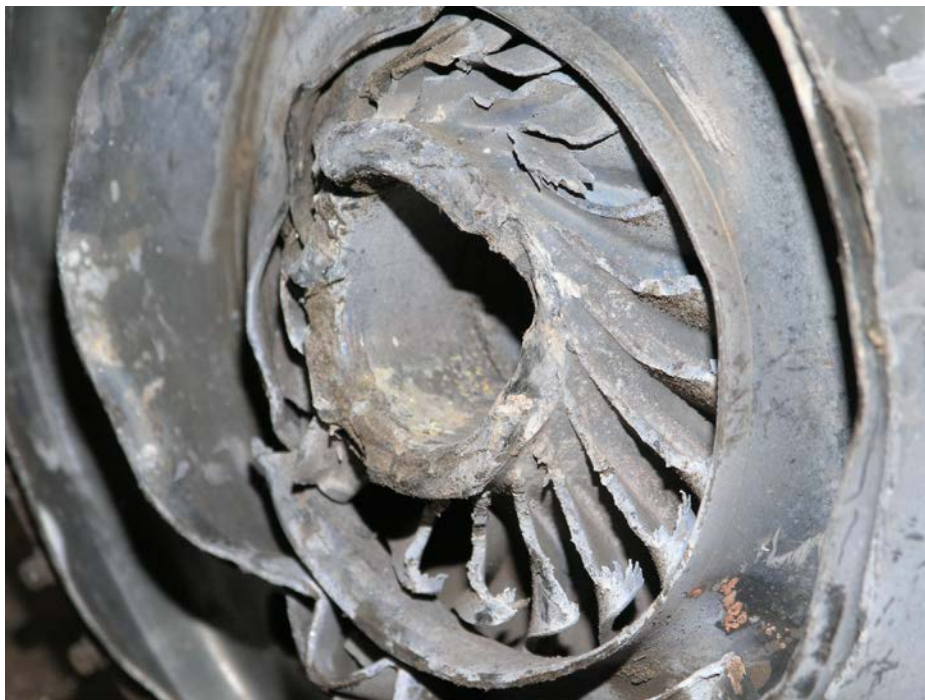
Figure 8. Second-Stage Compressor Impeller.
