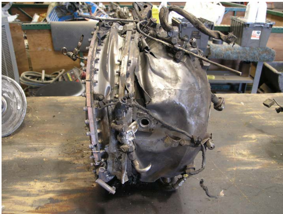
Figure 10. Second-Stage Compressor Housing and Plenum.
