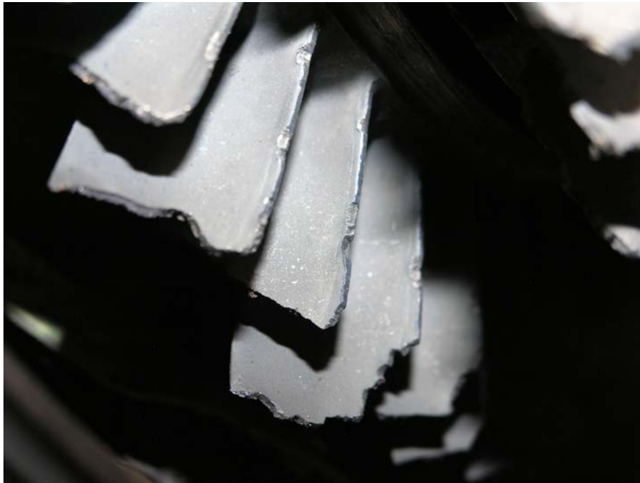
Figure 17. Third-Stage Turbine Rotor Blades.
