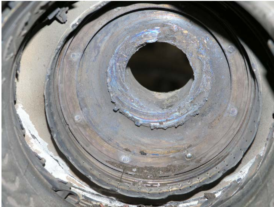
Figure 9. Second-Stage Compressor Impeller, Aft Looking Forward.
