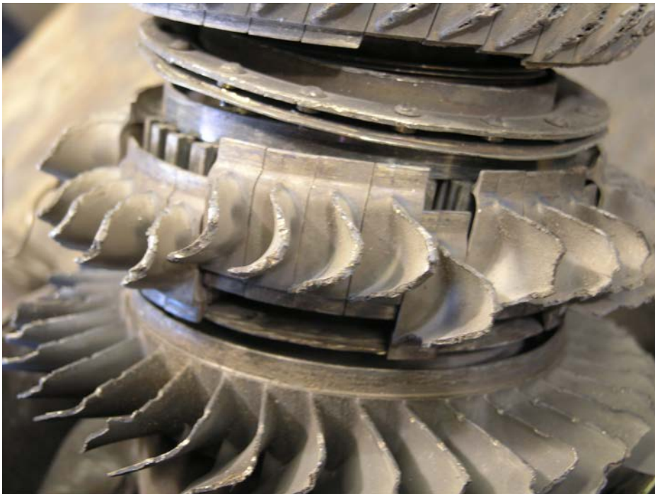
Figure 14. Second-Stage Turbine Rotor.
