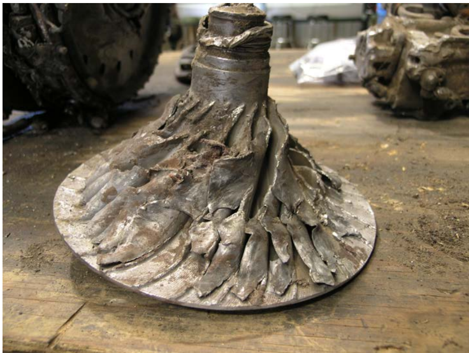
Figure 6. First-Stage Compressor Impeller.
