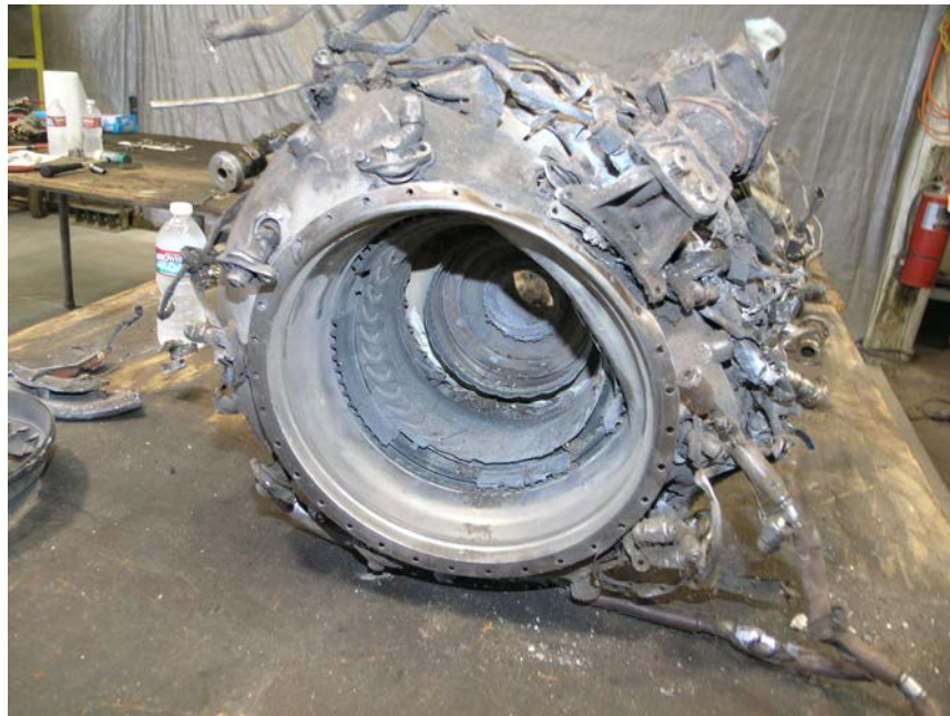
Figure 3. Second-Stage Compressor Housing and Impeller, Plenum, Combustion Liner, First- and Second-Stage Turbine Stator Vane Outer Supports.
