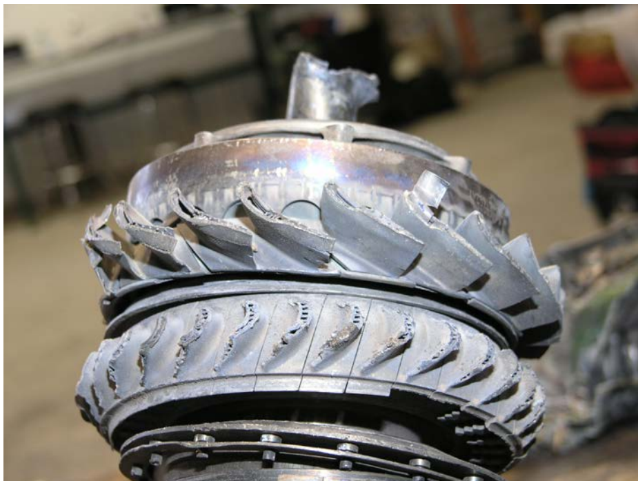
Figure 12. First-Stage Turbine Stator Vanes and Rotor Blades.
