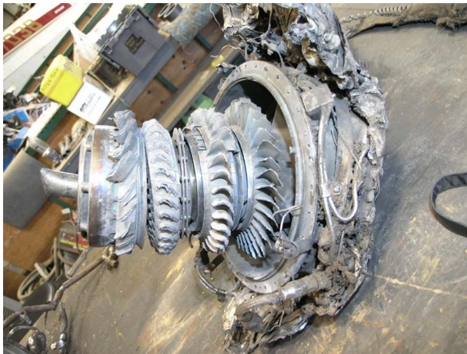
Figure 4. First-, Second-, Third-Stage Turbine Rotors and Turbine Bearing Support Housing.
