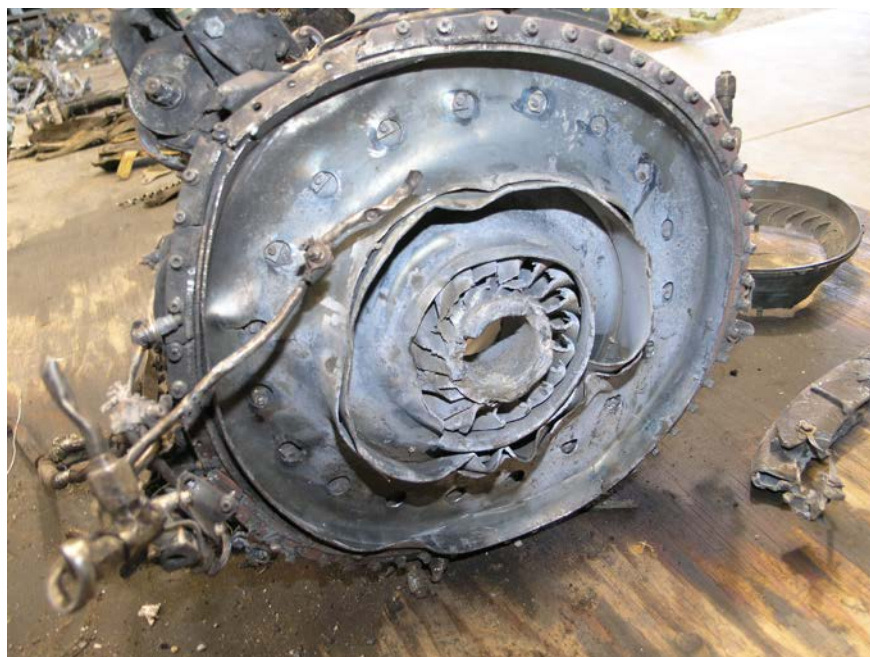
Figure 2. Second-Stage Compressor Housing and Impeller, Plenum, Combustion Liner, First- and Second-Stage Turbine Stator Vane Outer Supports.
