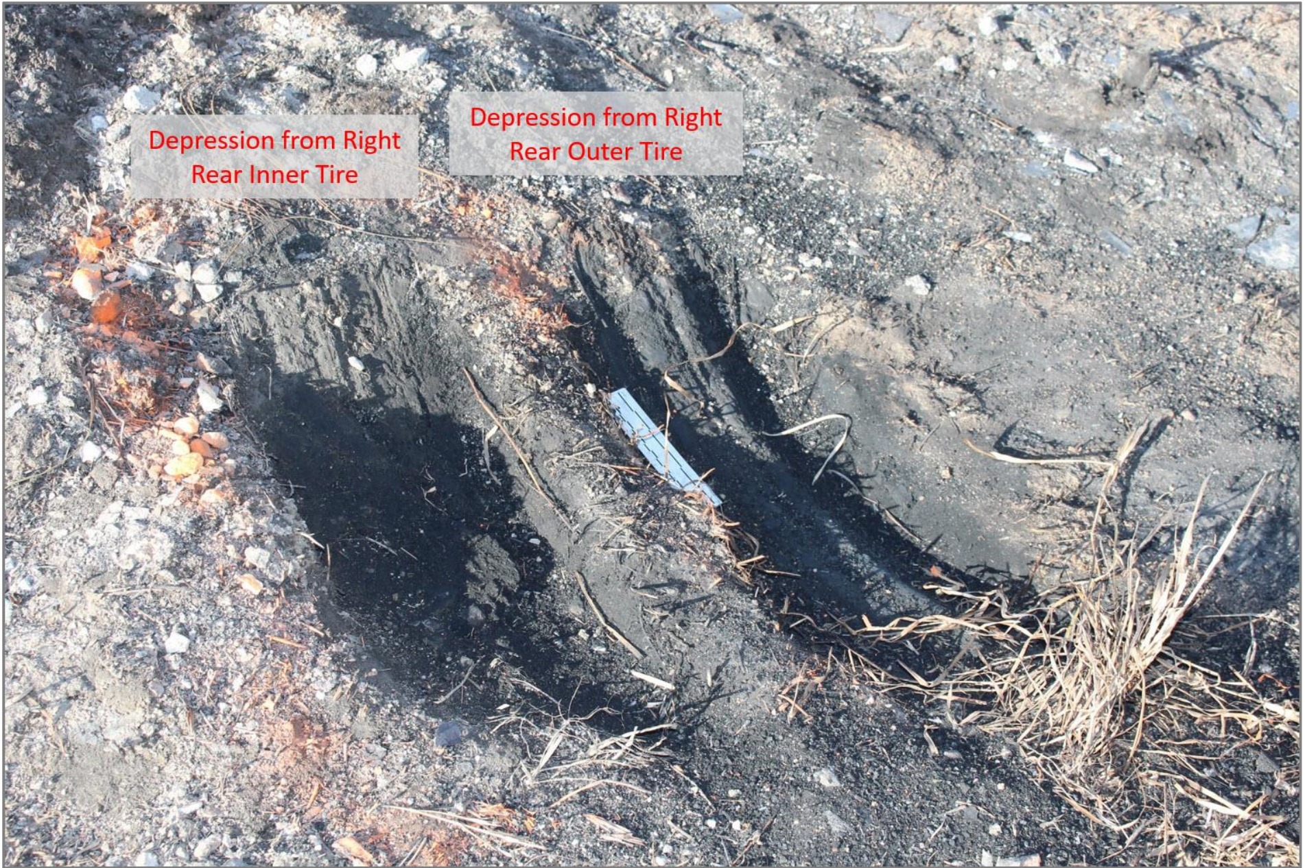
Highway Photograph 4 – Right Rear Tire Depressions Near the Bottom of Ditch Foreslope
