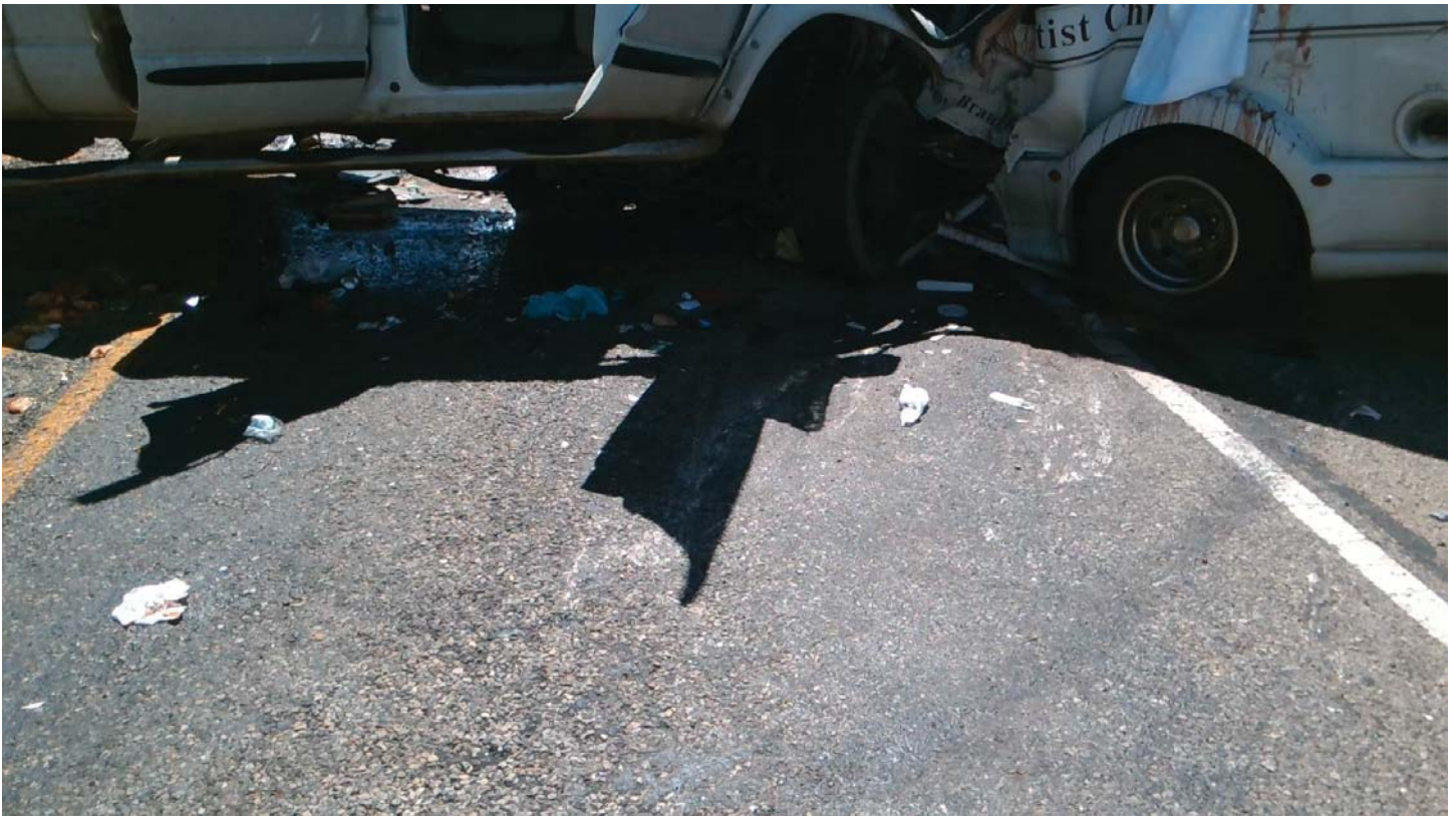
Highway Photo 10 – Closer view of scrapes on the pavement and tire friction marks leading away from the impact area.
