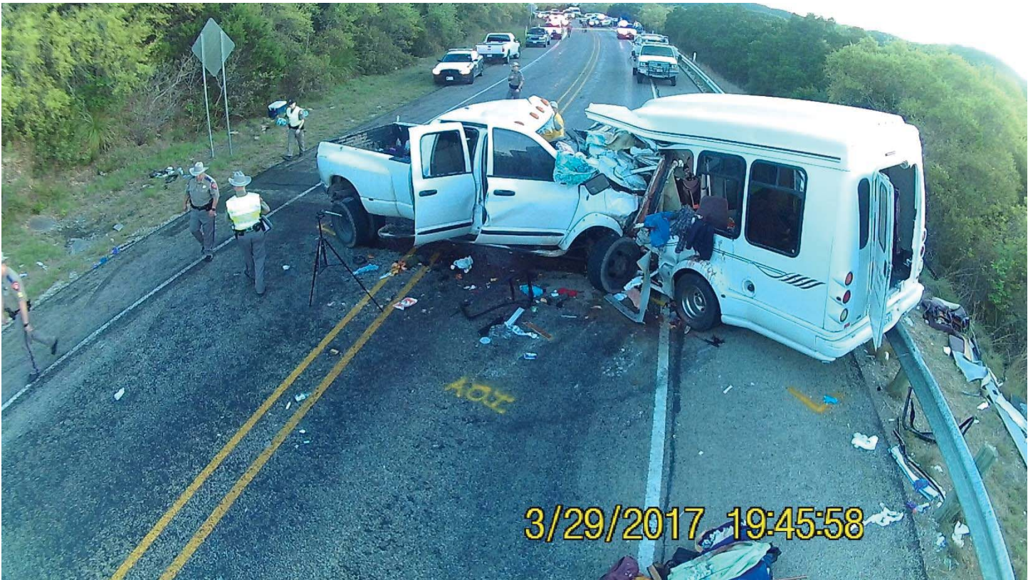
Highway Photo 1 – Southbound view on US 83, showing the final positions of both accident vehicles. Note the scrapes and tire friction marks leading away from the impact area. Highway photos 1-11 are provided courtesy of the Texas Highway Patrol
