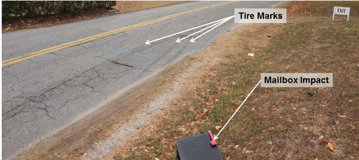
Highway Photograph 4 – Mailbox impact located in the foreground of the graphic and the tire marks in the southbound lane left by the school bus after the wheels returned to the pavement
