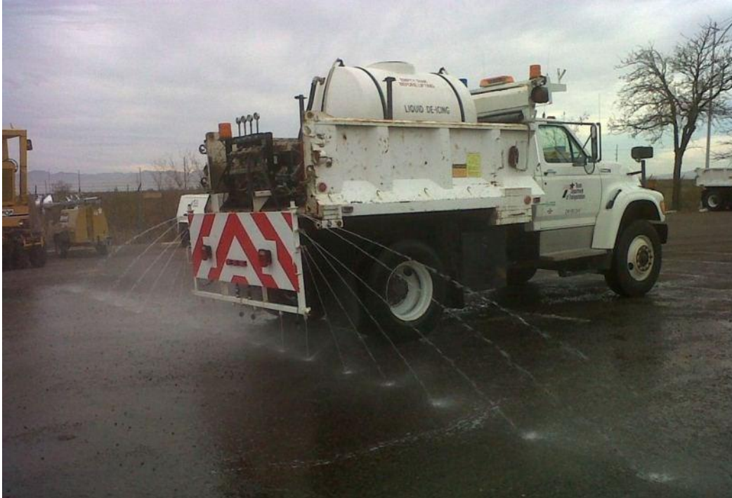
Figure 2 Application of liquid chemical by stream nozzles.
