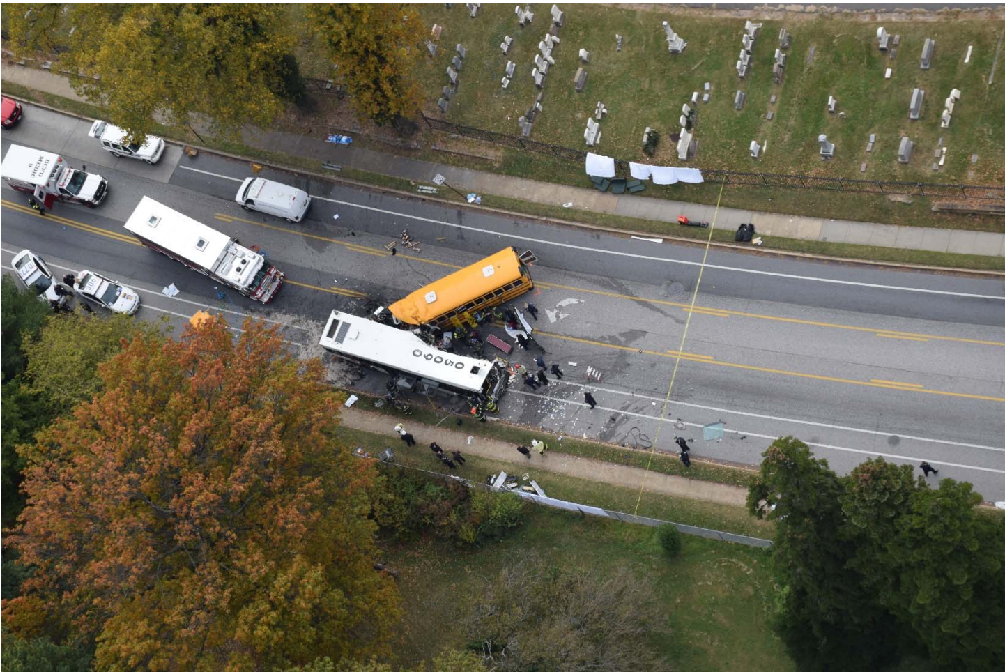
Highway Photo 13 – Aerial view of the school bus-transit bus impact area depicted by fluid spatter and debris forward of the transit bus.
