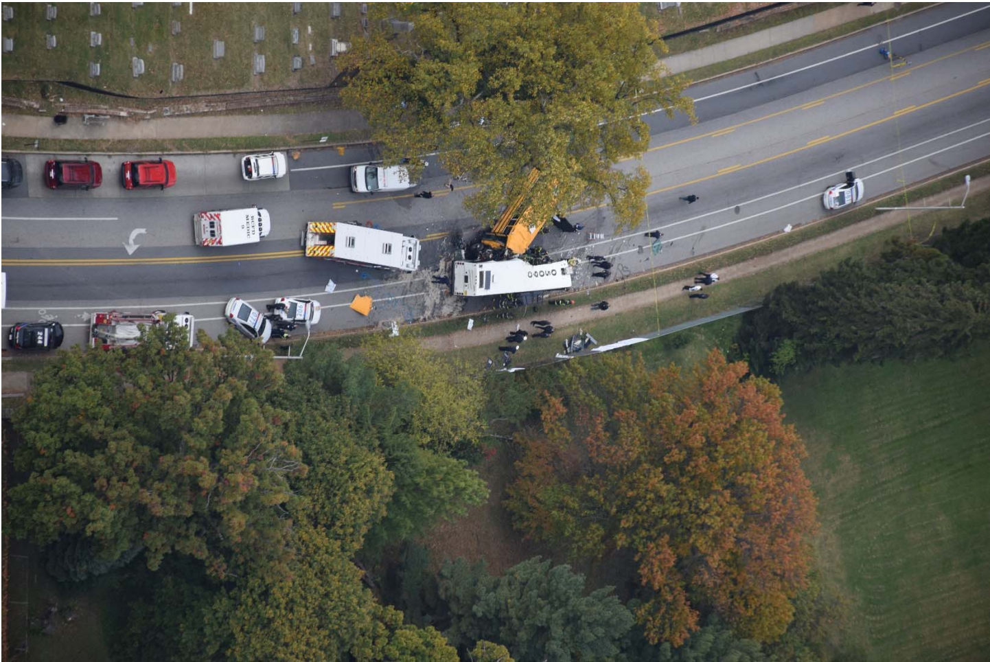
Highway Photo 9 – Additional aerial view showing the depth of penetration by the school bus into the left side of the transit bus
