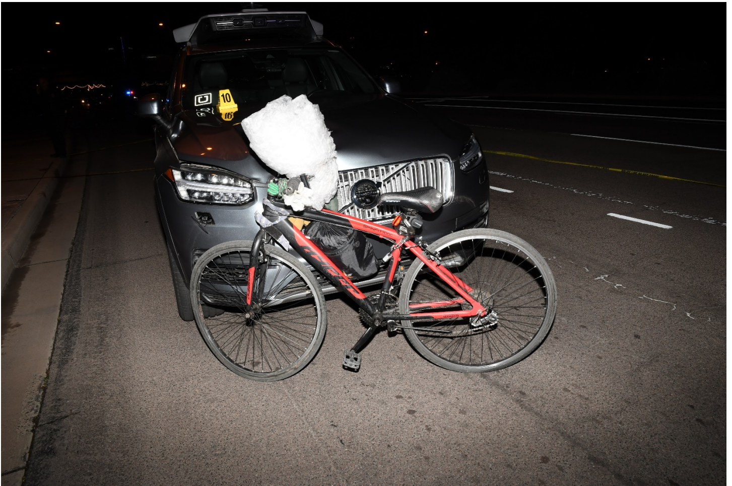
Photo 20 – View showing bicycle matched up to the damaged areas on the Uber/Volvo.
