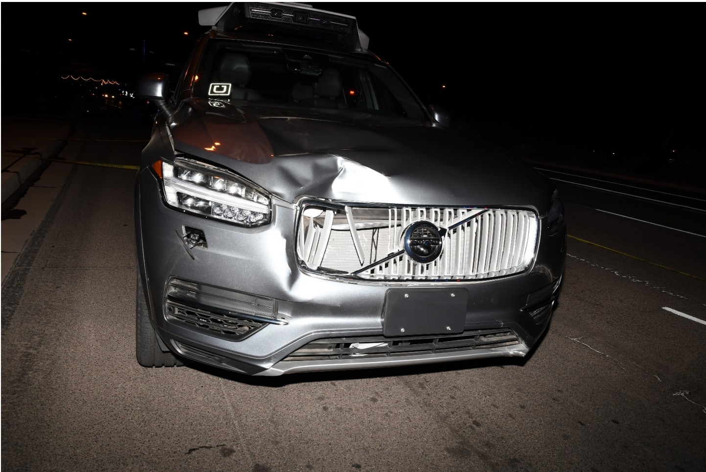
Photo 18 – View of the damage from the impact on the right front of the Uber/Volvo.
