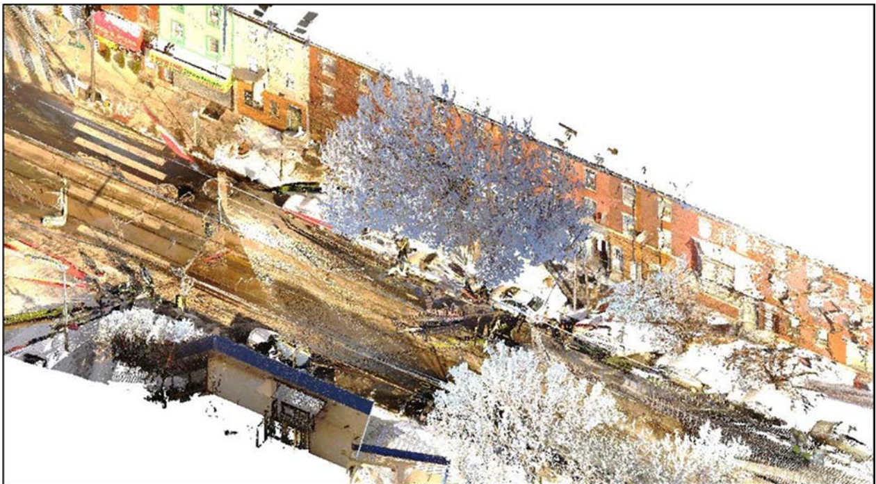
Figure 3: Screen capture depicting a portion of the 3D point cloud rendered from the scans. Movement of vehicles and person through the scene created color anomalies and stray objects.
