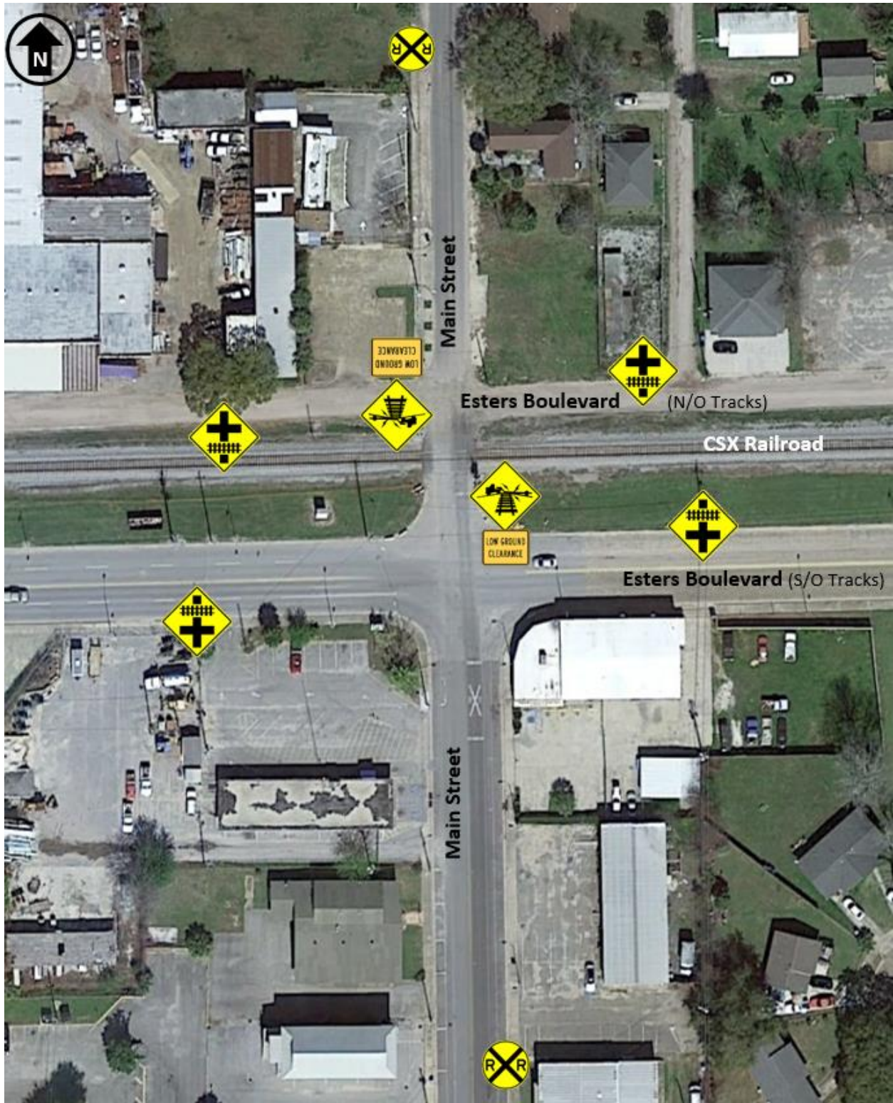
Figure 4: Crossing Related Advanced Warning Signs Near the Main Street Grade Crossing (modified from: Google Earth)
