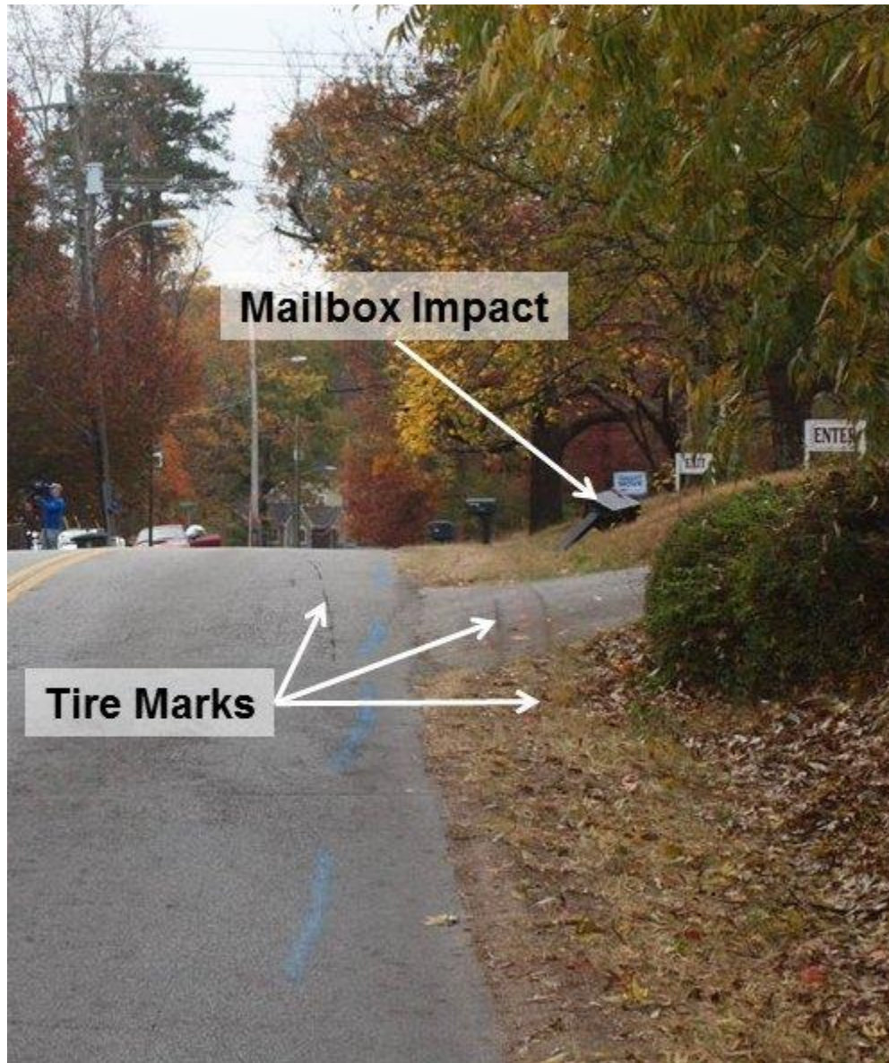
Highway Photograph 1 - Tire marks left by the school bus on the grass and right side of Talley Road in the southbound direction of travel and the mailbox impact located in the background of the graphic
