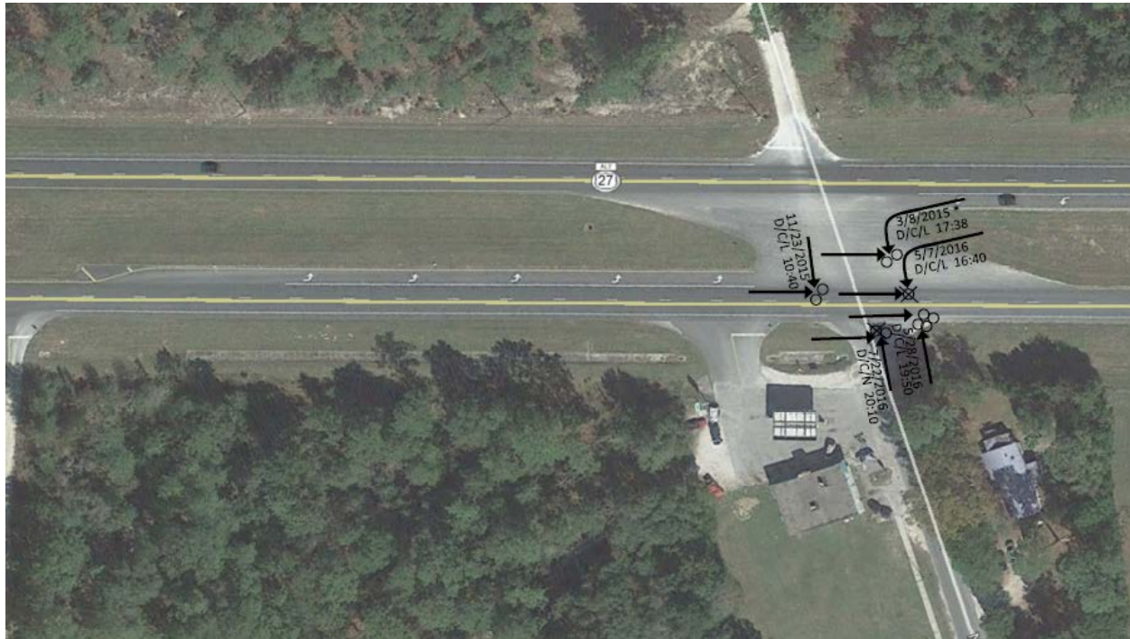
Figure 2. Depiction of vehicle movements for five recent crashes occurring at the intersection location. Image and graphic overlays courtesy of FDOT.
