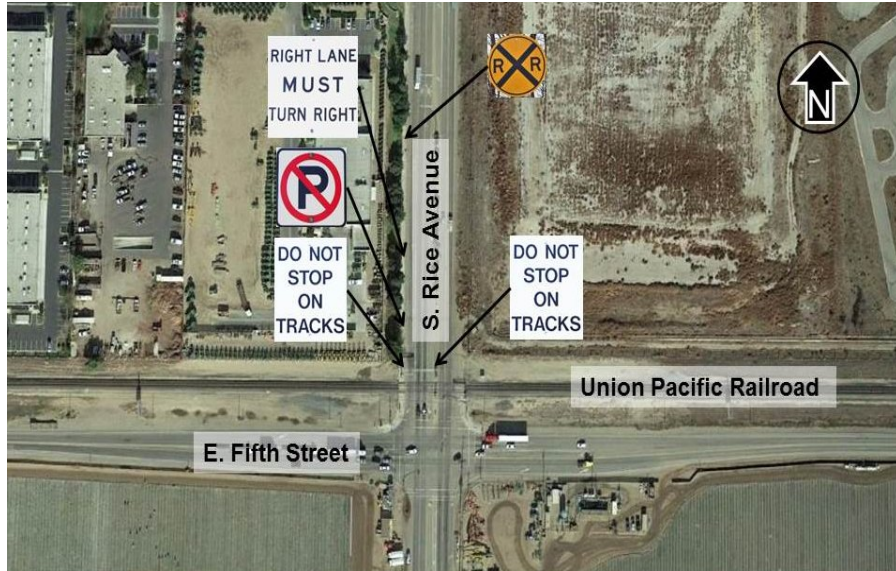
Figure 4 – Signage in the vicinity of the grade crossing on the southbound approach to the grade crossing.
